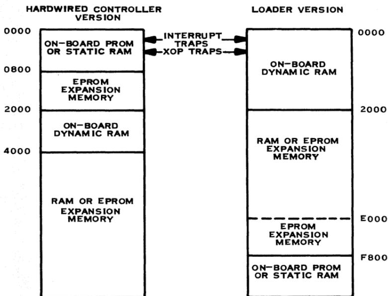
**NOTE:** FOR COMPATIBILITY WITH STANDARD 990 SOFTWARE AND OTHER 990 COMPUTERS, THE LOADER VERSION MUST BE USED WITH PROM CONFINED TO FC00 UP (512 WORDS) AND ADDRESSES F800-FC00 (TILINE PERIPHERAL CONTROL SPACE) NOT USED IN 990/4. ADDRESSES 0000-004F MUST BE RESERVED FOR INTERRUPT TRAPS, XOP TRAPS, AND STANDARD WORKSPACE.
