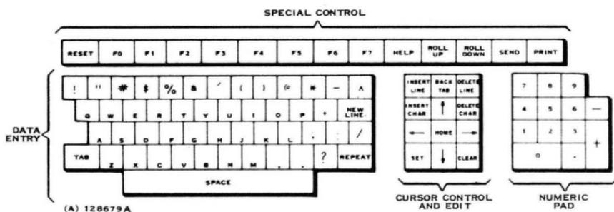
Figure 5-3. Model 913 Video Display Terminal Keyboard
