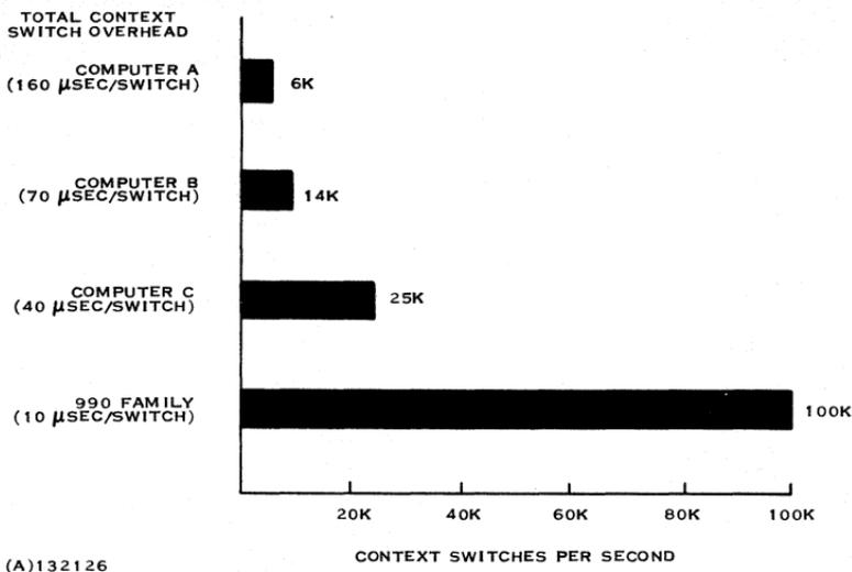
Figure 3-3. Comparison of Context Switching Efficiency
