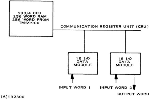
Figure 6-2. Hardwired Controller Block Diagram
