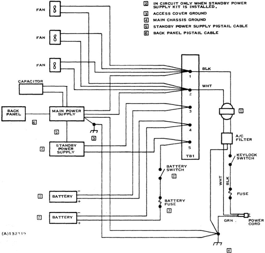
Figure G-1. Chassis Wiring for 6-Slot or 13-Slot Chassis
