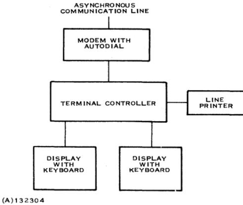
Figure 6-7. Functional Block Diagram for Intelligent Terminal
