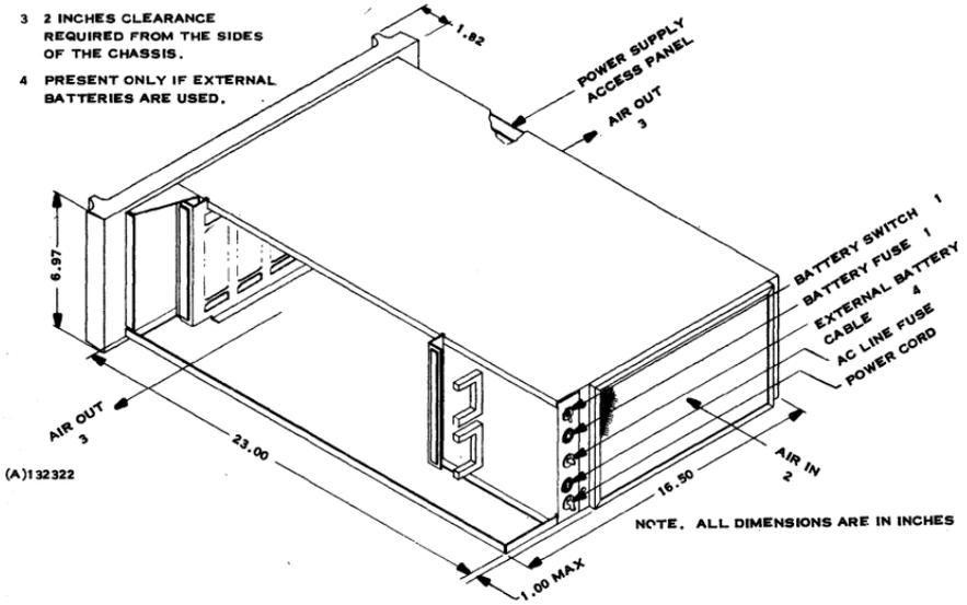
Figure G-3. 6-Slot Chassis Physical Configuration
