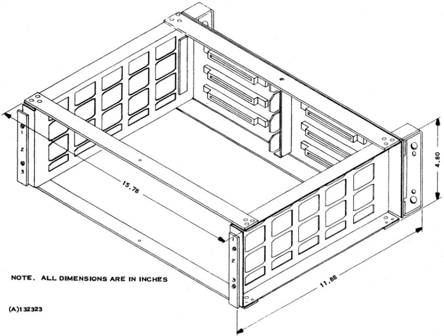
Figure G-4. OEM Chassis Physical Configuration
