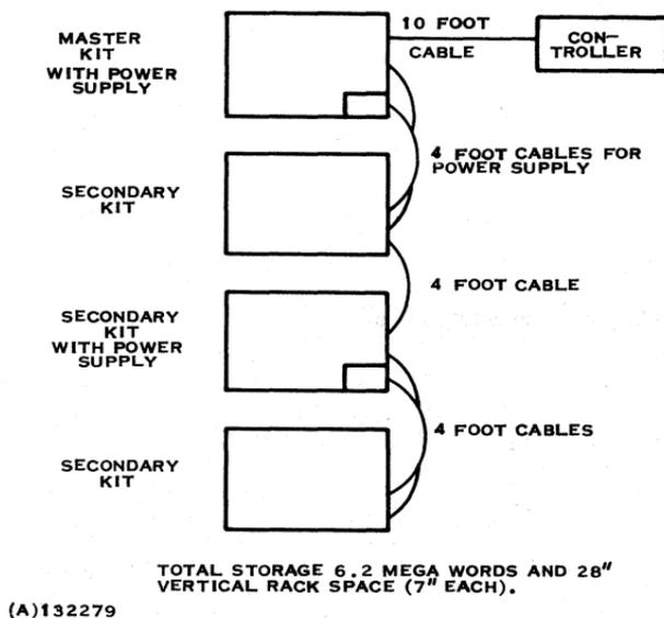
Figure 5-11. Disc System Configuration
