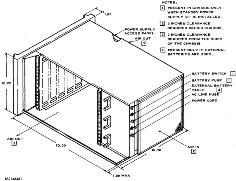
Figure G-2. 13-Slot Chassis Physical Configuration.
