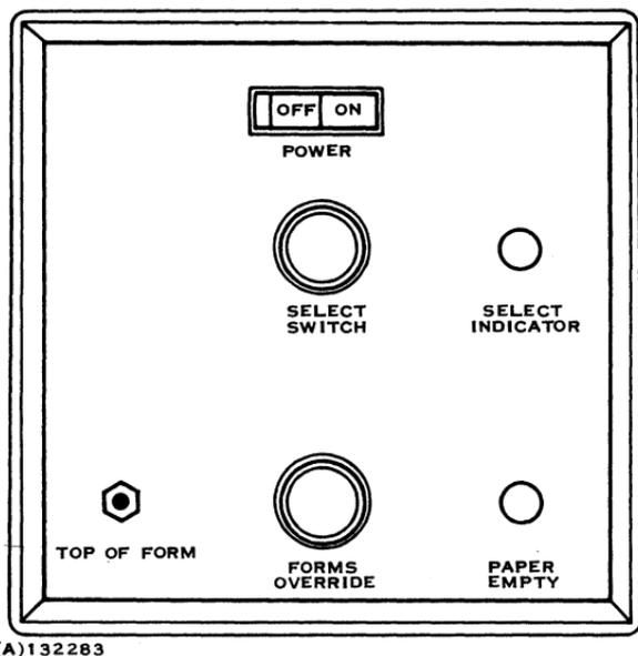
Figure 5-15. Model 306 Line Printer Operator Control Panel
