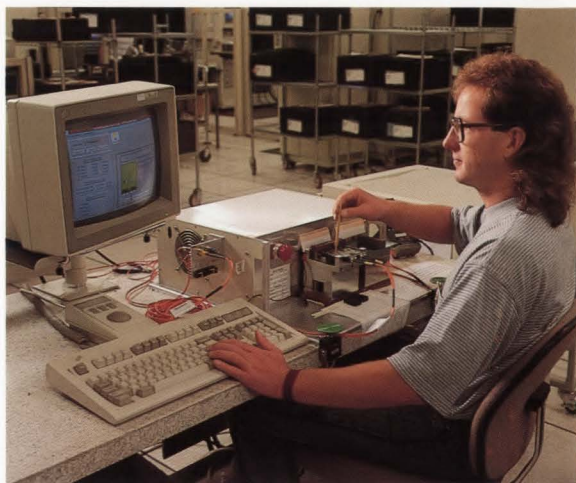
Figure 128. Multipurpose Functional Tester Setup
