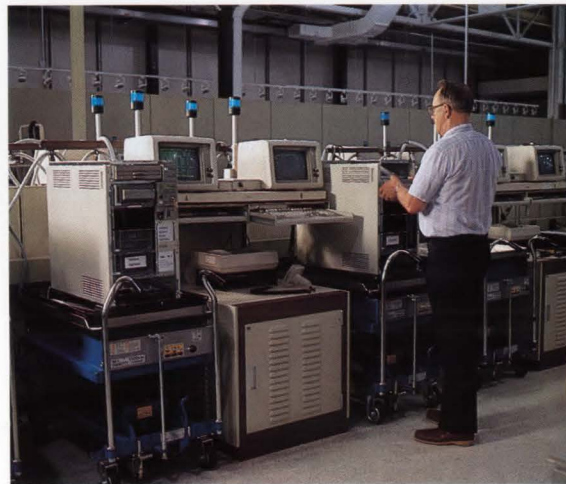
Figure 122. Test and Software Preload Station
