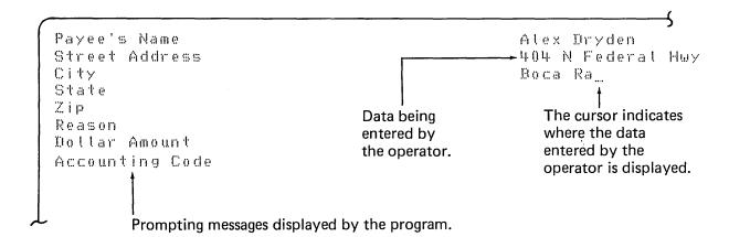
When used for input and output, the display screen is treated as a record I/O file, similar to a record I/O file on tape or diskette. You must open the display screen for input/output using device 002, for example:
