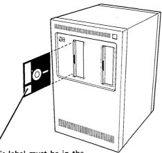
This label must be in the lower corner as the diskette is inserted in the diskette drive. The diskette drive door must be closed and latched after the diskette is inserted.
