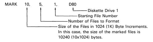
Unlike tape files, diskette files are not always formatted sequentially on the diskette. For example, file 2 might be on cylinder 3, file 3 on cylinder 9, and file 4 on cylinder 7. You can control the location of a file on the diskette only by using a totally unmarked diskette and issuing MARK commands in the same order as the files are to be formatted on the diskette.
