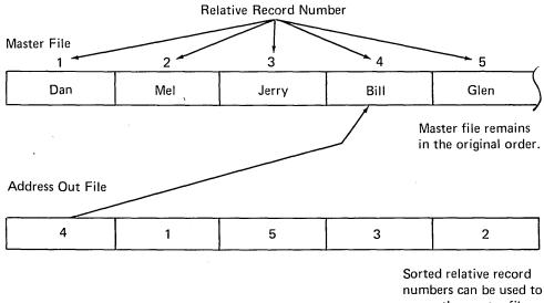
numbers can be used to access the master file in ascending order. The following statements might be used in a program to access a file in order using the record numbers in the address out file:
