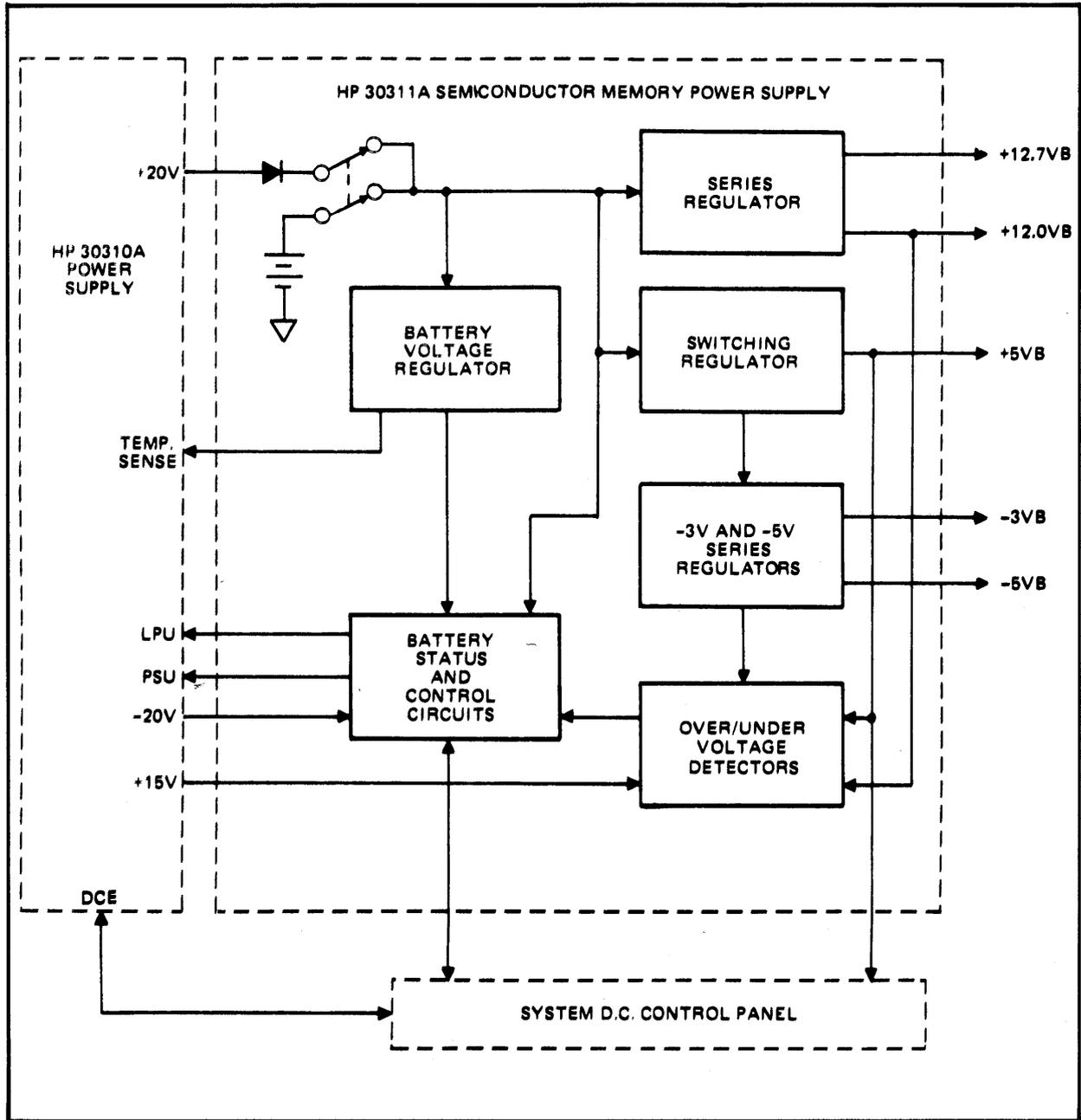
Figure 9-3. HP 30311A Power Supply Block Diagram
