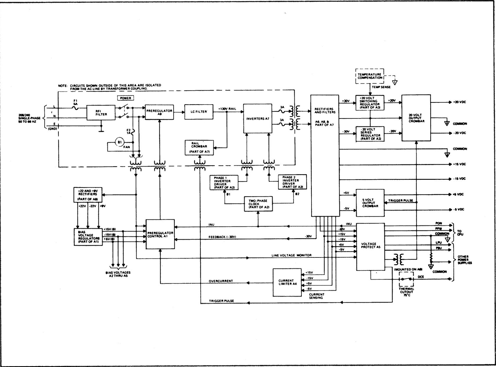
Figure 9-2. HP 30310A Power Supply Block Diagram
