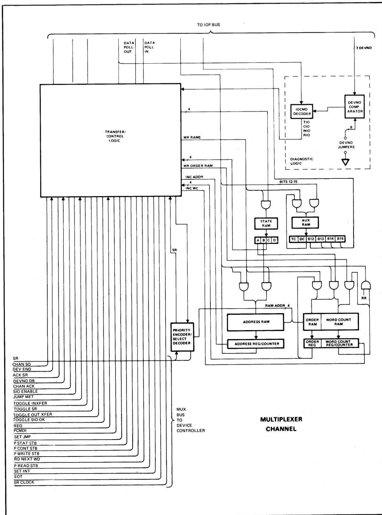
Figure 7-16. Multiplexer Channel Simplified Logic Diagram
