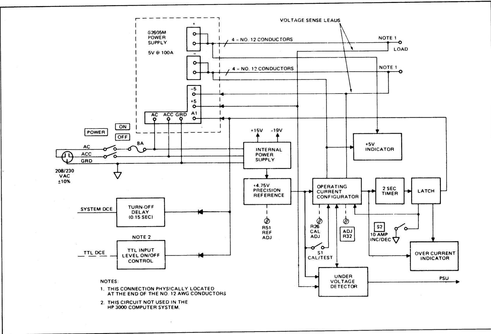
Figure 9-5. HP 30312A Power Supply Block Diagram
