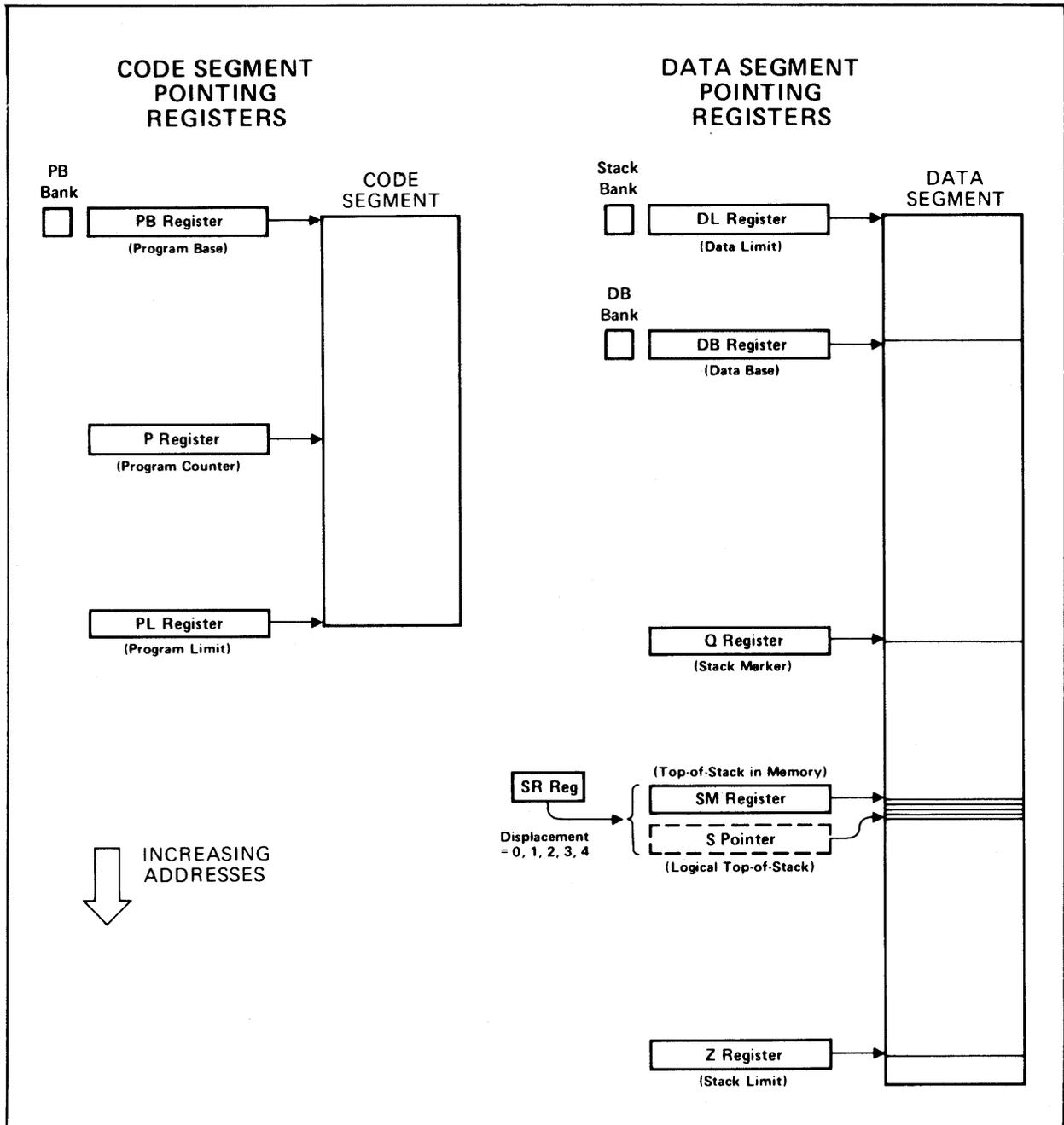
Figure 2-4. CPU Segment Pointer Registers
