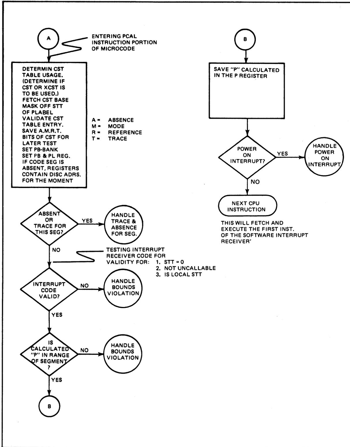
Figure 8-7. Interrupt Handler Flowchart (Sheet 2 of 2)
