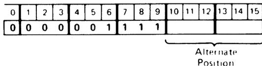
The Condition Code is set to pattern C as a result of the integer comparison of the second word of the stack with the TOS. Both words are deleted.
