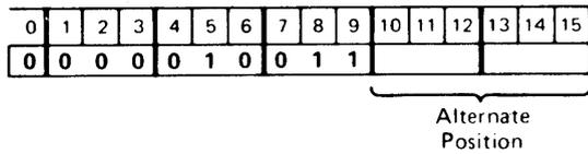
The integer in the second word of the stack is divided by the integer on the TOS. The two words are then deleted. The second word is replaced by the quotient, and the top word is replaced by the remainder.
