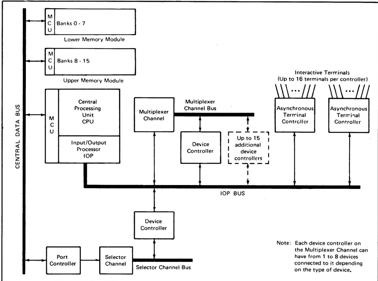
Figure 2-1. HP 3000 Series III Computer System Hardware Organization
