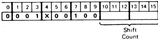
The TOS is shifted left  $n$  bits circularly. The value of  $n$  (modulo 64) is the number specified in the argument field plus, if  $X$  is specified, the content of the Index Register.
