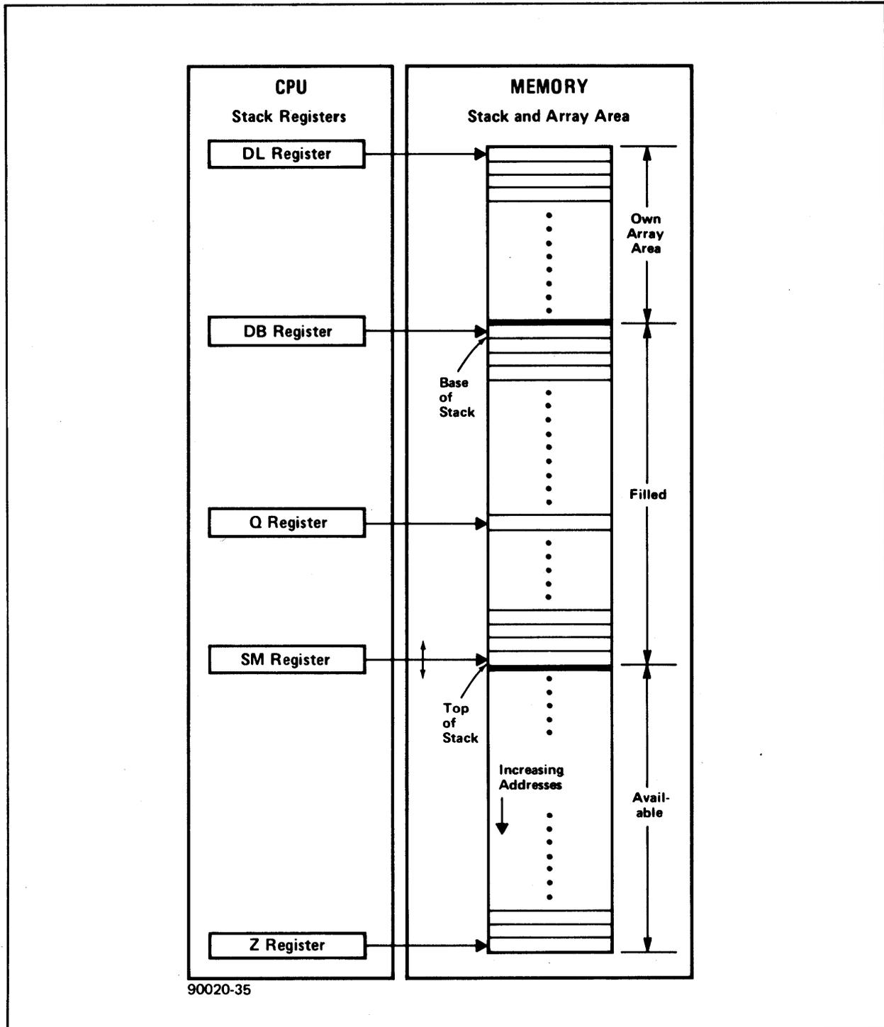
Figure 2-9. CPU Registers and Stack Basic Operations
