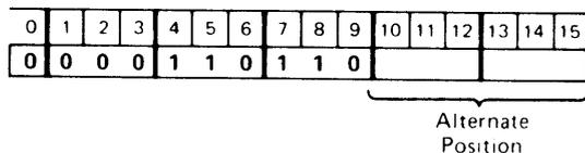
The top two words of the stack are combined by a logical exclusive-OR. The two words are deleted and the result is pushed onto the stack.
