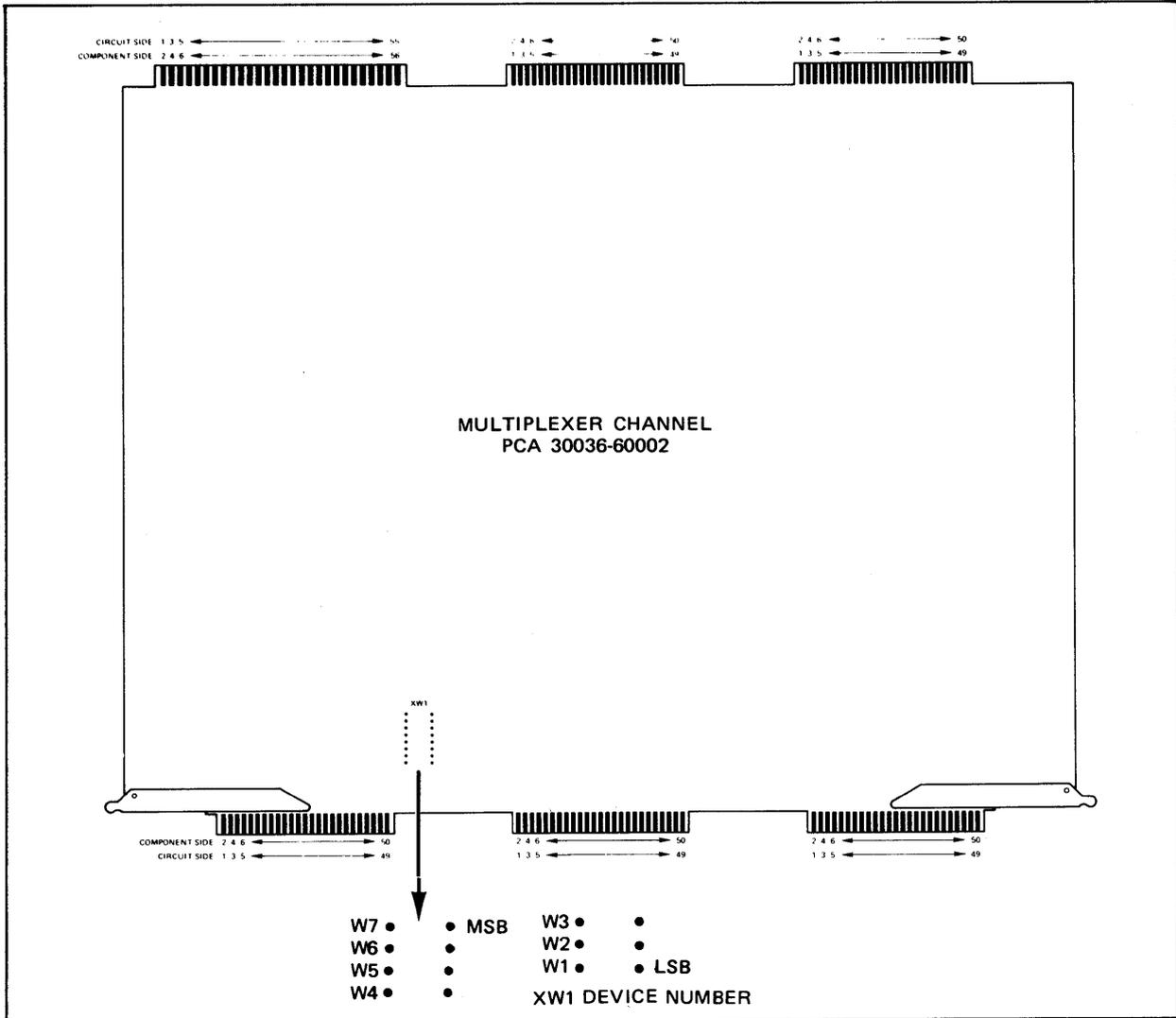
Figure 7-21. Multiplexer Channel PCA Jumper Locations
