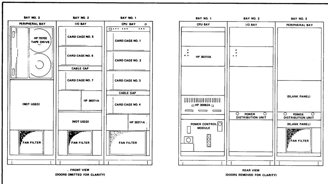
Figure 1-3. HP 32421A Series III Computer System, 3-Bay Model
