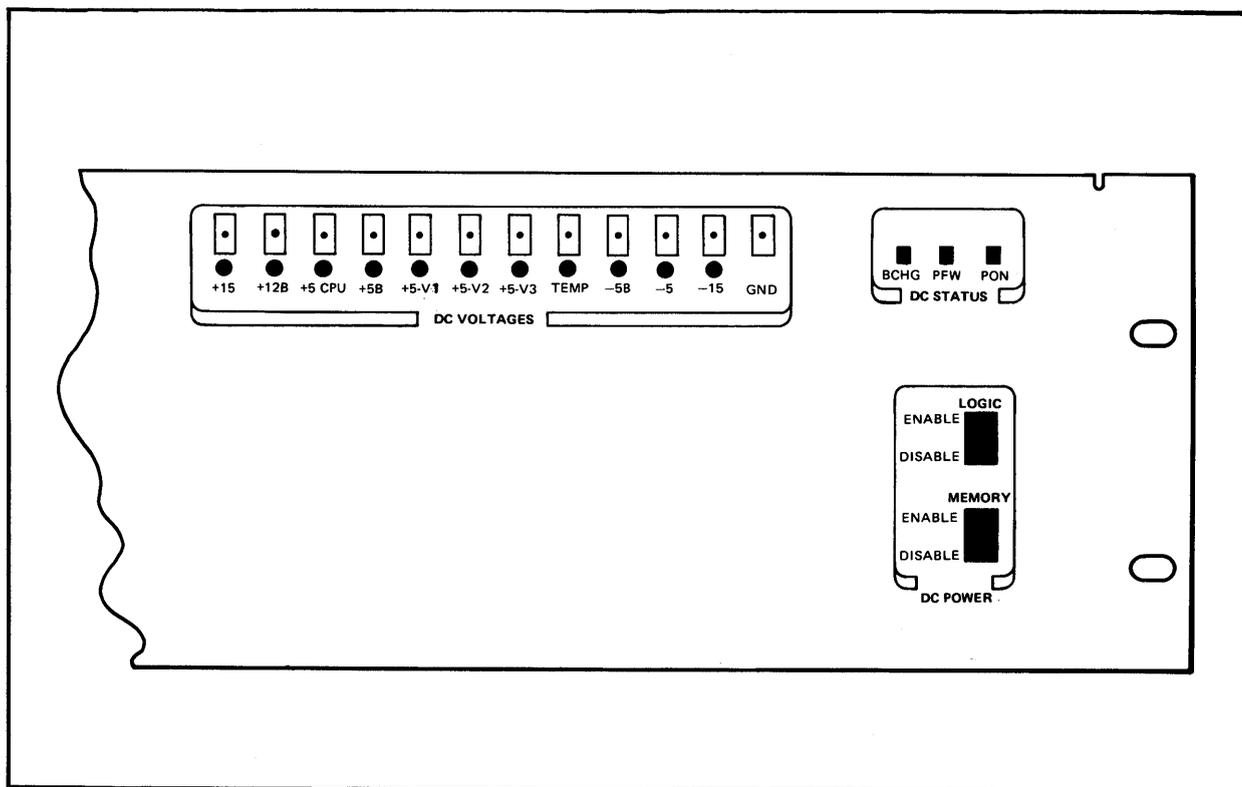
Figure 10-1. Power Supply Control and Display Assembly
