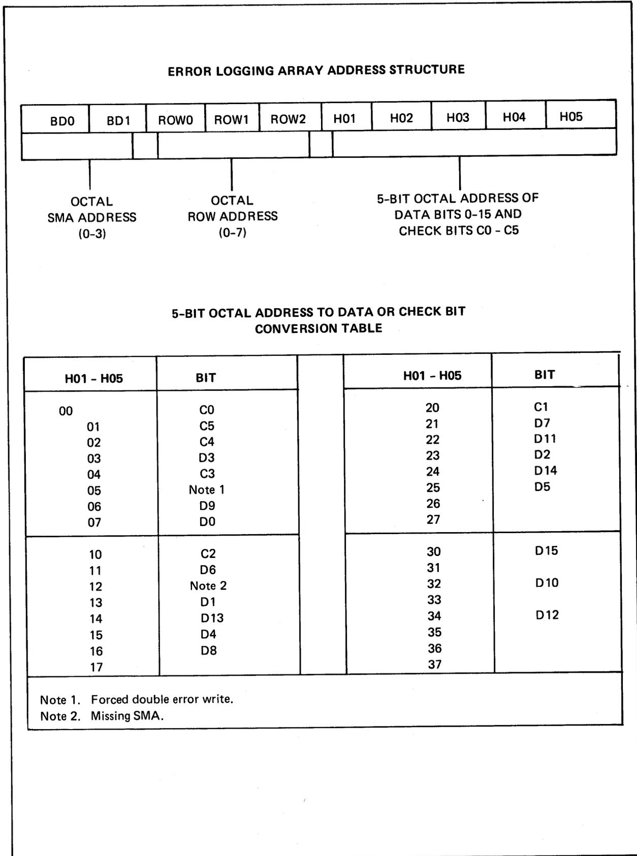
Figure 6-7. Decode of H01 through H05
