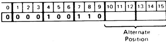
The double word in the top two words of the stack is duplicated by pushing a copy of it onto the stack.
