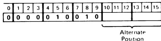
The top two words of the stack are multiplied in integer form. The two words are deleted and the least significant word of the double length product is pushed onto the stack. If the high order 17 bits of the double length product (including the sign bit of the second word) are not all zeros or all ones, Overflow is set.
