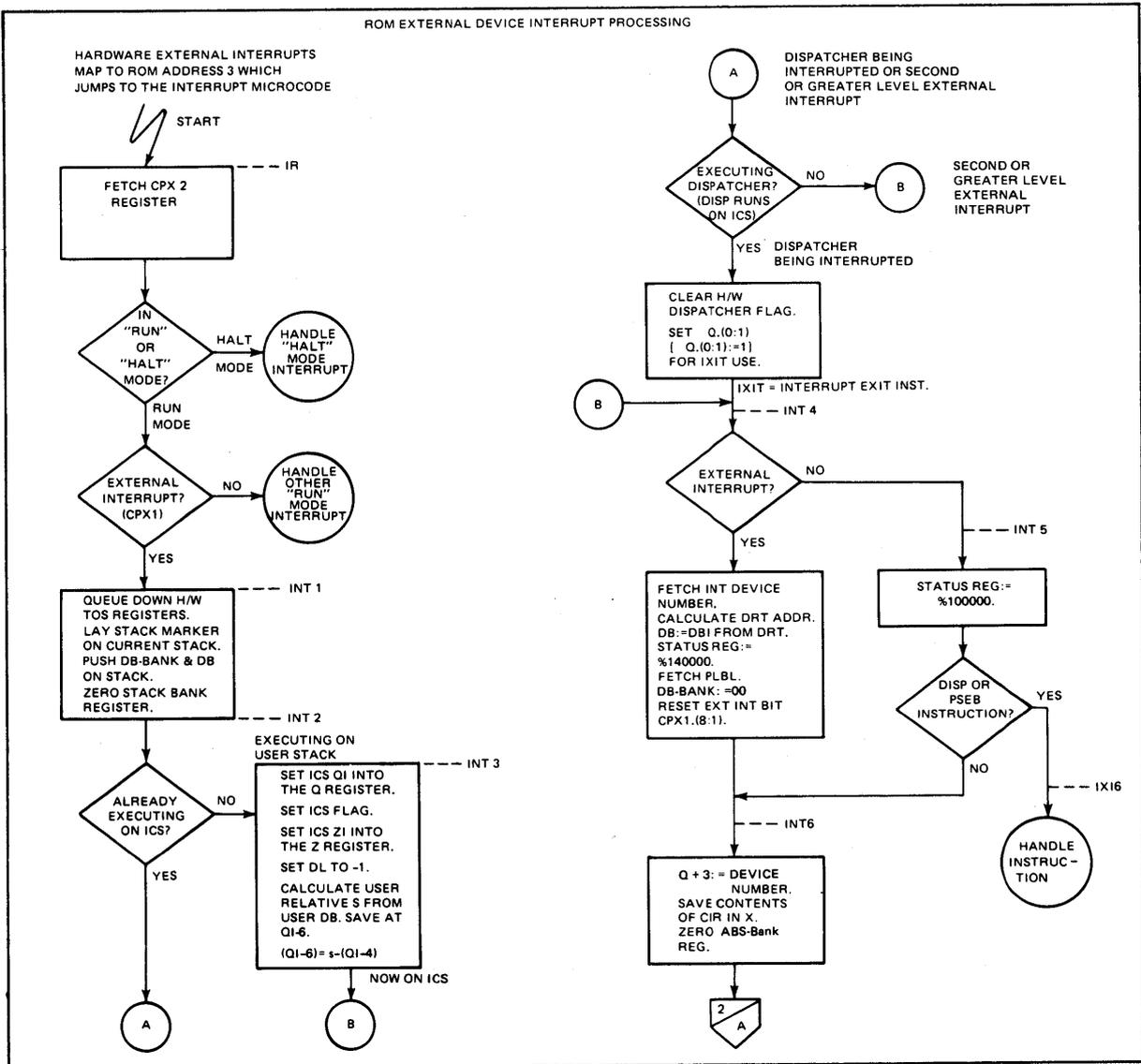
Figure 8-7. Interrupt Handler Flowchart (Sheet 1 of 2)
