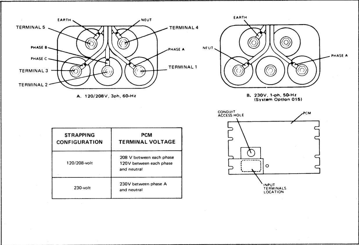
Figure 11-3. PCU/PCM Line Filter Connections
