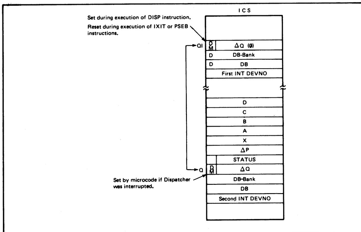
Figure 8-4. Second Level Interrupt or Dispatcher Interrupted
