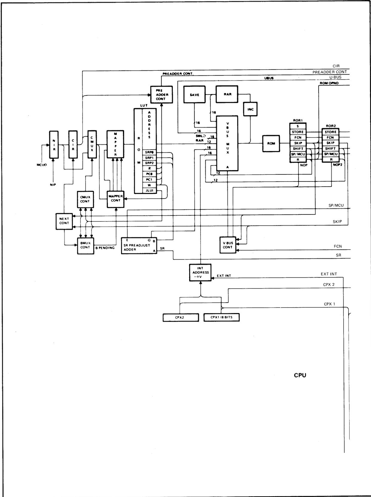
Figure 2-20. CPU Simplified Logic Diagram (Sheet 1 of 2)
