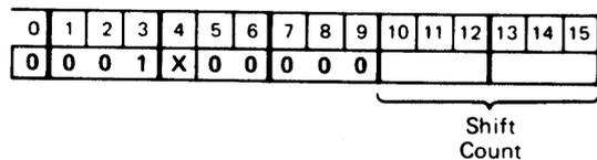
The TOS is shifted left  $n$  bits, preserving the sign bit. The value of  $n$  (modulo 64) is the number specified in the argument field plus, if  $X$  is specified (bit 4), the content of the Index Register.
