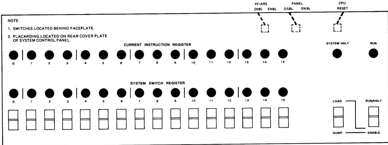
Figure 3-1. System Control Panel
