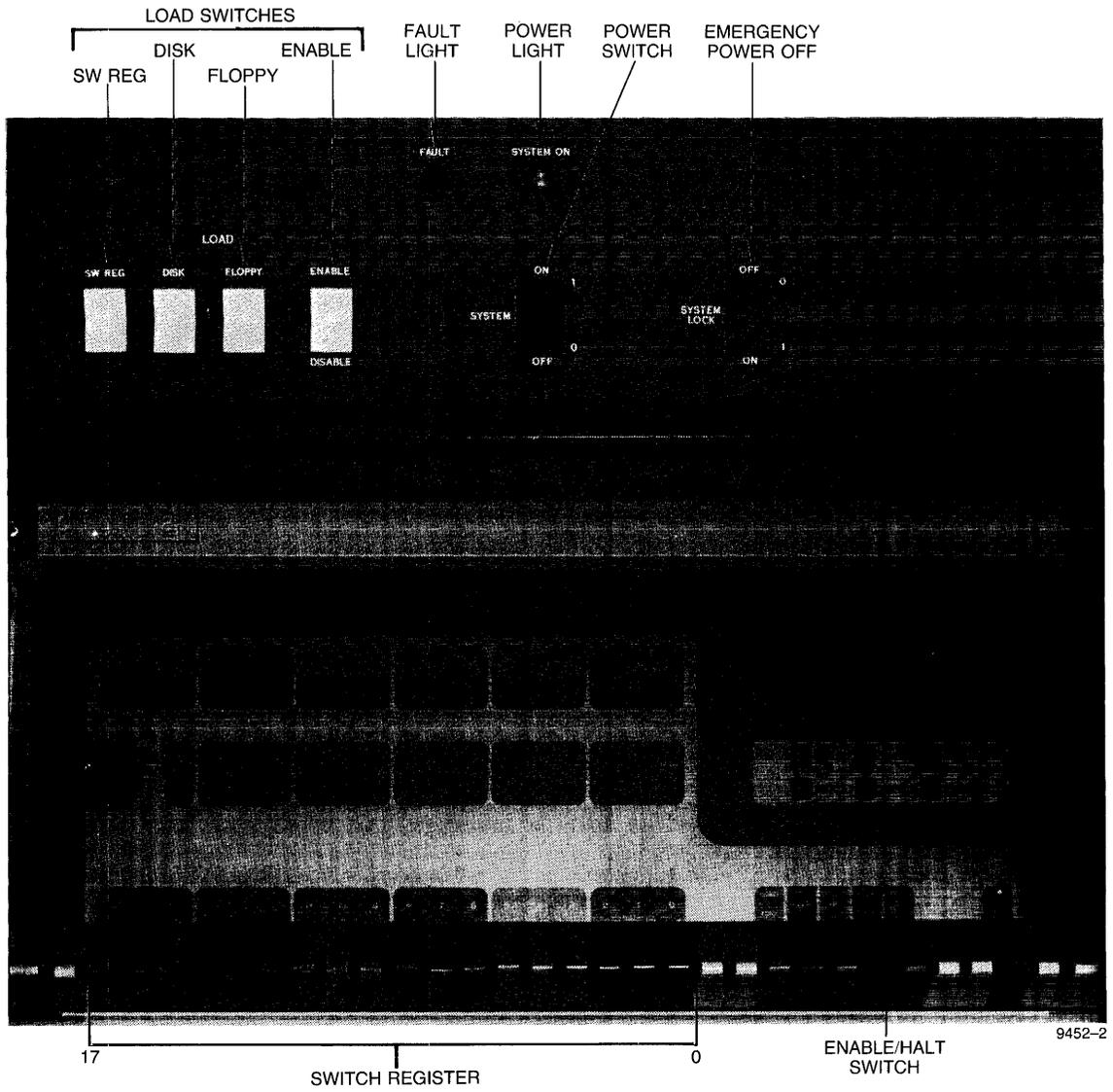
Figure 5-1 Load Switches and Switch Register for KL with Floppy Disks
