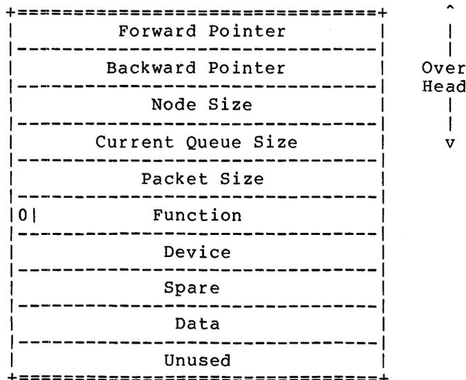
The first four words of the packet are not transferred to the KL. They contain information necessary to manage the queue in PDP-11 memory. The packet that is actually transferred across the DTE-20 during a direct transfer is always 12 (octal) bytes and consists of words beginning with Packet Size and ending with the Data word.
