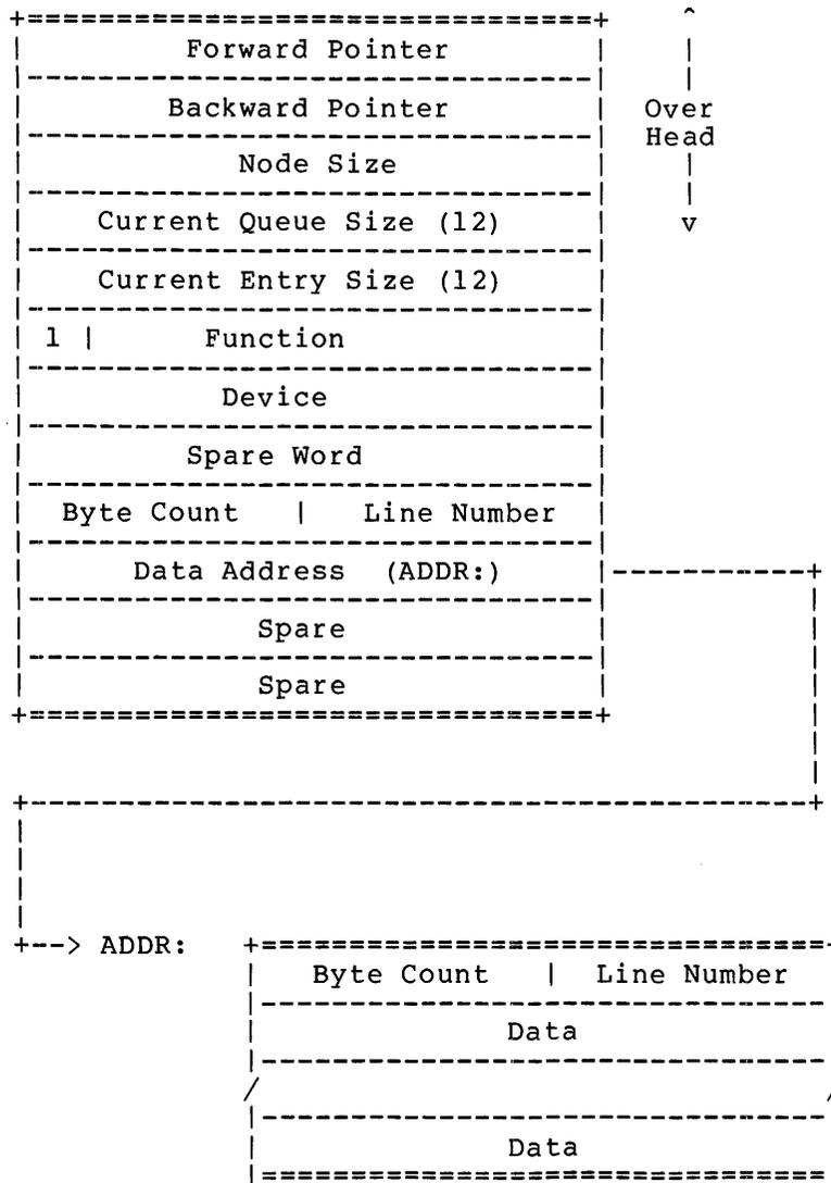
An indirect transfer takes place in two parts; first the header portion and then the data. Not all of the header shown above is transferred across the DTE-20. The Header transfer always consists of 12 (octal) byte starting with the function word and ending with the data address word.
