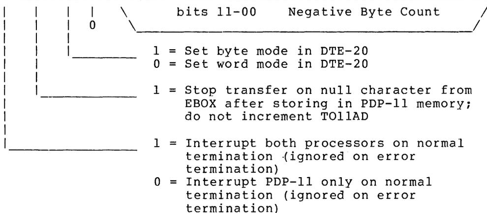
T011BC When the PDP-11 loads this register (the TO-11 byte count) with the number of bytes to be transferred, the DTE-20 begins the TO-11 transfer operation.
