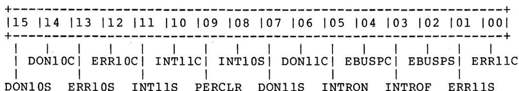
Figure 8-4 DTE-20 Status Word in Write State
