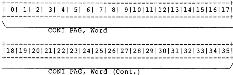
The CMPGWD word is the storage area provided for reading the system status of the Pager. The CONI PAG, instruction puts the status information here. (For more information on the Pager refer to the DECsystem-10/DECSYSTEM-20 Processor Reference Manual.)
