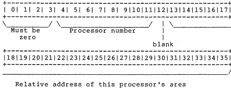
This word is part of the negative extension to the Communications Region. It specifies the location of the PDP-11's owned area by means of an offset from word 0 of the Communications Region.
