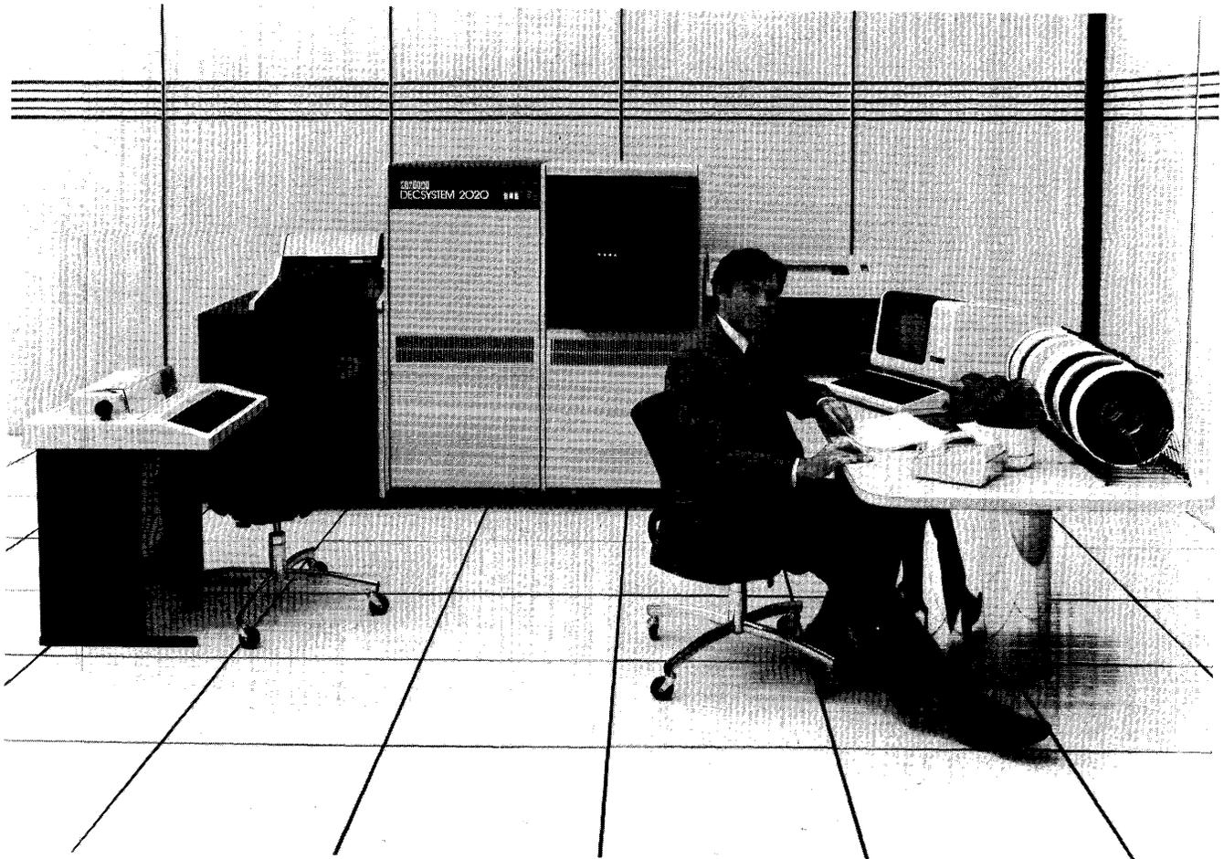
The KS10 central processing unit (CPU) forms the basis of the DECSYSTEM-2020.
