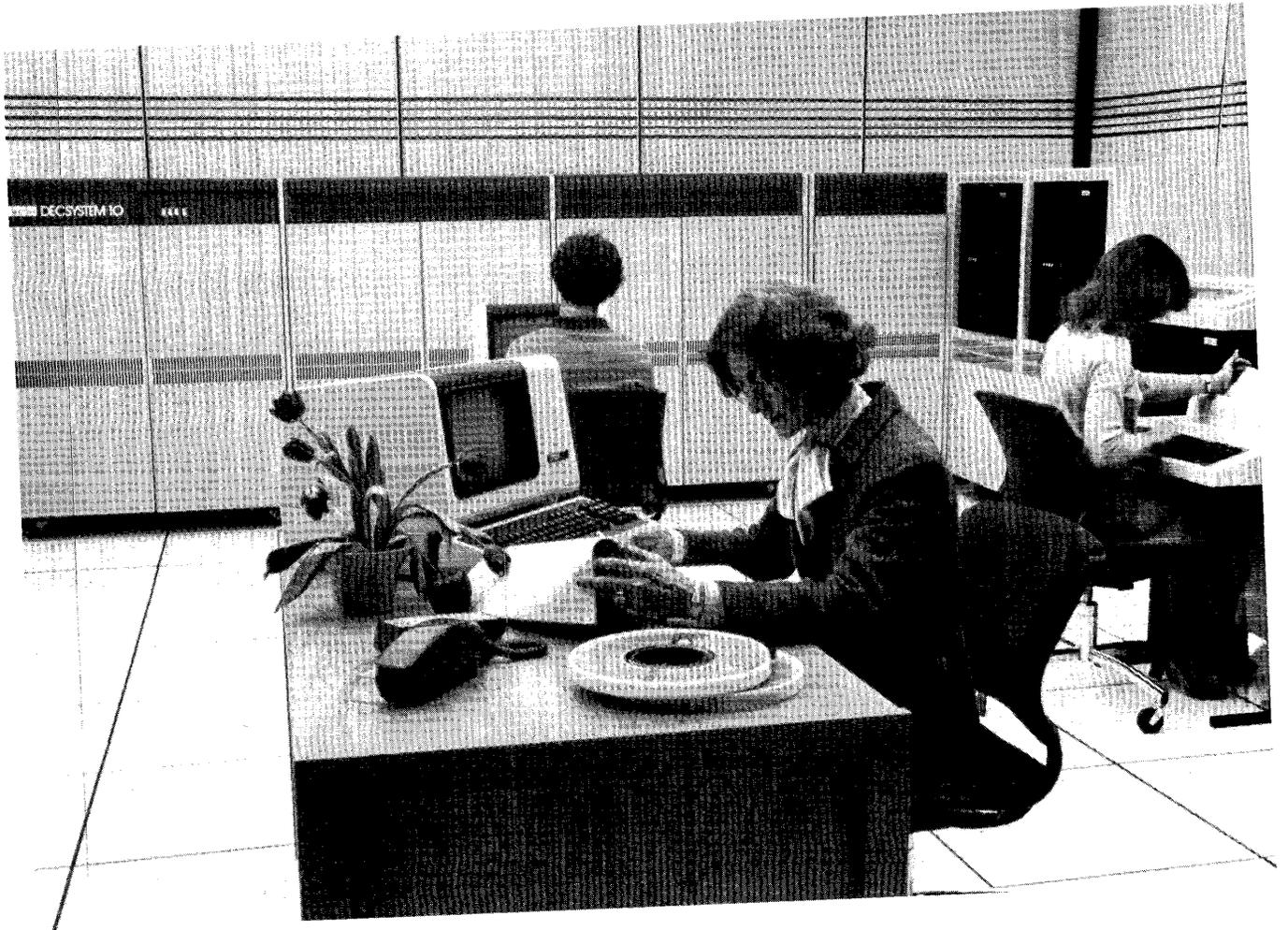
The DECsystem-10 consists of hardware and software that allows the user to run a variety of programs efficiently and conveniently. The system as a whole is designed to execute many different kinds of jobs concurrently.
