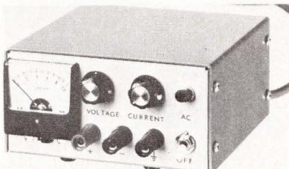
New Power-Pact series of miniature supplies features 0.01% reg. plus front-panel control and metering of output voltage and current-limiting level. Five models are available with outputs of 10, 20, 50, 100, and 150 V at 20 W. Case dimensions are 2½ in. high by 5 in. wide by 5 in. deep. Pacific Radionics. (408) 379-3280.
