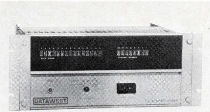
Model 380 system consists of a high level (single ended or differential) multiplexer, a sample and hold amplifier and a binary A/D converter. Its 100 kHz thruput rate applies to both random access and sequential modes of operation. Heart of the system is a Model 301 A/D converter that can digitize an analog signal to a resolution of 15 bits binary, at 250 kHz. Data West Corp. (602) 947-4295.
