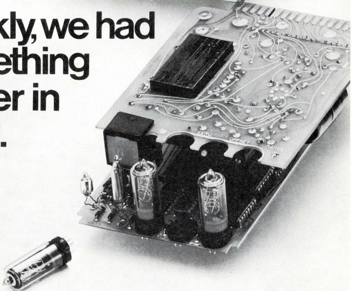
We built our second generation DPM\* to fit into seven square inches of panel. *That's less than any other digital panel meter requires.* But we didn't stop there. The Model 1290 mounts completely from the front of the panel. *The entire chassis pulls out from the front for servicing or replacement.* Even the Nixie\*\* tubes are pluggable! Think of the convenience in continuous systems opera-
