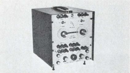
Model TRS-105 ac to dc thermal transfer standard is self-certifiable. Can reference up to 1 kVrms to known dc voltage. Eleven ac ranges. Over-voltage protected. Needs 100-nv f.s. sensitive null detector. \$1500. Julie Res., (212) 245-2727.
