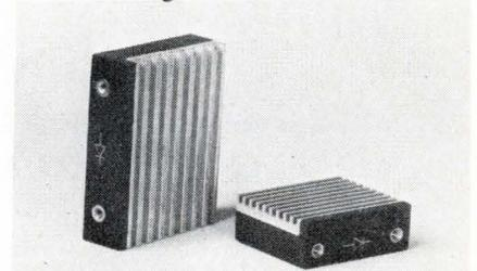
Two new medium power rectifier modules (J531 and J532) dissipate 10 and 20 W respectively in free air (25°C). They may be assembled into many configurations of rated voltage and current. With a  $\frac{1}{4}$  in. min. space between modules they will operate at rated current in 25°C amb. air. Solitron Devices, Inc. (914) 359-5050.
