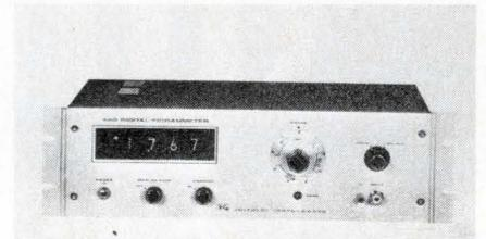
Model 440 has 9 ranges:  $10^{-2}$  to  $10^{-10}$  A f.s. Accuracy,  $\pm 0.5\%$  on sensitive ranges,  $\pm 0.2\%$  on others. 100% overranging, auto polarity and overload indication. Recorder output; printer output optional. \$995. Keithley Instr., (216) 248-0400.
