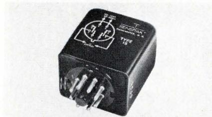
Internal reed switch load contacts respond to phase reversals of input signal. These hybrid modules can often replace more complex, costly, and frequently less reliable components commonly used for transducer sensing, servo-positioning, or sensing and regulating motion displacement in process and machine control systems. Sensitak Instrument Corp. (603) 627-1432.
