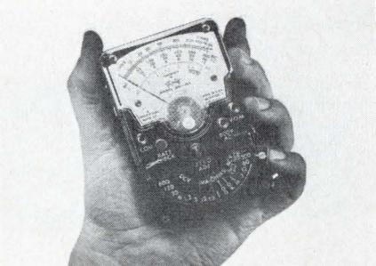
Battery-operated Model 310-FET measures 0.3-600 Vdc in 6 ranges; 3-600 Vac (5k $\Omega$ /V); 0-1.2 mA; resistance to 5 M $\Omega$ . Battery self-test position. Size 2.75 x 4.25 x 1.125 in., 14 oz. User Net, \$70. Triplett, (419) 358-5015.
