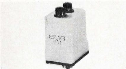
VB series monitors have SS voltage sensors that determine pre-selected under or over voltage conditions and de-energize an internal control relay if these limits are exceeded. The monitor can be used to sound an alarm, light warning lights, or shut down the equipment. A time delay accommodates start-up transients. Diversified Electronics, Inc. (812) 424-2288.
