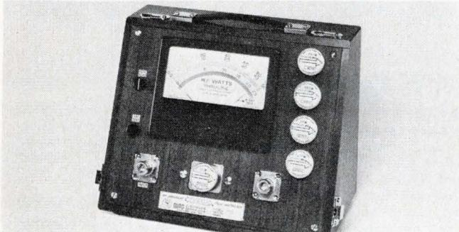
Self-contained Model 4345 samples reflected or forward power. Taut-band meter shows peak power, 250 W to 5 kW, 950-1300 MHz. Accuracy  $\pm 6\%$  of reading at 25 calibrated points. Less than 1.08 insertion vswr. Changeable connectors. Bird Electronics, (216) 248-1200.
