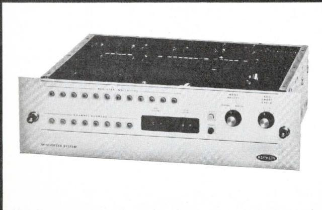
These three new MINIVERTERS™ combine multiplexer, sample-and-hold amplifier and analog-to-digital converter with throughput rate choice of 90KHz, 135KHz or 180 KHz. And each unit goes faster when short cycled; for example, the 180 KHz MINIVERTER runs at 360 KHz with 8-bit resolution.
