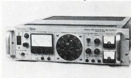
Both ac and dc outputs are superimposed over a 50-dB noise-level filtering. Regulation is 5 mVdc, and 0.25% ac. Outputs are 0-140 Vac, 0-8 Vdc, 500 VA. Fully metered. Model P-5505 costs \$875. Wanlass Instruments, (714) 546-1811.
