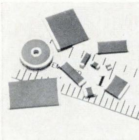
Ceramic chip capacitors are moisture resistant and contamination free in small rectangular, large rectangular, square, and monolithic disk feed-through configurations. Type K-1200 series, available in 51 models, ranges from 10 pf to 1.5  $\mu$ f. They operate from  $-55^{\circ}$  to  $125^{\circ}$ C. D-c working voltages are 50, 100, and 200. Monolithic Dielectrics Inc., Box 647, Burbank, Calif. [346]
