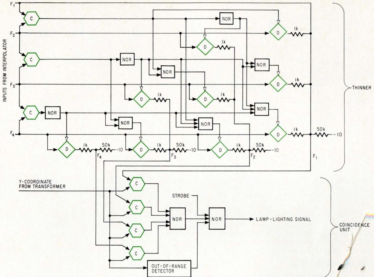
**Thinner.** The four outputs of the interpolator ( $F_1 - F_4$ ) are compared. If two outputs are nearly equal, the thinner eliminates one of them by closing a diamond gate. The coincidence unit compares the four or fewer outputs of the thinner with the Y-coordinate from the transformer, and a lamp in the display is turned on when the comparators detect a matchup.
