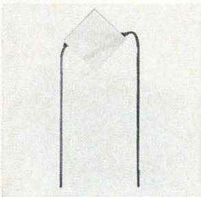
Thermoelectric module 3954-1 spot cools small components and controls temperatures of biological specimens. It is permanently mounted between 2 aluminum plates for mechanical strength and uniform cold junction temperatures. Units measure 4 sq cm with a heat-pumping capacity of 30.6 BTU/hr. Cambridge Thermionic Corp., 445 Concord Ave., Cambridge, Mass. [345]
