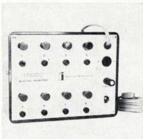
By providing a simultaneous visual indication of the logic states of up to 18 digital or binary circuits, the Logico digital monitor gives the engineer a picture of the operation of discrete or integrated systems. It can be left in the circuit while bread-boarding, and is useful for servicing. Price is \$59.50. Industrial Inventions Inc., RD2 463 US1, Monmouth Junction, N.J. [373]
