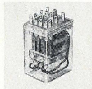
Magnetic latching relay type RR is offered in voltages ranging from 24 to 220 v a-c, and 12 to 110 v d-c. Standard design incorporates 4PDT contacts in fine silver, silver-cadmium oxide, gold nickel, silver palladium (60/40), and silver palladium (30/70). Mechanical life is 100 million operations. Schrack Electrical Sales Corp., 1140 Broadway, New York 10001. [356]
