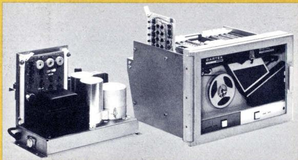
magnetic tape unit can asynchronously record and reproduce eight-bit parallel characters at any rate up to 120 characters per second. It can also record or reproduce characters at a continuous rate of 1600 characters per second. The unit is only 8" x 16" x 9¾" and fits easily into a console or standard rack, and has such impressive standard features as automatic tape loading. It uses 3" reels of ¼" tape for recording, with each reel capable of storing 140,000 characters.
