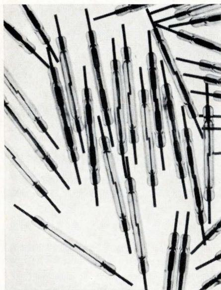
General Radio confirms through its own vendor-component evaluation program that IBM reed switches show zero failures after 25 million operations.
