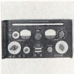
Standard-signal generator type 1003 covers 67 khz to 80 Mhz, with calibrated output of 0.1  $\mu$ v to 6 v behind 50 ohms. Total warm-up drift is typically 150 ppm in 3 hours, and drift after the warm-up period is typically 1 ppm per 10 minutes. Price, including the automatic control package and crystal calibrator is \$2,995. General Radio Co., West Concord, Mass. 01781. [370]
