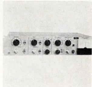
A phase-sensitive detection system recovers signals 51 db below ambient white noise in a 1-khz bandwidth. Model 120 lock-in amplifier operates as an amplifier-detector-filter combination with an equivalent over-all noise bandwidth of 0.0083 hz. Minimum full-scale sensitivity is 100  $\mu$ v. Price is \$765. Princeton Applied Research Corp., P.O. Box 565, Princeton, N.J. [388]
