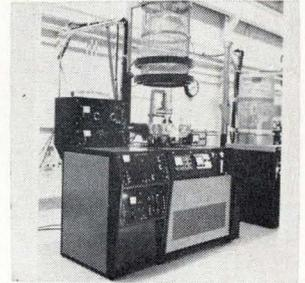
Designated the Plasma Vac AST1 300, a reactive sputtering system features 2 parallel-mounted water-cooled disk electrodes. The target electrode and discharge suppressor are in the upper position and the substrate-table electrode in the lower. An r-f supported plasma discharge is used to ionize the gas. Consolidated Vacuum Corp., 1775 Mt. Read Blvd., Rochester, N.Y. [428]
