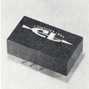
Operational amplifier OA-125 is stable at closed-loop gains of unity or greater, and provides a gain-bandwidth product of 125 Mhz. It is suited for linear applications as well as those involving nonlinear elements in the feedback loop, such as threshold circuits. Price is \$135. Computer Labs Division, Strandberg Engineering Laboratories Inc., 1109 Valley Park Dr., Greensboro, N.C. [386]
