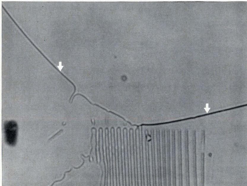
**Bell Laboratories' model (200x) permits physical simulation of a eutectic phase diagram for an alloy such as lead-tin. Diagram relates liquid proportions (horizontal scale) to temperature (vertical).**
