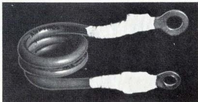
When heated above 621 F, Type E-125 TEFLON® tape sinters to form a rigid, tough, hermetic seal around coils, cables, or other forms. It won't burn either. Teflon just melts. Available in thicknesses from 0.002" to 0.010" and widths from 1/8" to 3", with tensile strengths from 1100 to 1800 PSI and dielectric strength from 700 to 800 VPM.
