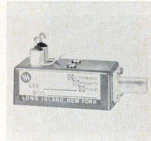
Fundamental voltage-tuned oscillator model ETS3152 has a tuning range of 1.2 to 1.8 Ghz. Linearity is within  $\pm 1\%$  over 75% of the range. The devices, 1 x 1 x 2 $\frac{1}{4}$  in. provide a power output of 50 mw c-w. Noise is -70db, and harmonics approximately -15 db, Microwave Products Division, Consolidated Airborne Systems Inc., 115 Old Country Rd., Carle Place, N.Y. [404]
