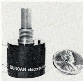
Ten-turn wirewound pot model 3253 PixiePot is 7/8 x 3/4 in. and weighs 1/2 oz. Resistance tolerance is ±5% over 100 ohms to 100 kilohms. Linearity is ±0.25% and resolution is typically 0.222. Units are rated at 2w at 25°C. Price is \$5.95 in lots of 1 to 24; less than \$4 in production quantities. Duncan Electronics Inc., 2865 Fairview Rd., Costa Mesa, Calif. [353]
