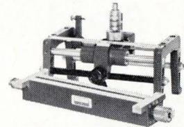
**Coaxial slotted line** for traditional swr measurements in coax 1.8 to 18 GHz. Very low residual swr (<1.04 at 18 GHz) results in high-est accuracy. Model 816A, \$250. (Used with 809C Carriage, \$200, and 447B Detector, \$125.)
