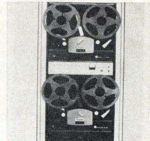
Multichannel recorder-reproducer model 248 is for communications in air traffic control, fire and police service, and other specialized uses in government and industry. It is expandable as logging needs increase and is equipped with 4,800 ft of tape on 10 $\frac{1}{2}$ -in. diameter reels and allows 24 hours of recording time at 0.653 ips with each transport. Dictaphone Corp., Rye, N.Y. [384]
