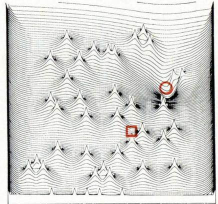
**Sidestepping.** Path shown in color indicates the connection between the two peaks. Sidestepping is caused by obstacles along the way. At right, target peak is again pulled down at a later stage of the process and the terrain examined for other connecting paths. Heavy black vertical lines and horizontal plateaus indicate several paths already completed.
