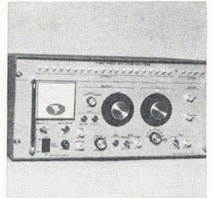
Fully automatic shock spectrum analyzer model N980 is designed for lab or field use. Accuracy is  $\pm 3\%$  (any model), and frequency response is  $\pm 0.5$  db. The unit spans 1 to 10,000 hz. Frequency intervals are selected by pushbutton in ½-octave increments or by vernier control. Dynamic range is 60 db. MB Electronics Inc., 781 Whalley Ave., New Haven, Conn. 06508. [368]
