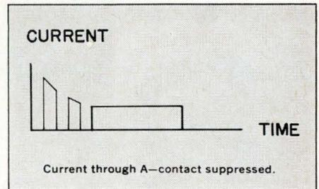
Another major process which causes material transfer in reed switches is arcing.
