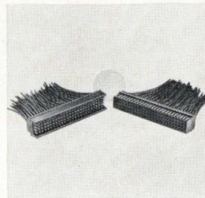
Miniature phenolic connectors offer from 4 to 104 circuits in multiples of 4. They have aligning ribs to assure positive polarity. The connectors are UL recognized to 250 v a-c at 5 amps average per contact. They can be used by manufacturers of computers, communications equipment, and consumer-type equipment. Molex Products Co., 5224 Katrine Ave., Downers Grove, Ill. 60515. [352]
