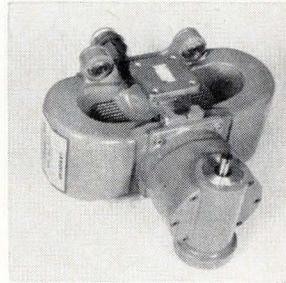
Tunable coaxial magnetron SFD-325, for airborne and ground-based radar systems, has a frequency range of 16 to 17 Ghz, and peak output power of 75 kw. Compatibility of the tube with modulators delivering widely varied pulse shapes is assured by the low pushing factor (60 khz/amp). Duty factor is 0.001. S-F-D Laboratories Inc., 800 Rahway Ave., Union, N.J. [403]
