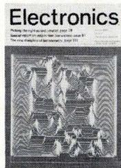
A computer program that views a printed circuit as a three-dimensional map (cover) speeds its efficient design. The program, developed under Atomic Energy Commission auspices, takes component descriptions and hand-drawn circuit schematics as its inputs and delivers complete specifications for wiring paths and component positioning.
