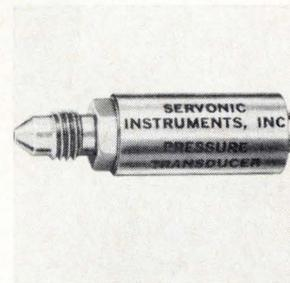
The Minduser measures 0.5 x 1 in. and is available in pressure ranges from 0-500 to 0-10,000 psia and psig. Used primarily for airborne telemetry and control, it monitors air, fuel, and other media compatible with its NiSpanC sensing element. Over-all accuracy is  $\pm 1.75\%$ . Servonic Instruments, subsidiary of Gulton Industries Inc., 1644 Whittier Ave., Costa Mesa, Calif. [376]
