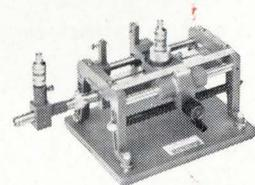
**Coaxial swept slotted line system** retains high accuracy resulting from 816A Slotted Section's low residual swr while you make **swept frequency swr** measurements from 1.8 to 18 GHz. This technique is described in HP Application Note 84, yours for the asking. Model 817A, \$925.
