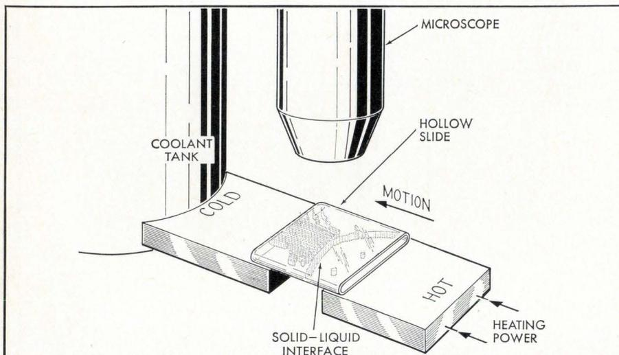
**Experimental setup in which photographs such as that below were taken. The glass slide or cell—containing a liquid which freezes like a metal—is placed between hot and cold blocks of brass. This produces a temperature difference along the slide. A solid-liquid interface then forms between the two blocks. By moving the slide toward the cold block at a constant rate, one can observe the steady growth of the crystal under the microscope.**
