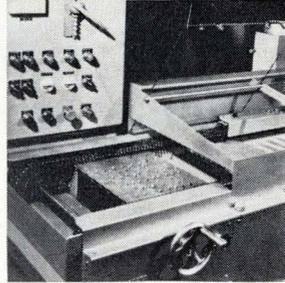
Integrated wavesolder system 364 has an adjustable conveyor, eliminating the need for board carrier or pallet. A p-c board from 2 to 15 in. is slipped into the conveyor and firmly held as it passes the fluxing, flux-drying, preheating, and soldering stations. The system is suited for white room use. Electro-Mechanical Division, Electrovert Inc., 86 Hartford Ave., Mt. Vernon, N.Y. [426]
