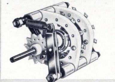
**MODEL 86 NON-SHORTING SWITCH FEATURES (Illustrated):** 7000 volt peak flashover at 60 cps • 20 ampere current carrying capacity • Current carrying members heavily silver plated • Coin silver contact shoes • Low loss silicone impregnated stator and shaft • Black anodized aluminum support brackets • Nylon detent wheel
