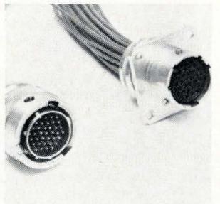
Circular connectors type ESM are bayonet locking, subminiature, and have a high contact density (0.080 in. center-to-center). They come in a 37-contact version in a No. 12 shell, and a 92-contact type in a No. 18 shell. Contacts are rated at 5 amps. They accept 22-, 24- or 26-gauge wire and are accessible from the rear of the connector. Elco Corp., Willow Grove, Pa. 19090. [348]
