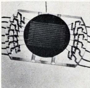
Gold-stripped semiconductor detector 5441 on an n-type silicon disk is used for studying the structure of a beam of charged particles. It may be used in a beta spectrometer for the simultaneous measurement of electrons with slightly different energies. Resistivity is greater than 10,000 ohm-cm. Energy resolution is less than 35 kev. AB Atomenergi, Studsvik, Nyköping, Sweden. [440]
