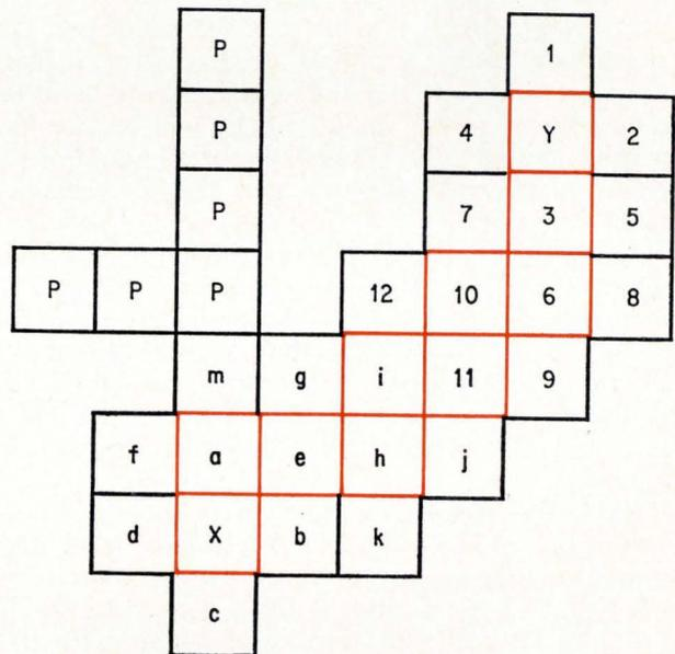
**Step selection.** With the X and Y squares representing the peaks between which a path is to be completed, the computer scans the area between them. Steps are chosen in the most downward direction from both X and Y. The squares surrounding the two peaks represent various lower altitudes. Steps can only be taken vertically or horizontally. They can neither be on or adjacent to steps of a different path nor retrace a previous step. The completed path is shown in color.
