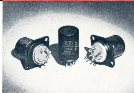
The LT Series relays provide hi-level performance in a subminiature hermetically sealed housing — space saving without loss of performance. Meets military standards. **Features:** height above mounting panel 40% of standard relays (7 pin flange mount); time delays, 2 to 75 sec.; operating temp., -65°C to ±85°C; operating voltages, 6.3 to 115V AC or DC.
