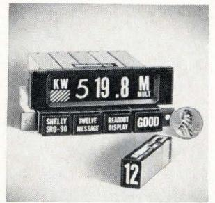
Ultraminiature rear projection readout SR-90 has 12-message capability. It reads out symbols, characters, or up to 4-line messages 0.1 in. high. Front dimensions are 0.650 x 0.460 in. Lamp replacement is accomplished from the front panel, by removing the readout from the housing assembly. Shelly Associates Inc., 111 Eucalyptus Dr., El Segundo, Calif. 90246. [344]
