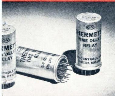
Each enclosed thermal time delay is shock proof and shatter proof — designed for industrial applications requiring reliable operation and long life. **Features:** temp. compensated; time delays, 2 to 180 sec.; heater voltages, 6.3, 26, and 115V. AC or DC; contacts, SPST, NO or NC.
