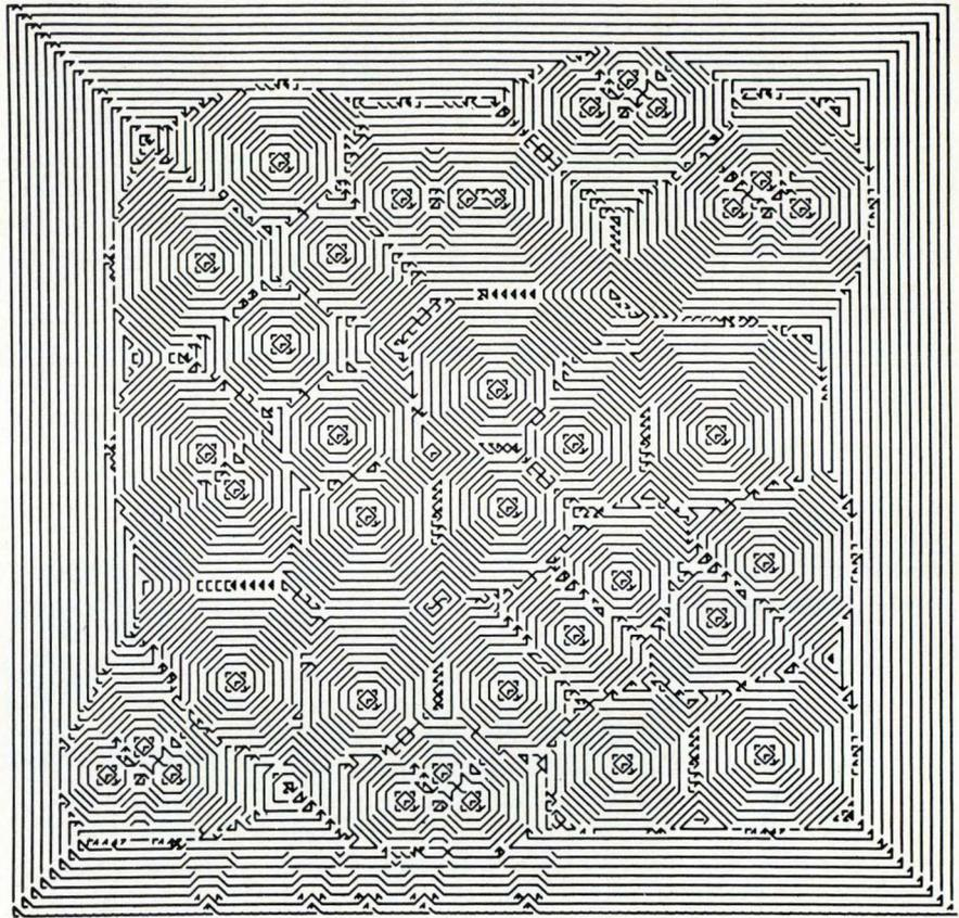
**Contour map.** Top view of initial layout of basin and peaks for a particular circuit at the start of the computer run. Peaks represent component conductor pins and the basins represent the possible conductor paths.
