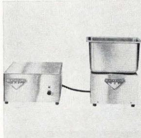
Ultrasonic cleaners for p-c boards and components come in tank capacities of  $\frac{1}{2}$  and 1 gallon. Each cleaner consists of the tank (detachable for cleaning); the transducer assembly, which induces cavitation in the tank; and the generator, which powers the transducer. The tank is for use with water-base detergents. Blackstone Ultrasonics Inc., 25 Barrett St., Sheffield, Pa. [425]
