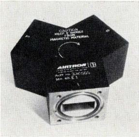
Designed to operate in X band in WR-12 waveguide, model 336505 is a 3-port junction circulator with a peak power of 300 kw and an average power of 300 w. Suitable as a circulator, isolator, or duplexer, it offers insertion loss of 0.3 db, isolation of 20 db, and vswr of 1.20. Price is about \$350. Airtron Division, Litton Industries, 200 E. Hanover Ave., Morris Plains, N.J. [401]
