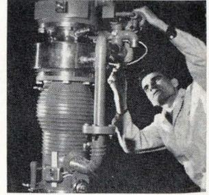
Vacuum pumping module 3352 pumps about 900 liters per sec. This allows more rapid production operations in vacuum metalizing, IC deposition, high temperature furnaces, and space simulation equipment. The module measures  $35\frac{1}{2} \times 21\frac{1}{2} \times 27$  in. It uses a 6-in. diffusion pump. Price is about \$2,000. National Research Corp., 160 Charlemont St., Newton, Mass. 02161. [424]
