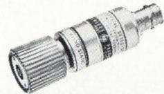
**Crystal detector** provides wideband detection from 10 MHz to 18 GHz. Use for leveling and monitoring applications. Has low swr and very flat response ( $\pm 1$  dB full range). Model 8470A, APC-7, \$175; Type N, \$160.
