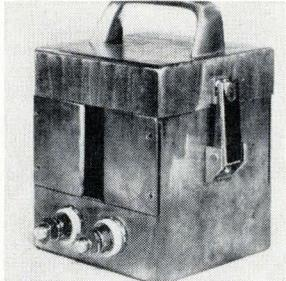
An injection-current probe can be clamped around d-c, 60 hz or 400 hz power lines carrying up to 300 amps, without altering their transfer characteristics. Designated GIP7418, it is also capable of injecting 1 amp from 100 hz to 100 khz into a circuit using an audio amplifier as the source. Genistron Division, Genisco Technology Corp., 18435 Susana Rd., Compton, Calif. [366]
