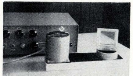
**Playing the angles.** Crystal at right is rotated by stepping motor whose controller is at the rear. Six arc minutes of rotation change incidence angle of laser beam enough to separate holograms.
