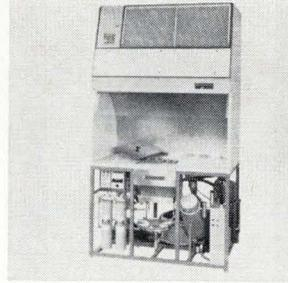
A cleaning station called Micro-Cleaner helps reduce rejects of ICs. It provides 5 hot, cascading rinses and a final rinse of hot, ultrapure water in a totally clean environment. The recirculating, re-purifying system includes a built-in still, demineralizer, organic removal bed, 0.1-micron particle filter, and storage sump. Barnstead Still & Sterilizer Co., 2 Lanesville Ter., Boston. [427]
