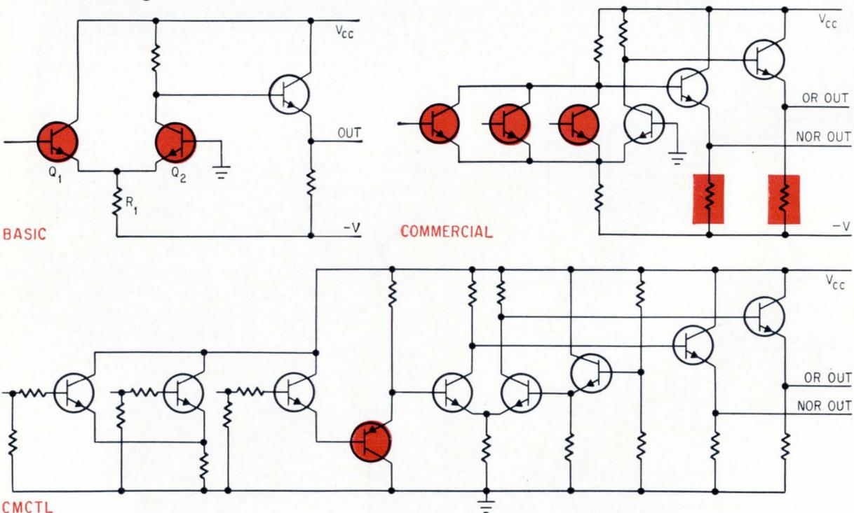
Basic current-mode logic gate, top left, operates as differential amplifier with constant current through  $R_1$ . At the top right, commercial version has emitter-coupled input gate. Added emitter-follower stage provides inverted (NOR) output. Logic swing is boosted in the bottom circuit, current-mode complementary transistor logic, CMCTL, and only one supply voltage is needed, through the use of pnp transistor.
