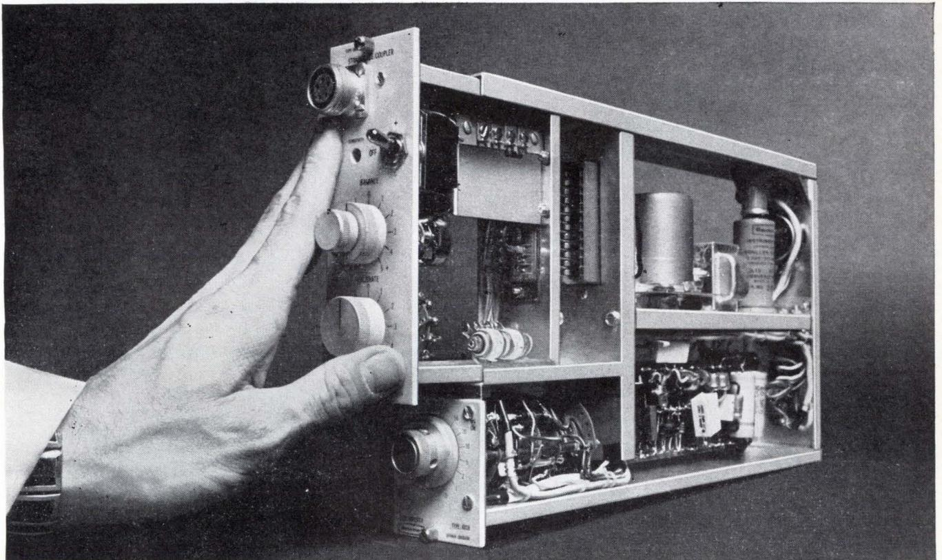
Record directly . . . strain . . . pressure . . . displacement . . . temperature . . . or any other phenomena that can be transduced into an electrical signal. The Beckman 9800 Series Input Couplers (over 30 of them) plug directly into the preamplifier in the Dynograph® Recorder, averting heavy expenditures for specialized amplifier systems when your application needs change.
