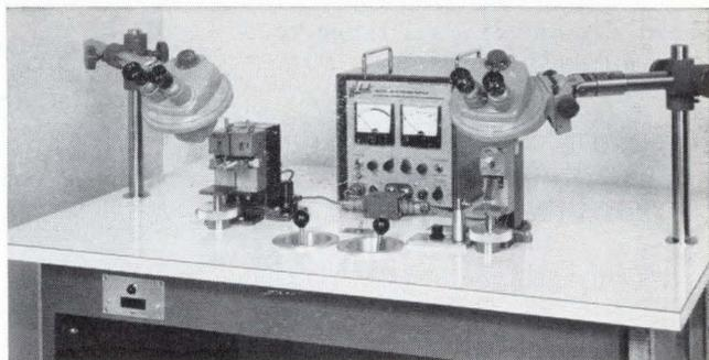
Weltek's new Model 750 can be set up in minutes to do micro-miniature welding, controlled soldering or "nail head" bonding. With this one piece of equipment you can solder or weld flat packs to p.c. boards, do module welding, point-to-point microsoldering or bond a wire to a transistor chip! The possibilities are unlimited. The 750 can do *all* of your miniature joining work... in the lab or in production. And it is reasonably priced.
