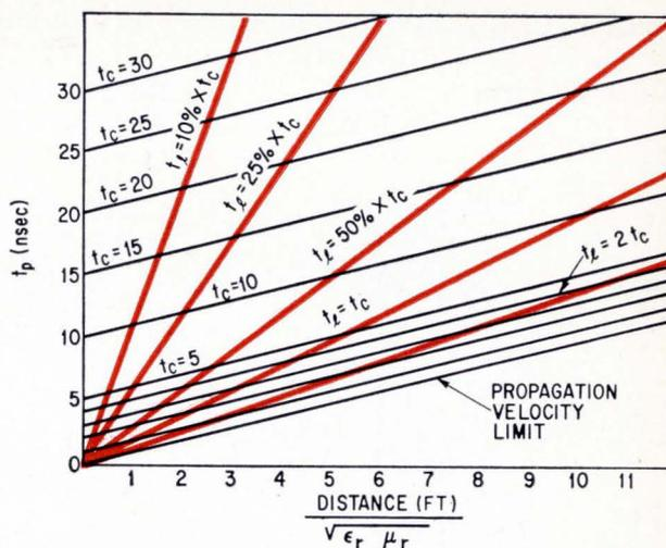
**Trade off between system logic delay,  $t_p$ , and interconnection lengths between IC's.** Delay resulting from IC is  $t_c$ , while delay caused by the interconnecting media is  $t_i$ . The line lengths are normalized for relative permittivity and permeability of unity.
