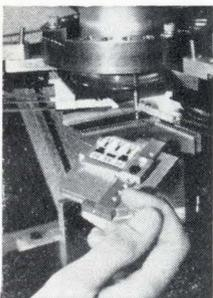
Production rates of 600 trims per hour are attainable with this new, complete system which automatically trims and tests resistors to any specified value within 0.5%. Once operator has placed module in position, checking, trimming, and inspection are automatic. Complete cycle requires from one to three seconds, depending on programmed tolerance and the amount of material to be removed.
