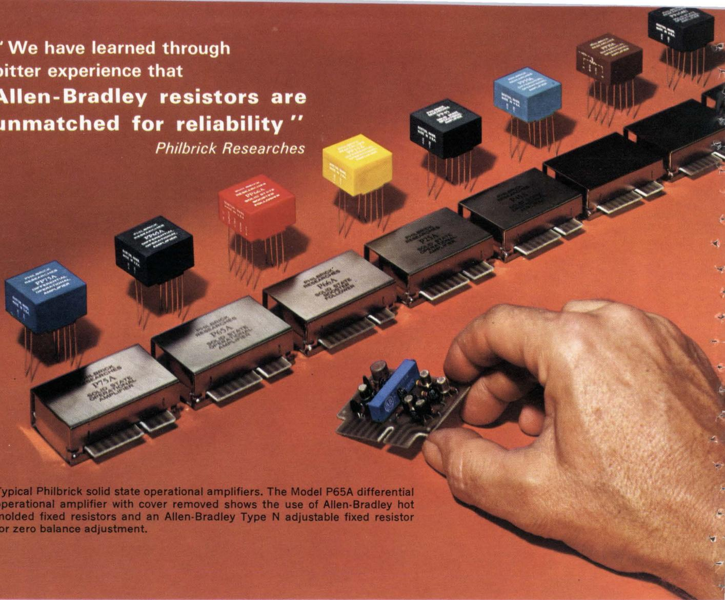
Typical Philbrick solid state operational amplifiers. The Model P65A differential operational amplifier with cover removed shows the use of Allen-Bradley hot molded fixed resistors and an Allen-Bradley Type N adjustable fixed resistor for zero balance adjustment.
