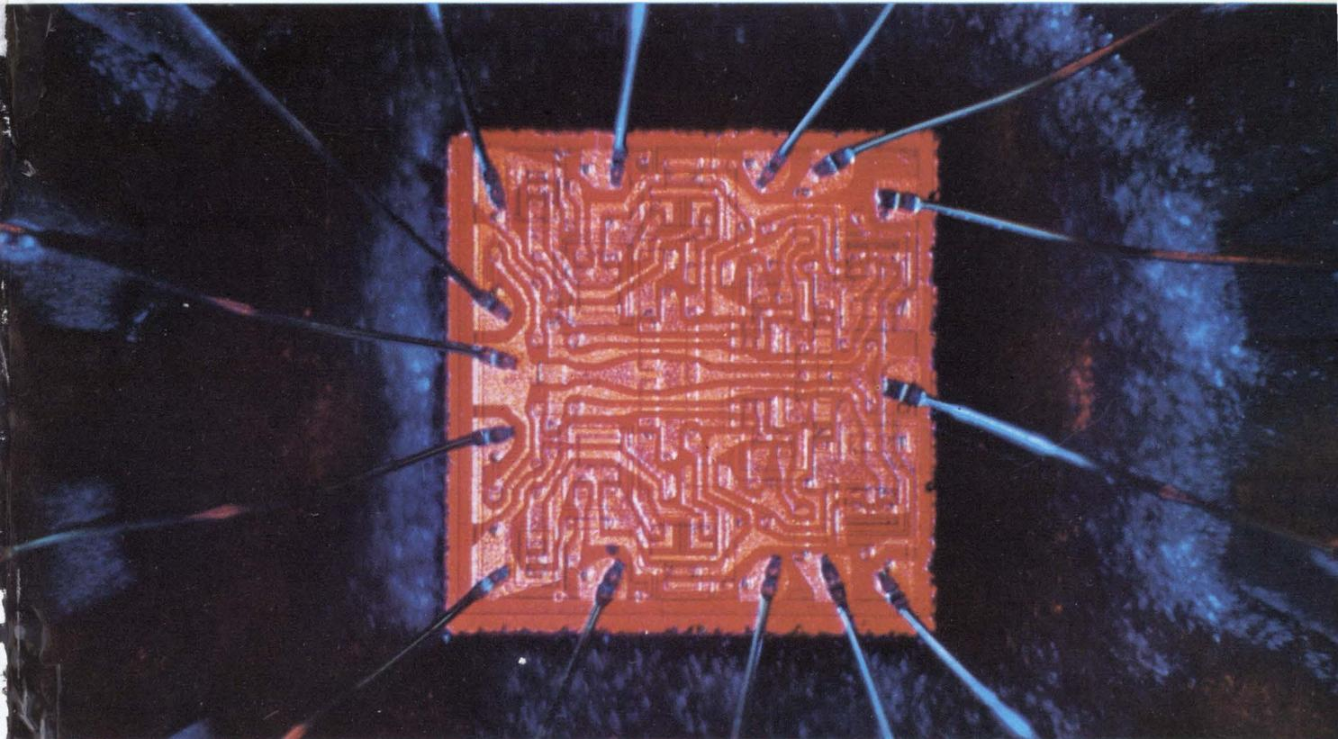
**Dual J-K flip-flop** contains 28 transistors, 38 resistors. The RTL device is a complete general-purpose storage element designed by Fairchild Semiconductor for industrial shift registers and binary counters.
