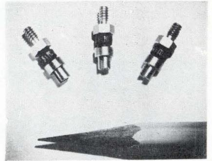
square wave frequencies as high as 40 khz, or even higher sine wave frequencies for new miniature rectifiers. They offer a 9-amp current rating and peak inverse voltage up to 400 v with all models having controlled avalanche characteristics. Surge ratings are as high as 150 amps for one cycle.
