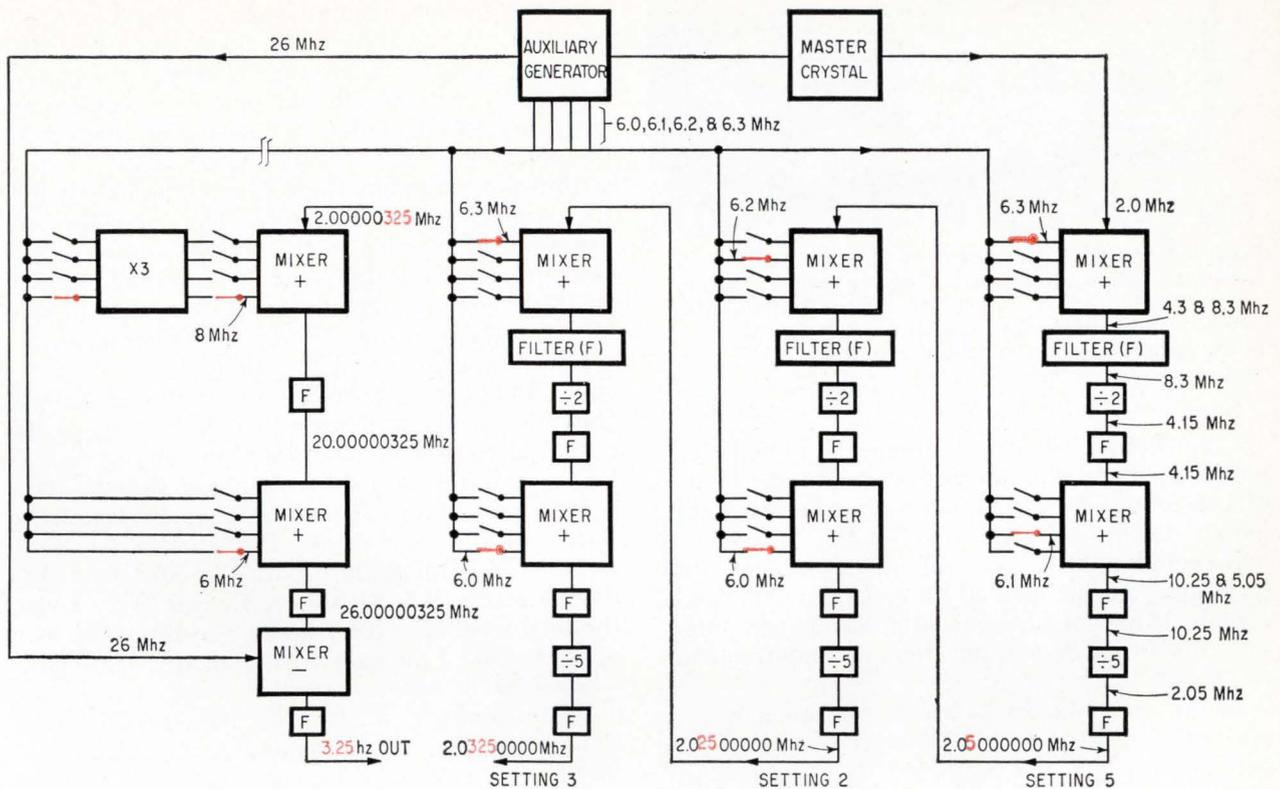
**Decade modules** mix signals produced by crystal oscillator to produce desired output—3.25 hertz in this example. Selecting the desired frequency closes various switch-contacts to feed the proper slave frequencies into mixer. Decimal portion (in color) of each decade's output is shifted one digit to the right as it progresses.
