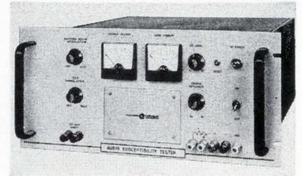
Two modulation-modes—random noise and external input—are available in a solid state 5 amp d-c power source that has output voltage adjustable from 18 to 37 v. The instrument is designed for electromagnetic compatibility testing and can simulate abnormal power supply conditions for checking equipment performance.
