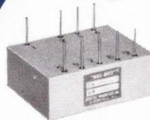
This G/M extremely low level signal current magnetic modulator operates from 0 to  $\pm 1 \mu$ a DC full scale with a frequency response of 0 to 100 cps minimum for a carrier excitation of 400 cycles. Excellent zero point, amplitude and phase angle stability with respect to line voltage, frequency and temperature range.
