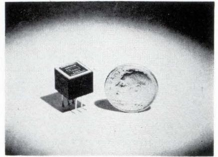
microminiature operational amplifier packaged in a case  $\frac{3}{8}$  x  $\frac{3}{8}$  x  $\frac{1}{5}$  in. Model KM-23M amplifier is designed for commercial and industrial use in analog computers, high-gain/low-drift servopreamps, high stability a-c amplifiers, voltage comparators, and similar applications.
