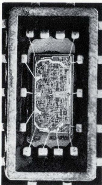
Complex functions like this will be part of the Series 54 line. First product will be a quadruple binary latching circuit with four flip flops on a chip.
