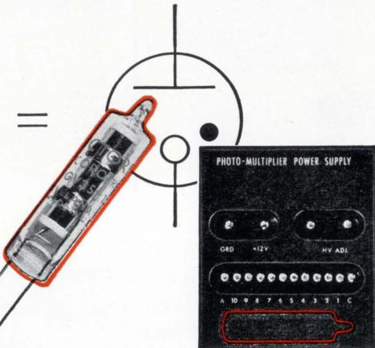
Corotron actual size: Photo-multiplier power supply, showing Corotron location, 1/3 size.
