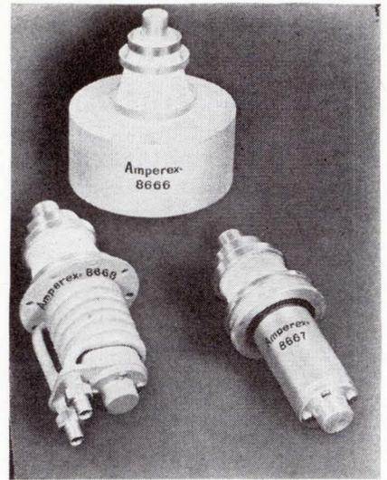
ries 8666, 8667 and 8668 with 10-kw dissipation. Each series is either air-cooled or water-cooled. Water cooling is accomplished with a conventional water jacket or with an integral helical coil attached directly to the tube anode. The helical cooled version offers a substantial reduction in water consumption.
