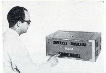
Bidirectional counters furnish accurate, high-speed determination of dimension, travel or position along one or two axes of motion. Primary application is for machine tools, layout and plotting machines and similar equipment where lead screw rotation can be monitored to provide a direct and continuous display between stationary and movable members.
