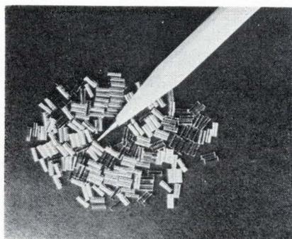
Semiconductor manufacturers will benefit from an alkali-free sealing glass for use with Kovar or molybdenum. The material, called AFG-47, not only is alkali-free but also has a high lead content providing much greater resistivity at elevated temperatures, and has a longer working range. Resistivity, expressed as the logarithm of ohm-centimeters is 11.8 at 250°C and 10.2 at 350°C; thermal expansion
