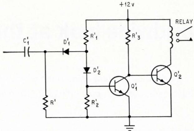
**Conventional high-gain pulse amplifier** generates output pulses whose duration is determined by the time and amplitude of input pulses together with time constant  $R_2C_1$ .
