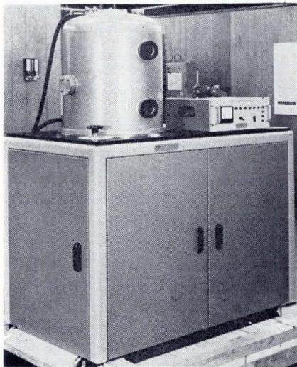
A fully automatic high-vacuum evaporator for producing thin film components can reach to pressures of less than  $5 \times 10^{-8}$  torr in a 20-inch diameter bell jar. Fast cycling time is achieved with liquid nitrogen and a 1900-liters-per-second oil diffusion pumping system. The pumping system is made fail-safe with an interlocked automatic valve control.
