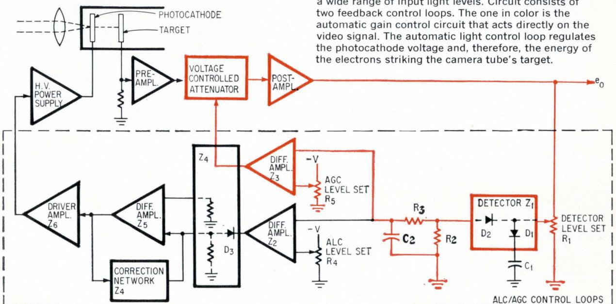
ALC/AGC control circuit holds video output constant over a wide range of input light levels. Circuit consists of two feedback control loops. The one in color is the automatic gain control circuit that acts directly on the video signal. The automatic light control loop regulates the photocathode voltage and, therefore, the energy of the electrons striking the camera tube's target.
