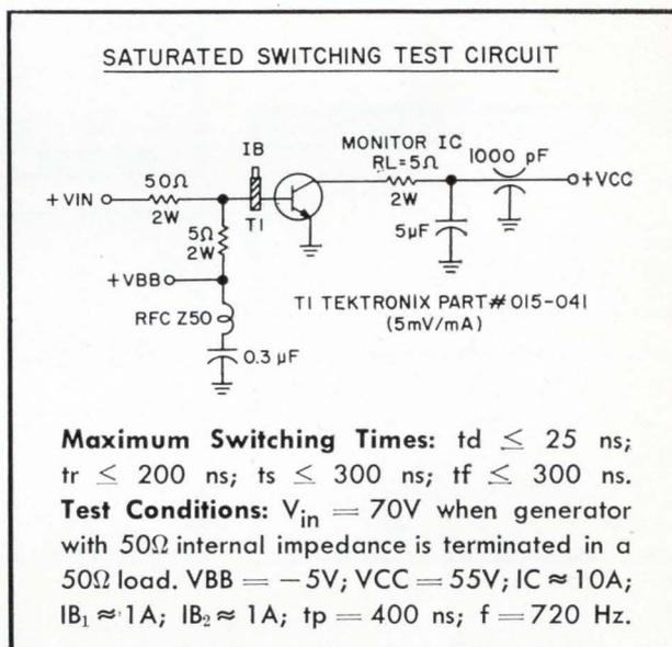
You'll find over 100 types to choose from. With IC's of 3, 5, 10, 15 and 20 amps, and VCEO from 40 to 100 volts. Low saturation at high current, and low thermal resistance provides more useable power. There's sure to be one suited for your high current switching or amplifier application. Bendix silicon planar power NPN transistors come in six different package configurations, too.
