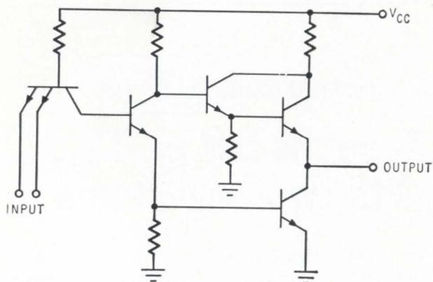
Typical two input TTL gate circuit used in the new high-speed Texas Instruments' Series 54H logic line.
