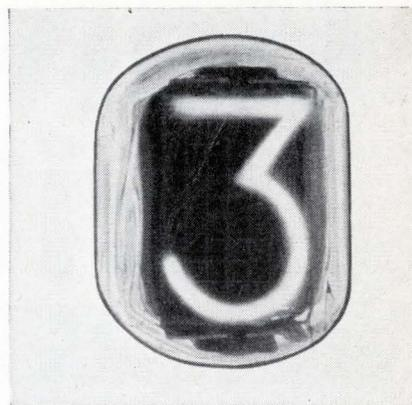
**Datavue\* End-View Tubes.** These tubes are easily read in high ambient light—do not wash out like other displays. Erroneous readings due to segment failure do **not** occur because the characters are fully formed. Raytheon Datavue End-View Tubes fit existing sockets and conform to EIA ratings. Models include round (CK8421) and rectangular (CK8422). Ultra-long-life types are designed for 200,000 hours or more of dynamic operation.
