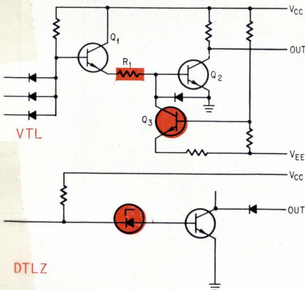
Variable-threshold logic, at the top, in which supply voltages are set at high or low values to provide high or low noise rejection.  $R_1$  replaces level-setting diodes of DTL, and  $Q_3$  acts as constant-current source. Zener diode in the DTLZ circuit, below, replaces conventional diodes to boost noise threshold to about 6 v, but power and propagation delay zooms.
