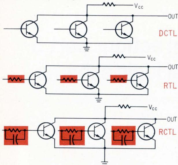
Collector-coupled or current-sourcing logic types include, from top to bottom, direct-coupled, resistor-coupled, and resistor-capacitor coupled transistor logic, abbreviated DCTL, RTL, and RCTL, respectively. The resistors in RTL overcome current hogging, while the RC input in RCTL avoids current hogging and, theoretically, improves speed.
