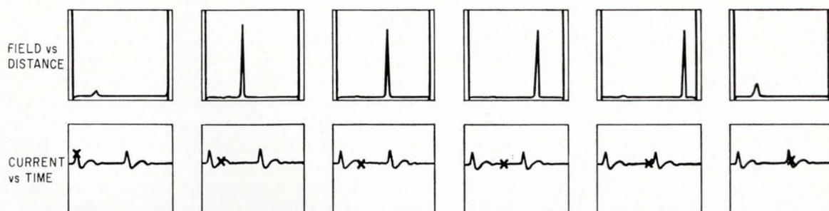
Several frames of computer-produced motion picture show how the dipole layer propagates through the sample after being nucleated at a point where the doping is 10% lower than the doping throughout the rest of the sample. The X's on the current curve show the current at the instant which is pictured in the field distribution plot. The time between frames is about 0.6 nanosecond. The repetition frequency is 680 megahertz.
