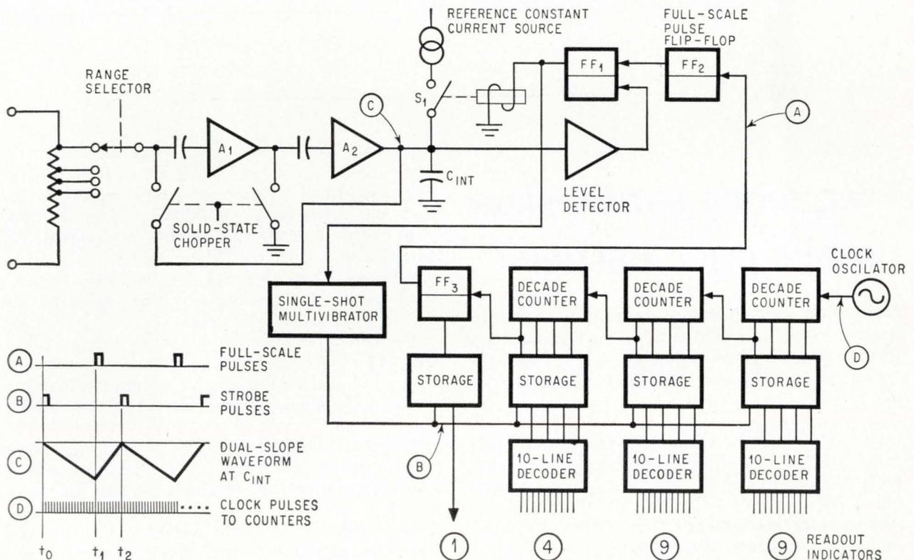
To measure voltage, multimeter measures the time required for the constant-current reference to discharge the integrating capacitor to zero volts after it has been charged to an initial value by an input voltage. The level detector senses the moment when  $C_{int}$  reaches zero volts and generates a strobe pulse to transfer the count from the counters to the readout and restart the measurement cycle.
