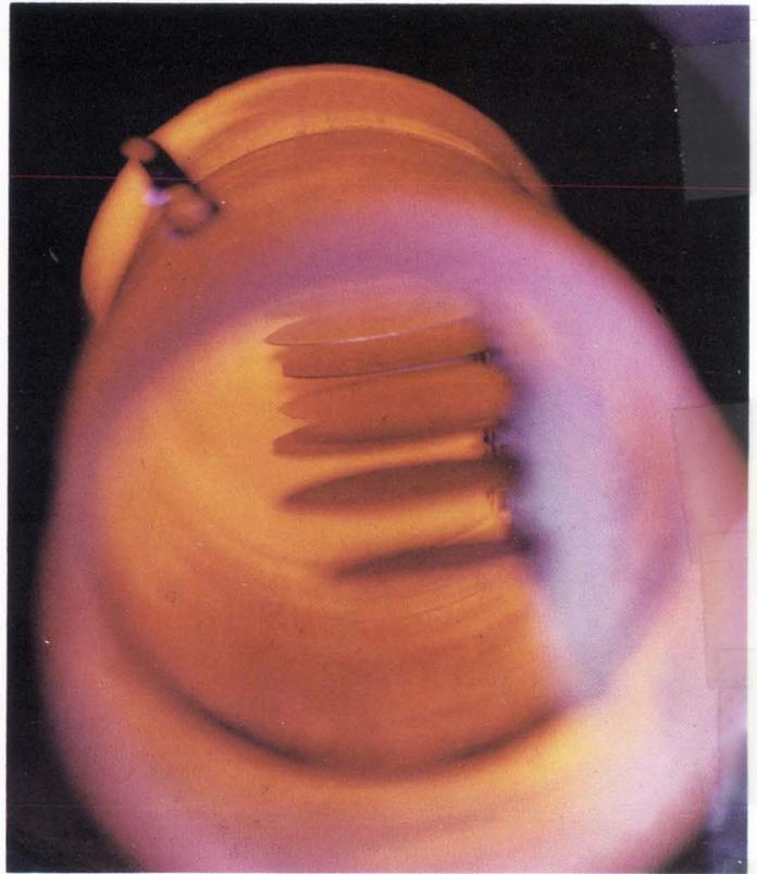
Digital IC wafers undergo diffusion in Honeywell furnace.
