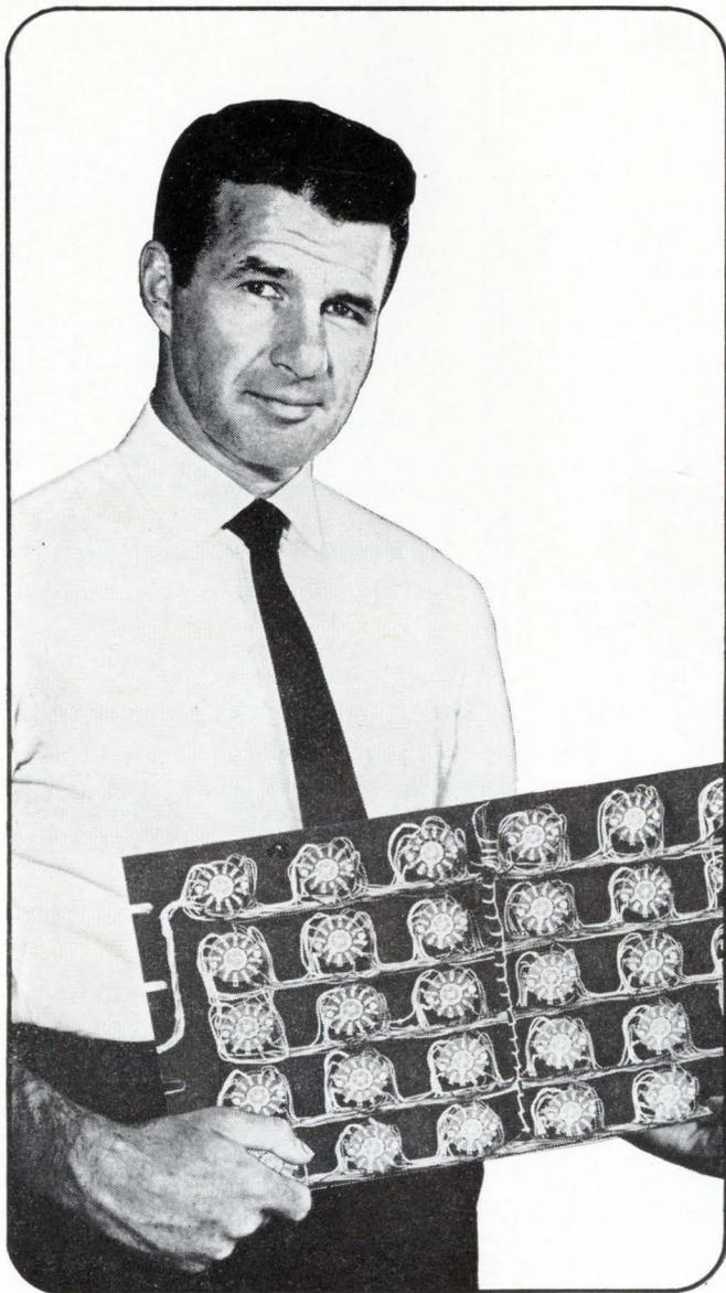
**USING ROTARY SWITCHES** requires 330 soldered joints . . . over 8 hours of labor . . . occupies 293 square inches of panel space . . . costs \$88.00 installed.
