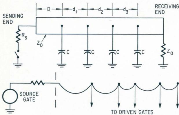
Tapped or daisy-chain fan-out technique requires high impedances to match the logic circuits.
