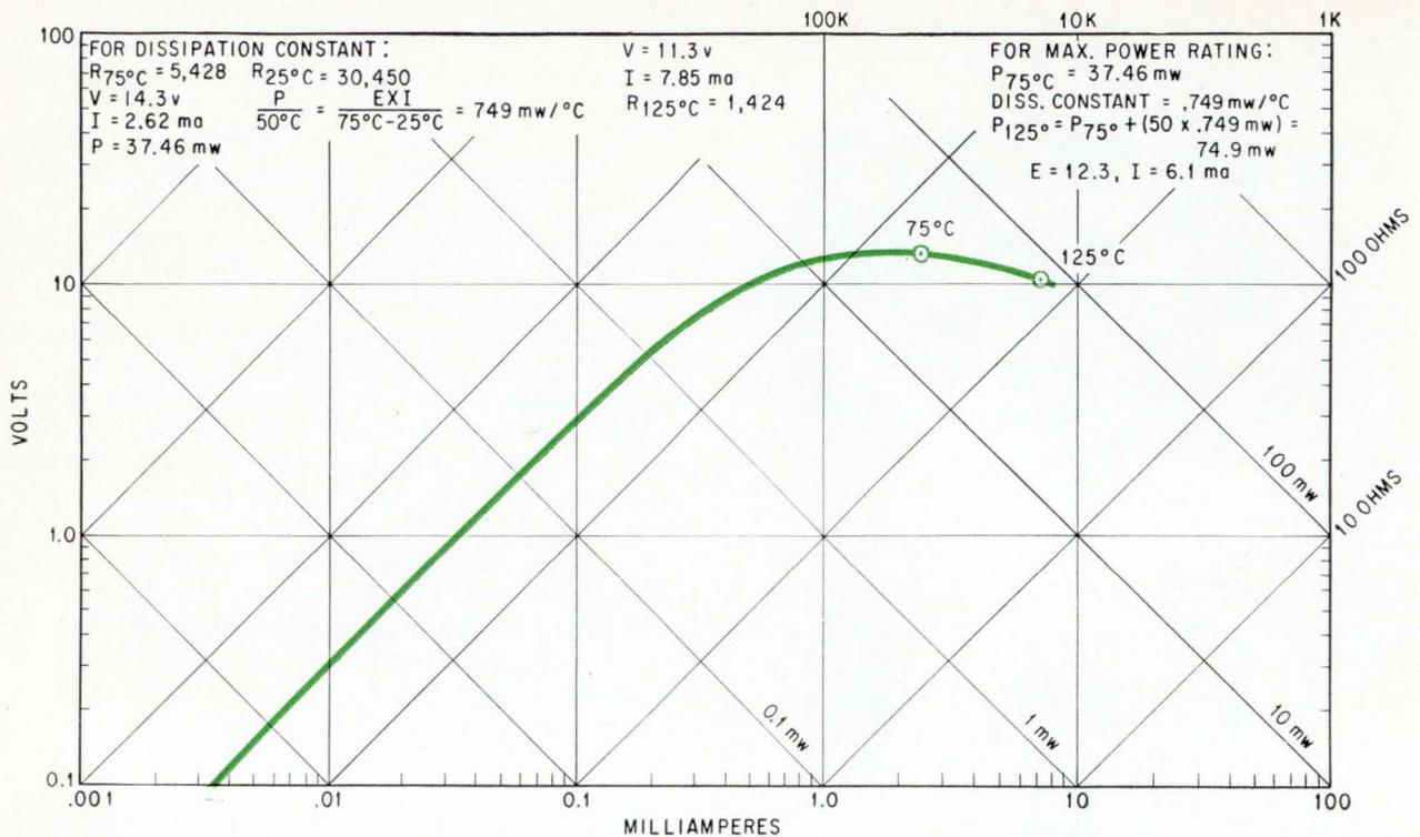
**Typical voltage current characteristic for a beryllium oxide substrate.**
