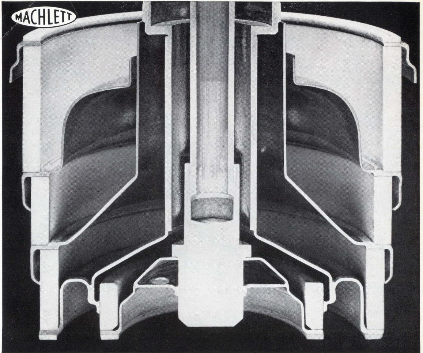
**Continuous cone electrode geometry: designed into all these tetrodes only by Machlett**
