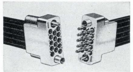
Designed for grounding radio-frequency interference, a line of molded plastic connectors assures good electrical contact with a double-finger construction. The contact is made possible by designing the locking springs as part of the subminiature coaxial connector. Thus, additional commoning springs and retaining plates are eliminated.
