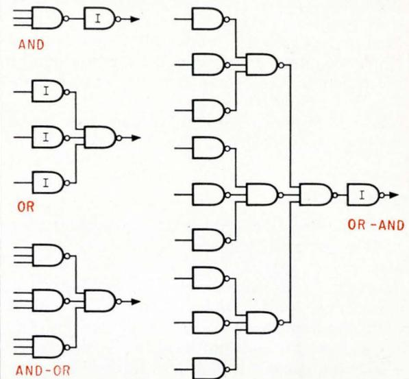
Using only NAND gates, such as in TTL circuitry, AND gate, OR gate, AND-OR, and OR-AND can be produced. For the AND, a NAND is followed by an inverter; in the OR, inverters precede a NAND; and AND-OR is made up entirely of NAND's; and the OR-AND is three stages of NAND's followed by an inverter.
