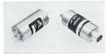
Preamplifiers with low noise and high input impedance are announced for use with hydrophones, accelerometers, infrared detectors, magnetometers, seismometers, biomedical sensors and other high-impedance transducers. Models 143 (20-db gain) and 144 (40-db gain) both come in four different package configurations.
