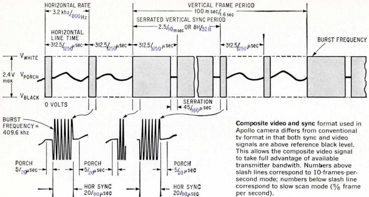
**Composite video and sync format used in Apollo camera differs from conventional tv format in that both sync and video signals are above reference black level. This allows the composite video signal to take full advantage of available transmitter bandwidth. Numbers above slash lines correspond to 10-frames-per-second mode; numbers below slash line correspond to slow scan mode (5/8 frame per second).**
