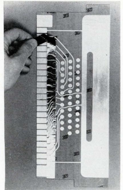
Plating tape is applied behind contacts to form one plating electrode.
