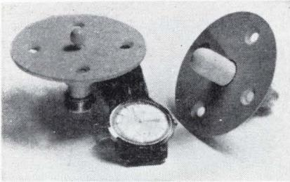
Beacon antennas—both stub and dipole—that operate from 8.5 to 9.6 Ghz are specifically designed for high performance aircraft.
