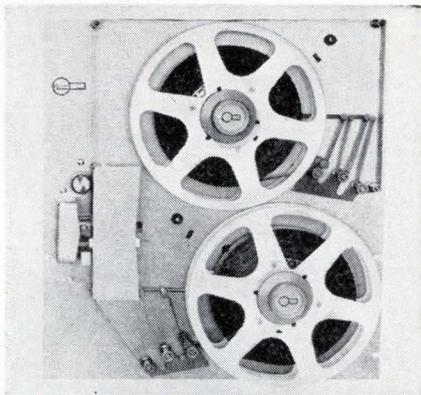
A compact, punched-tape reader and spooler reads 500 characters per second optically, and winds the tape on 10½-inch reels at 50 inches per second. The unit is only 21 inches high.
