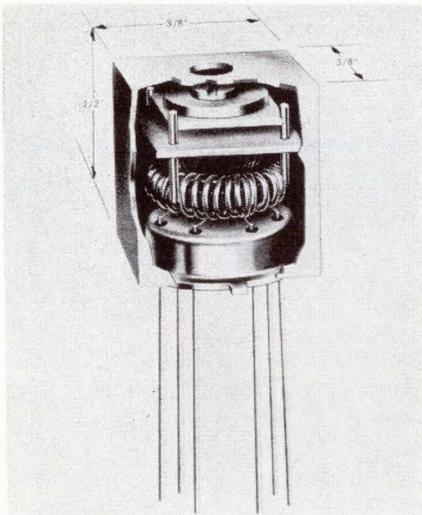
Typical of a line of miniature LC circuits is this phase detector packaged in a square can— $\frac{3}{8}$  in. square and  $\frac{1}{2}$  in. high—mounted on a standard 6-pin, TO-5 glass-to-metal-sealed header. A recent application has been in a monopulse radar system for weapons control, in which it detects the output phase difference between two 60-Mhz input signals emitted from an i-f amplifier.
