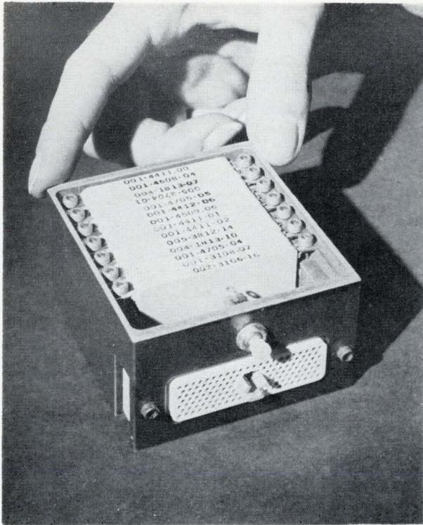
**Data-flow model** of a digital computer built from multicircuit monolithic chips attached to thin-film interconnection networks.
