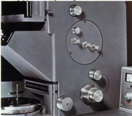
All features you want are built-in, at your fingertips. They can be used while you're comfortably seated. Conveniently reached control zone. Focusable stage.  $.5\times-3\times$  zooming variable magnification. Exclusive high-power stereo viewing. Visual observation, projection or photomicrography. Built-in shutter controls. Selector for transposable camera and viewing screen.
