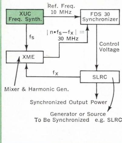
The Type XUC is the only true UHF-Synthesizer. It is the only single instrument to provide output frequencies to 1 GHz with 3V and 80 dB suppression of spurious. Generation of ultra-stable microwave frequencies is simplified and can be accomplished in two ways:
