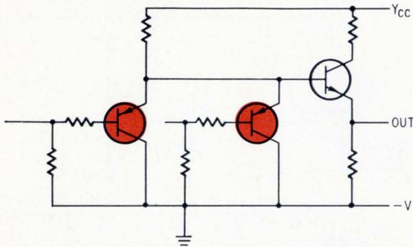
Complementary-transistor logic, CTL, needs current sink for low output level, current source for high-level output.
