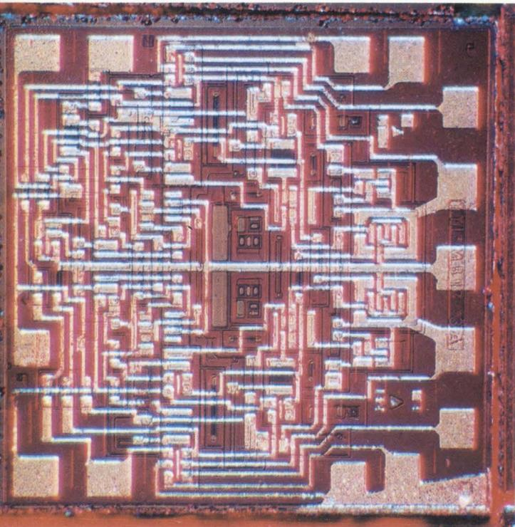
Rules of thumb in custom logic IC's like this one from Fairchild are: maximize functional circuits per unit area, minimize separate isolation areas, and use transistors in preference to passive elements.
