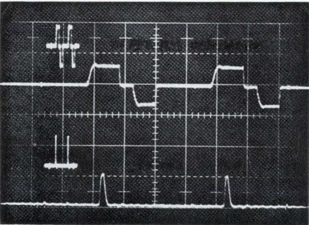
**Memory input and output** waveforms show the drive current on the top trace and the sense amplifier voltage on the bottom. The vertical scales are respectively 0.5 ampere per division and 3 volts per division; both horizontal scales are 1 microsecond per division.
