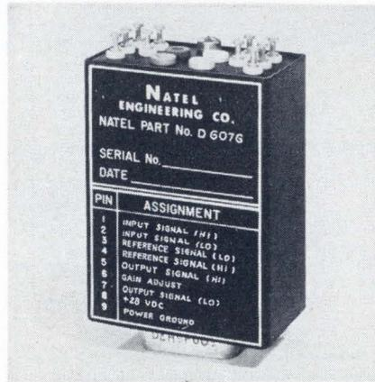
A miniature, solid state a-c amplifier-demodulator performs in extreme operational environments with the accuracy of laboratory-type instruments. It weighs less than 6 oz and occupies only 2.5 cu in. The unit operates either as an a-c to d-c converter or as a phase-sensitive synchronous detector for gyros, synchros, and linear variable differential transformers.
