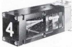
Illustrated: IEE Series 120 Readout — 160° circular viewing angle; character boundaries  $\frac{5}{8}$ " wide horizontal band drawn through .800" D circle. Brightness to 100 F. L.
