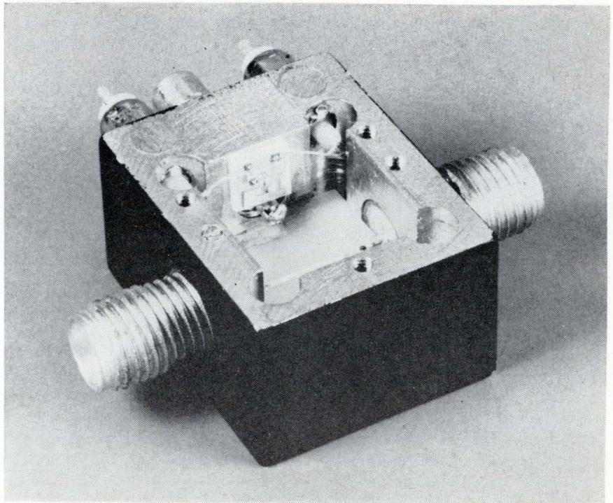
closeness to the diodes is shown by comparison tests. Using the internal driver, the switching speed is nominally 20 nanoseconds (in experimental models, the time has been halved). When the same switch was actuated by an external driver connected by a 10-inch coaxial lead, the best speed possible was 30 to 35 nsec.
