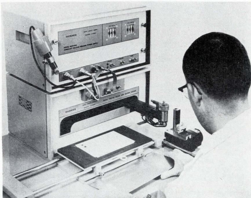
**Machines that automatically feed and place flatpacks on printed circuit boards haven't panned out, largely because girls with tweezers excel at gently handling the fragile IC packages.**
