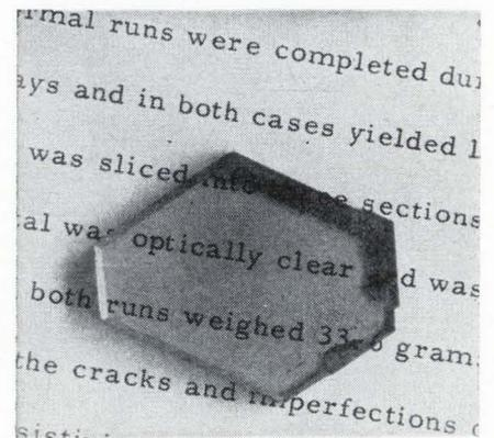
ductivity. Typically, the dopant is lithium. Resistivities of 1 ohm-cm to as high as  $6 \times 10^9$  ohm-cm have been obtained.
