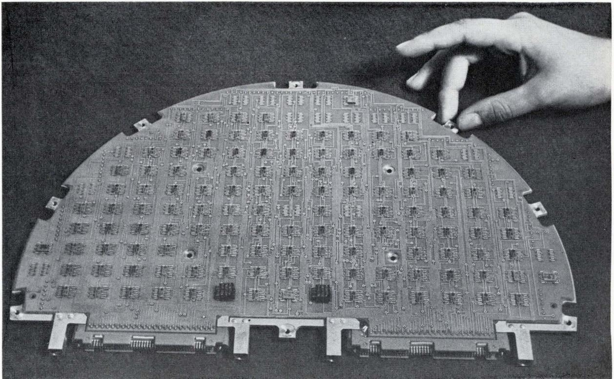
Flatpack mounting and wiring details are visible in this view of the arithmetic and control subassembly.
