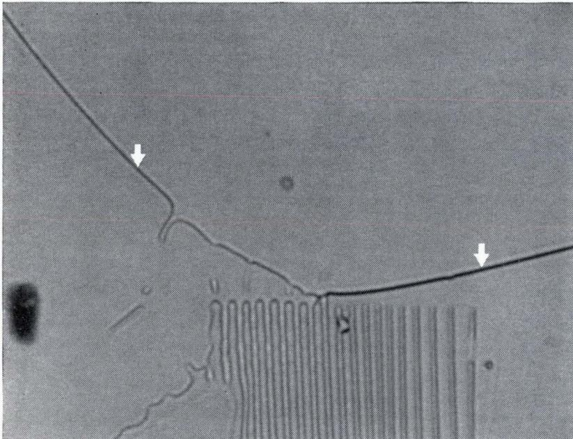
Bell Laboratories' model (200x) permits physical simulation of a eutectic phase diagram for an alloy such as lead-tin. Diagram relates liquid proportions (horizontal scale) to temperature (vertical).
