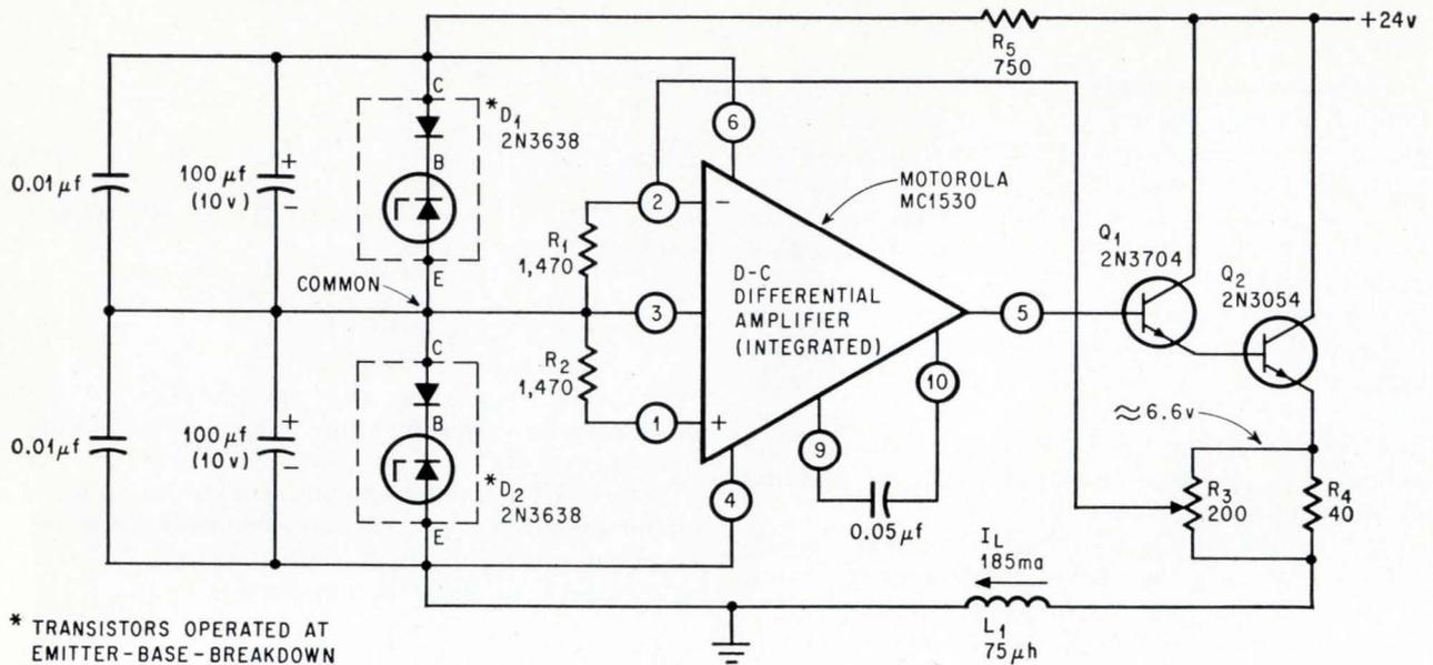
**Rising load current,  $I_L$ ,** raises the potential at pin 2 of the integrated amplifier. Pin 2 is the inverting input, so the higher voltage decreases the base current to transistors  $Q_1$  and  $Q_2$ , reducing  $I_L$ .
