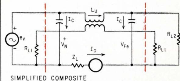
Equivalent circuit for a multiconductor system, top, accounts for common impedance, capacitive and inductive crosstalk. Next three diagrams show separate equivalent circuits for the three crosstalk sources, and the bottom circuit represents the simplified composite equivalent.
