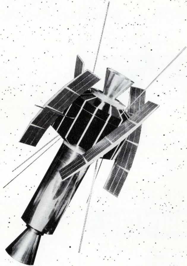
The Radio Astronomy Explorer (RAE) satellite is designed to give NASA an electronic map of the galaxy. Four reel-stored antennae of the RAE satellite consist of 2-in.-wide beryllium-copper strips over a tenth of a mile long. These antennae are made with furled metal strip produced by Hamilton Precision Metals, rolled to a thickness of  $0.002''$  and held to a tolerance of  $\pm 0.00015''$ .
