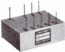
The micro magnetic squaring block and division module are assembled with semi-conductor operational amplifier for the solution of the indicated equation. Completely magnetic, solid state microblocks constitute the most reliable, space-saving analog voltage computing circuits available.
