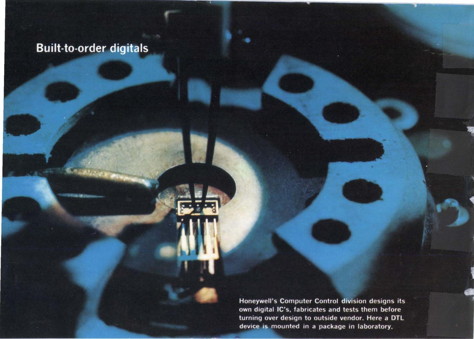
Honeywell's Computer Control division designs its own digital IC's, fabricates and tests them before turning over design to outside vendor. Here a DTL device is mounted in a package in laboratory.
