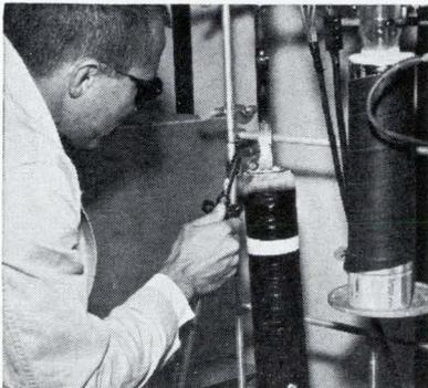
while one half inch away the same quartz tube is cooled by liquid nitrogen to -196°C. In half an inch, G-E fused quartz accepts a temperature gradient of 1994°C. Remember this fantastic capability of G-E quartz as you, in your own field, seek solutions to the uncommon challenge.
