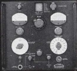
**Standard-Signal Generator** with a 9.5- to 500-MHz frequency range and 10-V, cw output behind  $50 \Omega$ ; or 5 V, modulated, behind  $50 \Omega$ . It has automatic output leveling *in all modes of operation* and true single-dial tuning (no trimmer adjustment needed). The generator frequency can be phase-locked to an external standard frequency. Modulation distortion is less than 3% at 80% AM. Type 1026-A Standard Signal Generator . . . \$6500.
