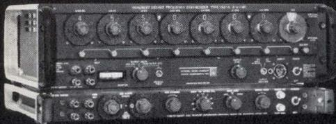
**Sweep and Marker Generator** for use with GR Synthesizers. It has nine sweep speeds, from 0.02 to 60 seconds, and sweep excursion is adjustable from  $\pm .001$  Hz to  $\pm 1$  MHz. Generates scope markers for quick calibration of the swept output. The synthesized center-frequency marker and side markers are accurate, stable, and precisely settable. Type 1160-P2 Sweep and Marker Generator . . . \$495.
