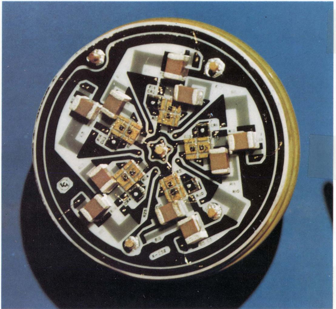
A divide-by-five ring counter has five current-mode switching stages, made in hybrid IC form by Electronic Communications Inc. for use in uhf digital communications system. The counter is used in pairs as a prescaler.
