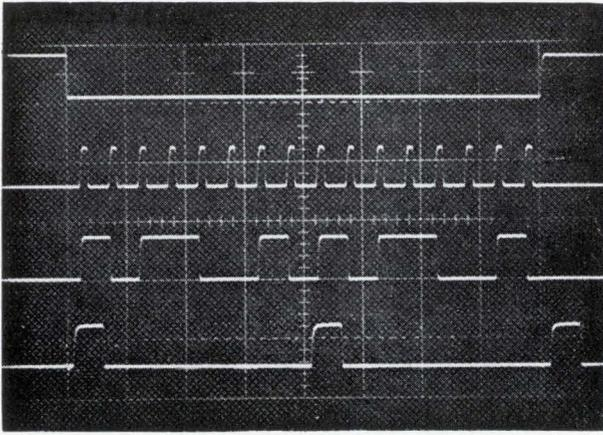
**Data and timing** waveforms from the computer are, from the top down, the instruction-execution cycle, the serial add shift operation, data from the accumulator, and the main computer timing pulse, once every 4 microseconds. The scales are 1  $\mu$ sec per division horizontally, and 5 volts per division vertically.
