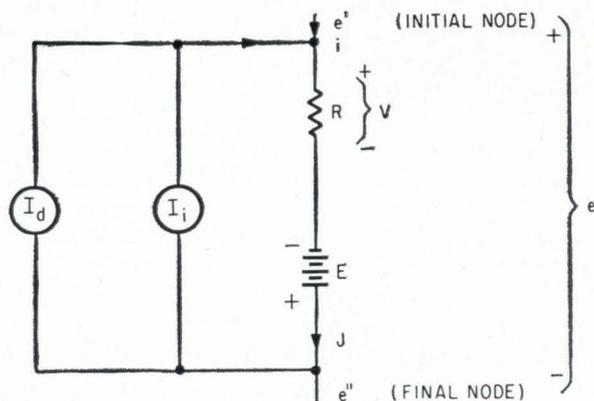
A circuit branch is defined from the initial node to the final node with each branch containing a nonzero R-parameter. The dependent current source is represented by  $I_d$  and  $I_i$  is the independent current source.
