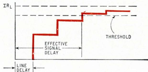
In nonmatched system, line reaches stable value after several reflections. Curve shows how effective delay of signal is greater than line delay alone.
