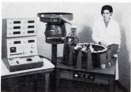
Testing and classifying diodes and rectifiers on production lines and at incoming inspection stations is done with a family of instruments. Designed for application with fast
