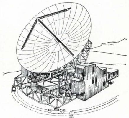
**British dish.** To tie into the Intelsat 3 satellite system, Goonhilly Downs ground station in Cornwall next year will have a new terminal with a 90-foot diameter stainless steel antenna.
