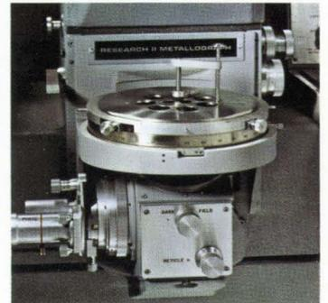
The exclusive Bausch & Lomb Foster Calcite Prism... your assurance of the finest results in polarized light... also provides vertical illumination for built-in bright field, sensitive tint, phase contrast and high power stereo viewing. A second prism produces an optimum level of dark field illumination.
