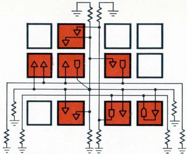
In this example of tree method, one gate is seen to drive both horizontal and vertical lines fanning out to flatpacks. All lines are terminated in characteristic impedance.
