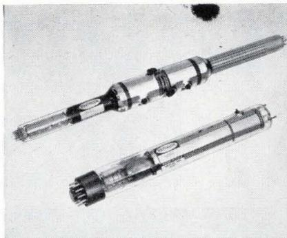
**Recording Storage Tubes.** The miniature tubes shown here are Raytheon's single-gun (CK1516) and dual-gun (CK1519). They provide high resolution, long storage, and fast erase capability.
