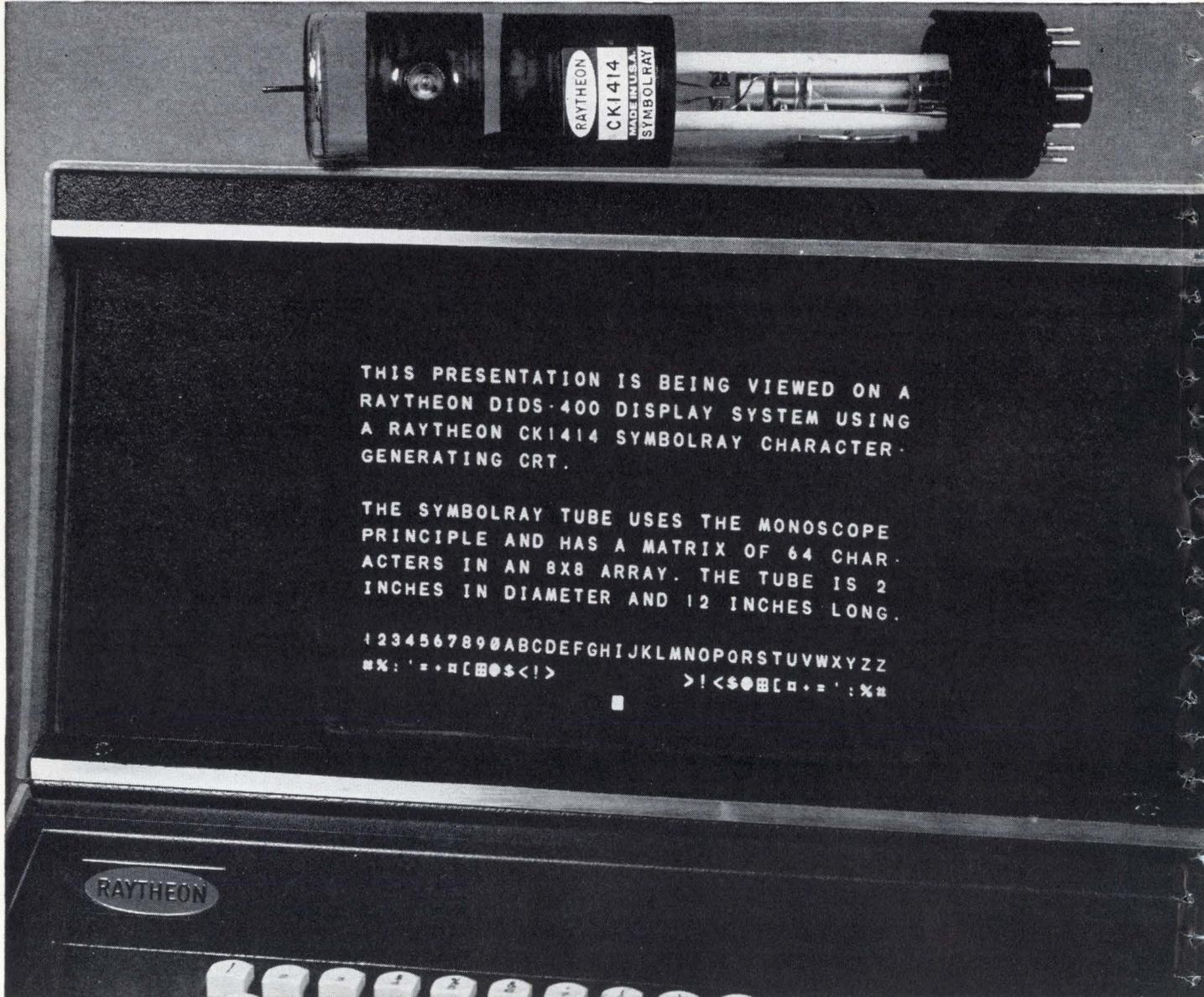
The presentation you see above was generated by a Symbolray\* Cathode Ray Tube identical to the one lying on the console. A new type of monoscope, the Symbolray can generate alphanumeric characters from electrical signals for cathode-ray display or for hard copy print-out. The presentation here is shown on a Raytheon tube (CK1415) used in a Raytheon DIDS-400 display system.
