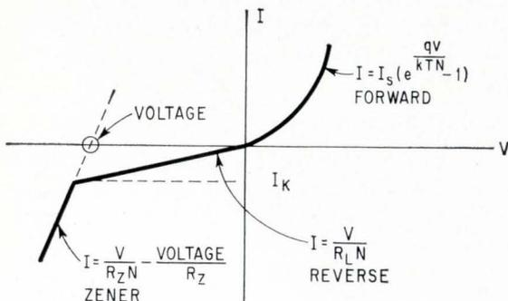
Typical characteristic current versus voltage curve for a zener diode. Plot is broken into three parts with each part represented by an appropriate current-voltage equation.
