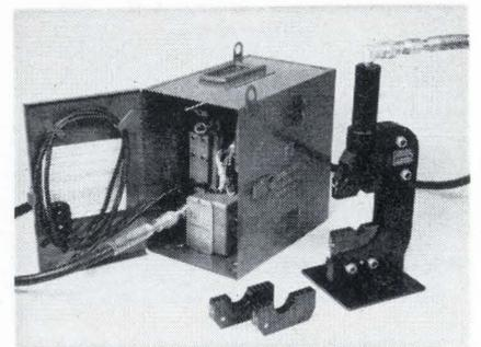
Both the inner and outer shields of multiconductor shielded cable are terminated by a new lightweight crimping tool. The Y40LH Hypress
