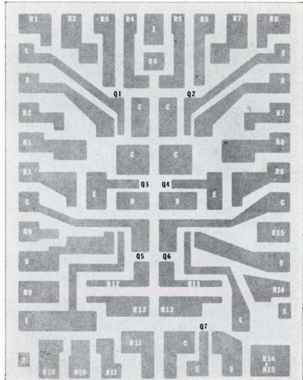
**Master dice breadboard** has six transistors and 33 resistors varying in value from 75 ohms to 10,000 ohms. Aluminum bonding pads shown in photo at right are connected to each resistor and to the emitter, base, and collector of each transistor.
