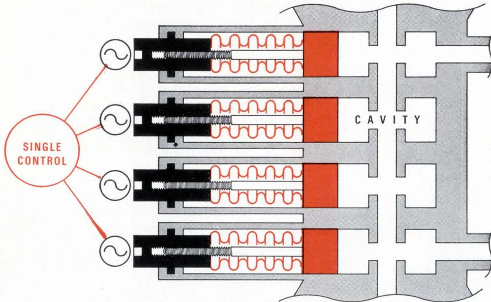
The secret of remarkable tunability for communication klystrons is Sperry's exclusive bellows-type tuner. Replacing the old-fashioned, short-life diaphragm, the bellows gives you longer tuner life and greater tuning accuracy. The bellows tuner, combined with remarkable tracking of the tube cavities, makes remote push-button or gang-mechanical tuning a reality.
