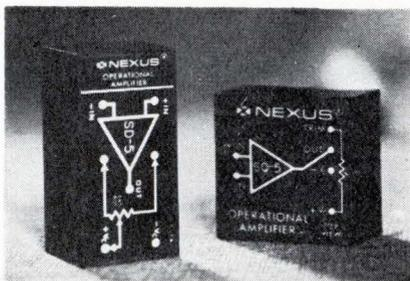
pedance, 20 megohms; differential input impedance, 200 kilohms. The unit measures 1.55 in. long, 0.78 in. wide and 0.60 in. high.
