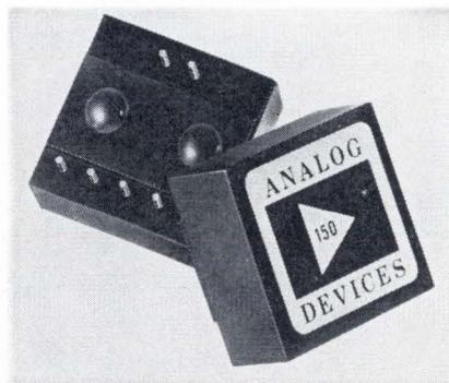
Operation for 1,000 hours from a pair of standard mercury cells, in addition to small size and low cost, is offered by a d-c differential operation amplifier. The unit measures 1 1/8 in. square by 3/5 in. high. It costs \$30; batteries are \$1 each.
