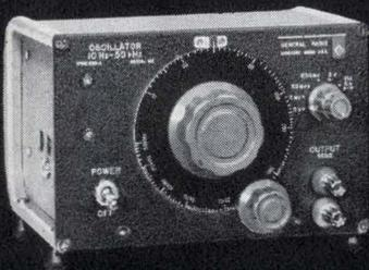
**General-Purpose Laboratory Oscillator** with its full 10-Hz to 50-kHz range covered by one turn of the dial. No range switch to wear out! This also means no range-switching transients and no ambiguous dial multipliers. Generates both sine and square waves, and can be synchronized to an external signal or can supply a sync signal. Has a calibrated 60-dB step attenuator and a 20-dB continuously adjustable attenuator. Type 1313-A Oscillator . . . \$325.
