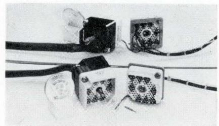
In the same mounting area normally required by a size 18 MS shell, a new connector will provide 100 removable contacts and six polarization positions. Because of their square design, ten of these connectors can be mounted in a space required for six round ones.
