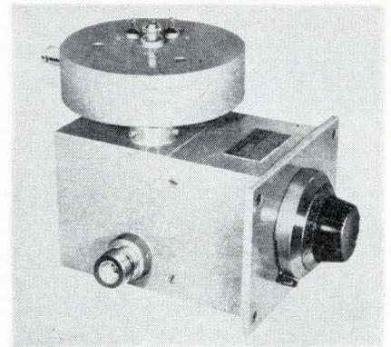
Designed for telemetry and general receiver applications, an integrated package contains a preselector, balanced mixer, and an adder network. It can also monitor individual crystal current.
