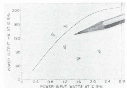
When used as a high-order multiplier at microwave frequencies—X-band and above—a new step-
