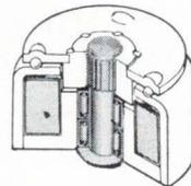
**Packaged Control Solutions** Here we put our disc-shaped solenoid to work as a driver for a miniaturized (4 $\frac{3}{16}$  x 1 $\frac{3}{32}$  x 1 $\frac{1}{32}$ ) 12-position stepping switch. Model shown is an armament control (intervalometer). It is used to fire 19 rockets in pairs sequentially, at 10 ms intervals. We can tailor one like it for your stepping or sequentially timed switch application.
