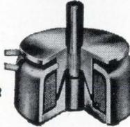
**Ledex Bi-Directional Solenoid** Energizing either coil causes shaft to move to right or left of center detent ("off") position. Shaft is spring-loaded... returns to center position when coil is de-energized. Outputs up to 350 pounds.
