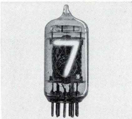
**Datavue\* Side-View Tubes.** New Type CK8650, with numerals close to the front, permits wide-angle viewing. These side-view, in-line visual readout tubes display single numerals 0 through 9 or preselected symbols such as + and - signs. Their 5/8"-high characters are easily read from a distance of 30 feet. Less than \$5 each in 500 lots, they also cost less to use because the bezel and filter assembly can be eliminated and because their mating sockets are inexpensive.
