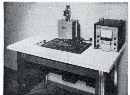
Joining flatpacks to p-c boards becomes a quick and easy operation with a semiautomatic solder reflow machine. It is designed for medium
