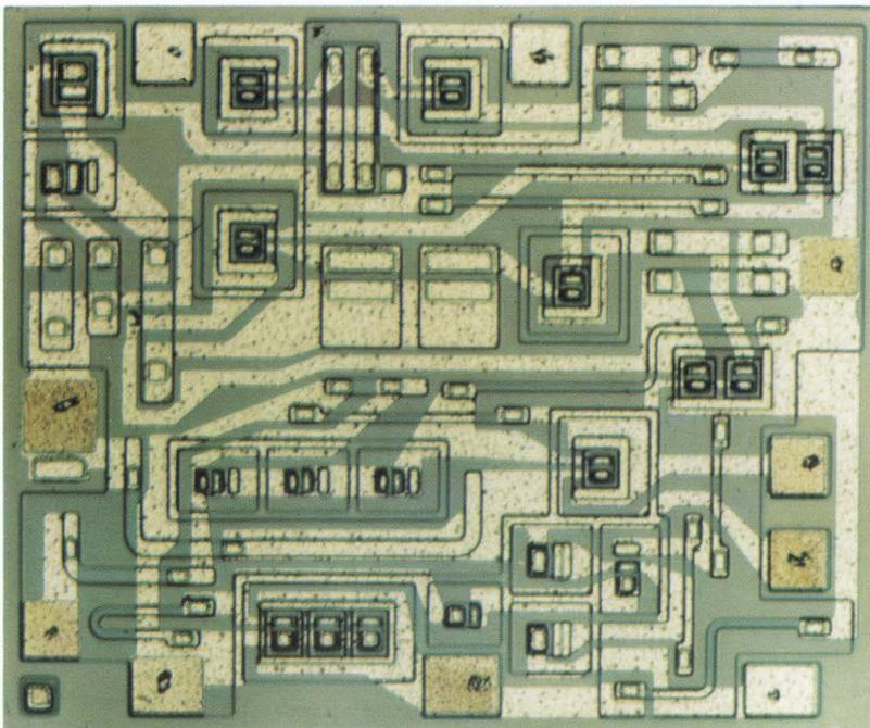
Modified-DTL, in which input diodes are replaced by transistors, forms the output of this monolithic sense amplifier. Built by Motorola Semiconductor for 0.5  $\mu$ sec-cycle core memories, its high and low output levels are 5.9 volts and 0.35 volts, respectively.
