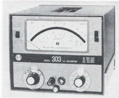
An analog meter capable of measuring a-c voltages from 2 hertz to 6 megahertz will be introduced at the IEEE show by Ballantine Laboratories Inc. The company's president, A.W. Parkes Jr. reports it is the first transistorized analog instrument capable of operating at such a low frequency.
