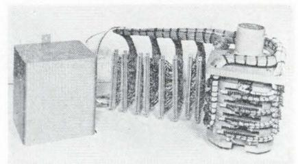
Data sampling and data logging in process control are two applications for a new rotary scanner switch. The high reliability switch is basically a sequential sampling device for feeding a large number of signal inputs into one channel,
