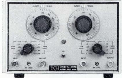
MODEL 3202 provides continuously adjustable high-pass, low-pass, bandpass and band-reject functions over frequency range of 20 Hz to 2 MHz. Two-channel bench unit shown; 5 1/4" x 8 5/8" x 1 1/4"-rack units available.
