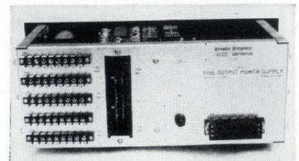
Five voltages from +20 to -20 volts d-c at currents from 1 to 7 amps are produced by the model 11578 power supply. The unit can be adapted to specific system requirements.
