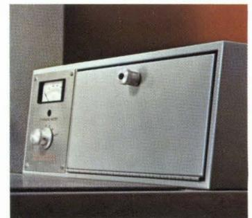
An integral exposure meter removes guesswork—lets you turn every film into a properly exposed photomicrograph with optimum contrast, high resolution. Within arm's reach is the built-in desiccator cabinet—a moisture-free area for safe storage of normal size and most frequently used specimens.
