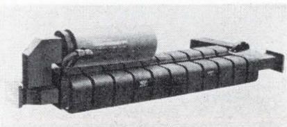
High peak and average power capability are features of a 4-port, liquid-cooled circulator. Model 336180 can handle 20 Mw of peak power and 20 kw of average power while maintaining a low insertion loss of 0.5 db maximum.
