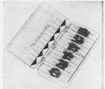
A "Zener Lab" has been introduced for use in accurately determining the zener tolerance of a circuit. It consists of a kit of 80 one-half-watt zener diodes, supplied in increments of 0.1 v throughout the range of 2.0 to 10.0 v. Each zener is graded to  $\pm 0.05$  v. tolerance at each voltage, which is stamped on the zener body.
