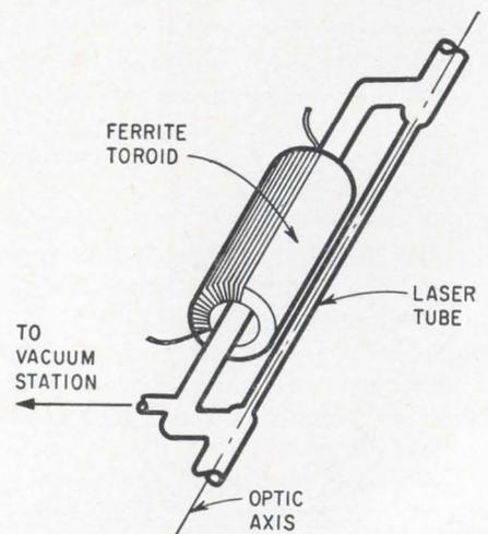
**Design of an experimental laser system** developed by William E. Bell of Spectra-Physics. A ferrite toroid, wrapped around the ion gas laser tube, induces an alternating voltage in the tube, causing laser action.
