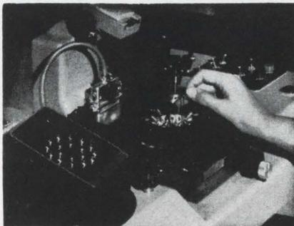
Testing integrated circuits and transistors in wafer form is accomplished by needle-like probes. These probes must contact the wafer's pads simultaneously; that is, they must be coplanar. Also, they have to contact at just the right angle, at the proper pressure, and have to scrape off the oxide
