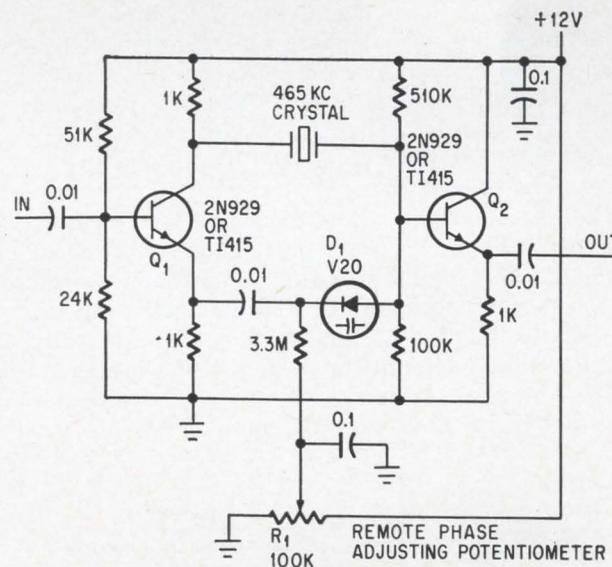
Phase inverter  $Q_1$ , substituted for the i-f transformer allows remote phasing by adjusting the potentiometer,  $R_1$ , which controls the bias on varactor,  $D_1$ . The circuit can be used over a wide frequency range.
