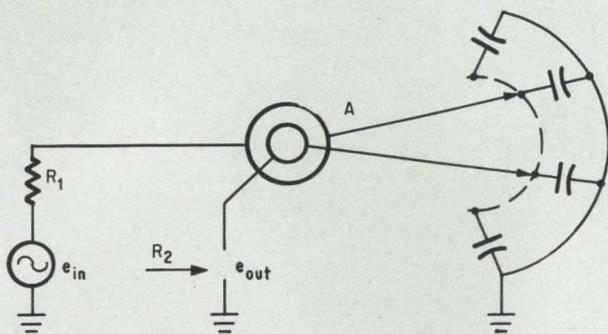
**Mechanical analog** of a comb filter. Here the mechanical rotational frequency of the switch fixes the location of the passbands, and the time constant ( $R_2$  times the capacitor being touched by the brush) fixes the width of each band.
