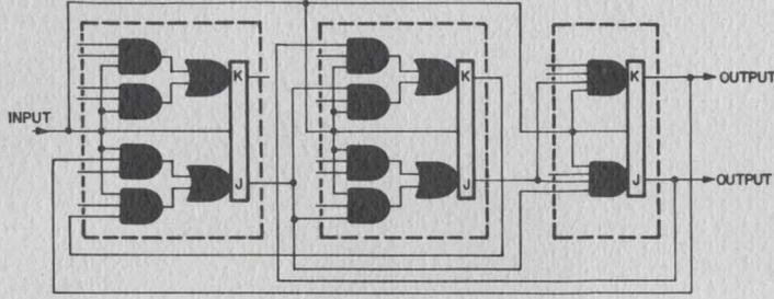
A simplified but effective method of performing divide-by-seven operations is described in the logic diagram shown above.
