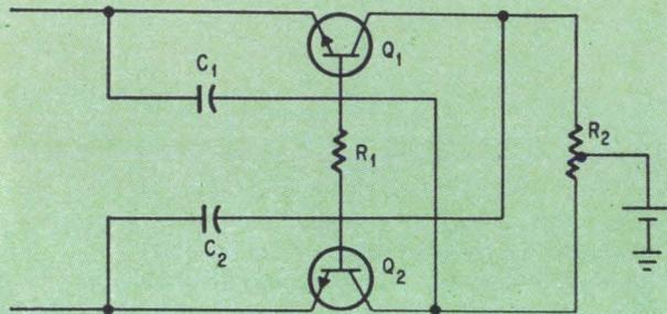
**Basic negative-impedance converter circuit. Common base connections assure equal input and output current. Cross-coupling inputs to the outputs fulfills the second requirement: equal input and output voltages.**
