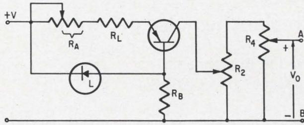
**Constant-current** to drive the potentiometers is provided by a common-base transistor amplifier.
