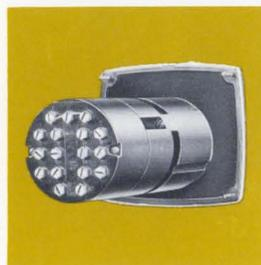
A space-saving control module eliminates the mounting and wiring of separate components . . . speeds up and simplifies installation. The control module simply plugs into the rear of the indicator and may be removed without interrupting the measurement circuit.
