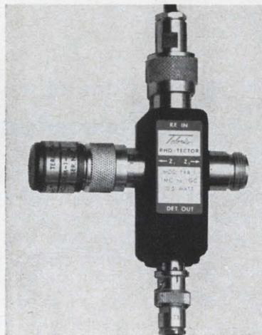
symmetrical bridge that determines VSWR by balancing the unknown against a known impedance. The output may be displayed directly on an oscilloscope or X-Y recorder.
