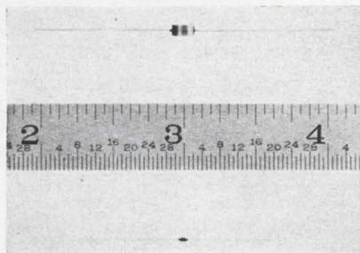
Magnetically pure silicon diodes are designed for space environments requiring low-density residual magnetism leads for magneto-
