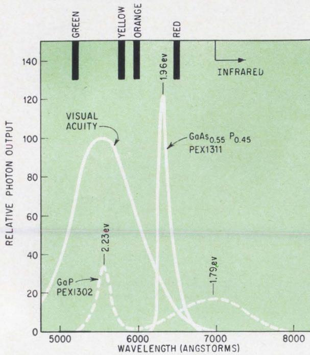
**Spectral output curves** for visual-light emitters compared with eye-response curve. The gallium-phosphide source has two peak emission points, at 5,600 angstroms and at 7,000 angstroms for the PEX1302. By adjusting the doping concentration in the region of the junction, the amplitude of the peaks can be changed.
