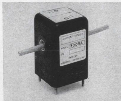
A line of solid-state, highly accurate current sensors utilize magnetic-flux-sensitive resistors in a magnetic-flux-balance circuit. The sensors measure d-c current in ranges from 0 to 1 ma to 0 to 100 amps and develop 0 to 5 v output.
