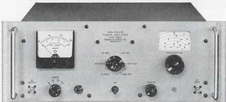
The BRC Power Amplifier Type 230-A is the ideal RF amplifier for low-level applications exhibiting a typical noise figure of 6 to 8 db. Three tuned, cascaded stages of grounded-grid amplification provide up to 30 db gain and a maximum power output of 5 watts. Typical applications include:
