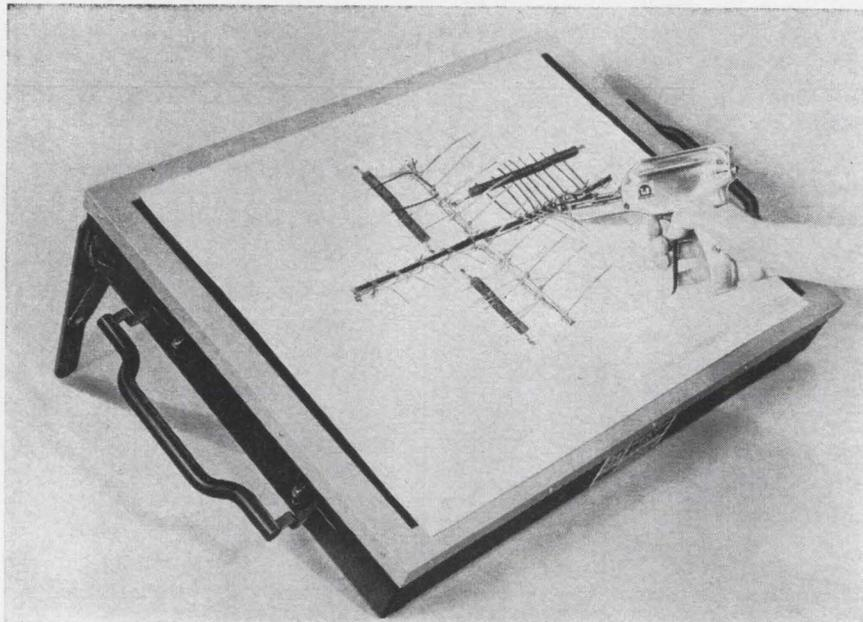
Wire-harnessing boards with reusable, retractable wire-routing pins are two ways better than the homemade harness boards that have been used for decades to pre-fabricate wiring assemblies, says the Thomas & Betts Co. The problems of board storage are avoided, and the pins don't interfere with harness tying and removal from the board.
