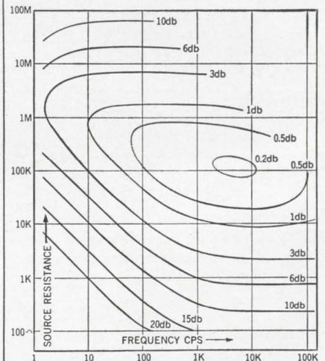
Contours of constant noise figure for a typical PAR Type A preamplifier plotted to show dependence on frequency and source resistance at 300° K. Amplifier operated single-ended.
