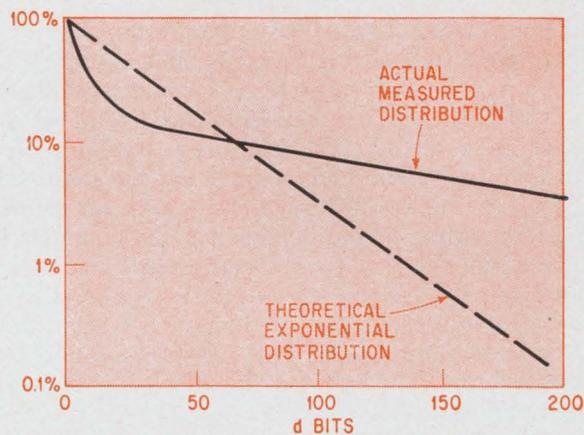
**Statistical distribution of intervals between errors.** The theoretical curve is based on the assumption that errors occur randomly and that the probability of error is constant. But this isn't the case when data is measured on an actual channel. The curve plotted from the measured data shows that there is a higher probability that another error will occur within 30 bits of the previous error.
