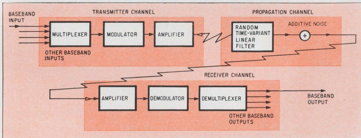
**Transmission channel.** For error control the digital communications channel is considered as including parts of the transmitter and receiver, and the propagation medium itself. Errors can occur in the transmitter or receiver channel because of the equipment. In the propagation channel, errors can occur because the behavior of the medium isn't constant, or because the signals become affected by the noise in the medium
