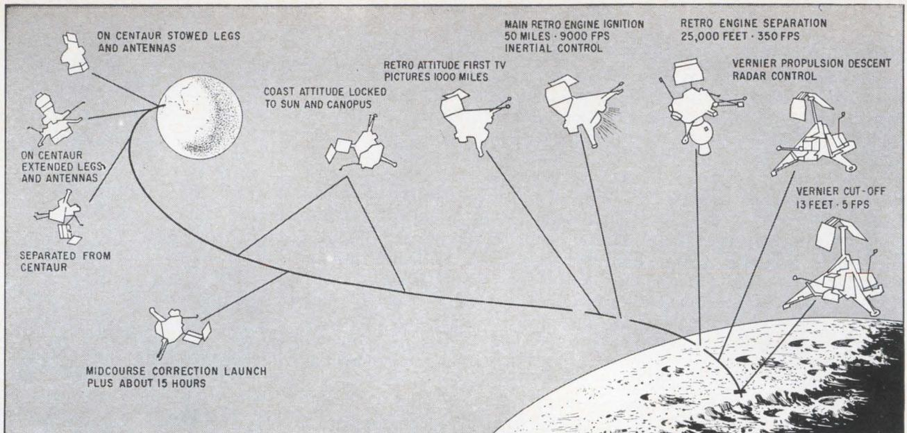
The surveyor spacecraft, about 15 hours after blast-off, gets a course correction from the California ground station, which also commands Surveyor to turn its legs toward the moon for landing, and instructs it to lock on the sun and the star Canopus for guidance. Sixty-six hours after launch, an elaborate system consisting of a retro-rocket, vernier engines and radars—still not working well, according to the subcommittee's report—is supposed to ease the bus down on the moon.
