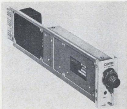
Model 3400 is a wideband amplifier for driving medium-power recorders, passive filters and display devices. One of the company's direct-coupled differential amplifiers in the 3000 series, it has a full-scale load current of 10 ma. The full-scale output voltage is  $\pm 10$  v, and the small-signal bandwidth is a minimum of 50 kc. The unit offers a totally isolated power supply, also modular dimensions that allow 10 model 3400's to fit into one model 3010 rack enclosure.
