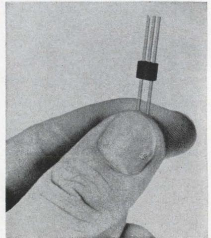
A solid-state silicon microminiature chopper is said to be the smallest ever devised. Model 6 Microchopper will connect and disconnect a load from a signal source, and may also be used as a synchronous demodulator to convert an a-c signal to d-c. Linear switching or chopping of voltages can be accomplished over a wide dynamic range from  $\pm 20 \mu\text{v}$  to  $\pm 5 \text{ v}$ . Model 6 is an inertialess device that can be driven from d-c to 100 kc.
