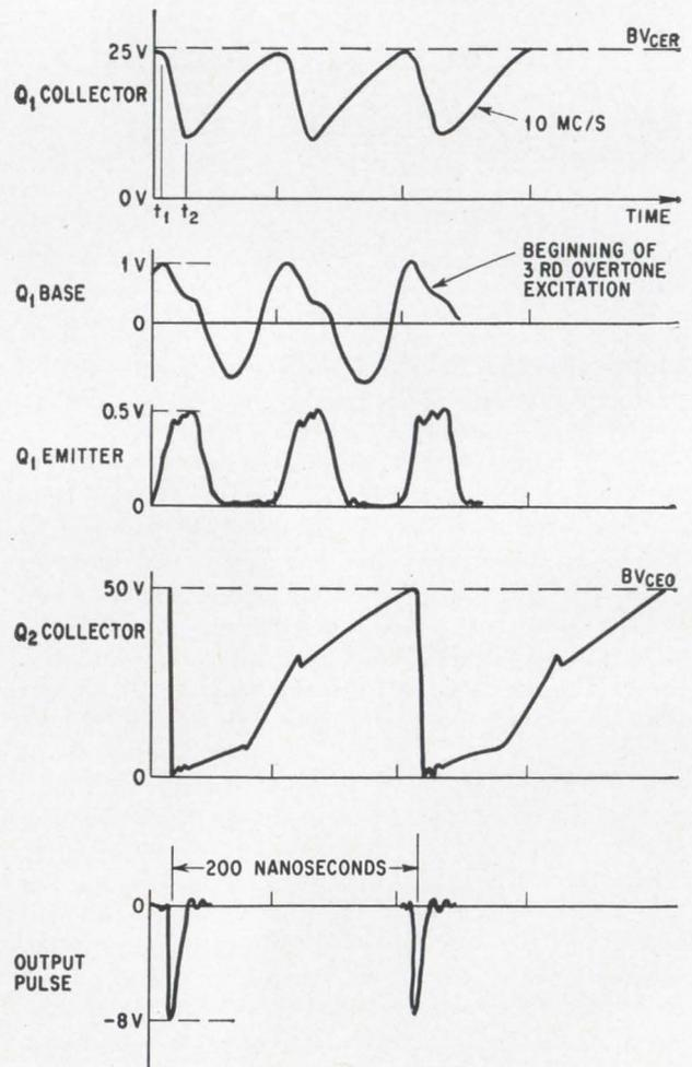
Output pulses occur during the interval  $t_1$  and  $t_2$  when  $Q_1$  is forced into heavy conduction. Frequency division at the output is controlled by the time constant  $R_5 C_2$ .
