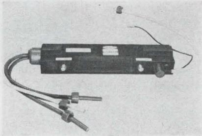
A broadband traveling-wave tube has been announced that delivers peak pulse power of more than 1 kv at a 2% duty cycle. The QKW-1366 covers both C and X bands in a single tube with a frequency range of 5 to 12 Gc. Gain is 34 to 40 db.
