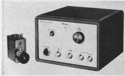
A uhf, solid-state sweep generator, model CS-77, has been introduced for testing and aligning uhf-tv tuners. It permits the user to sweep the entire uhf band in a single sweep, with pulse markers appearing at each end of the band. The unit provides a system for rapid check of tuner gain over the entire uhf band, and detailed bandpass checks at each end, without making adjustments to the sweep generator.
