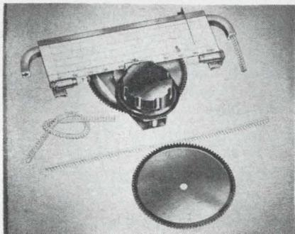
Model 10037 is a sturdy dial assembly that completely eliminates the annoyance of string-driven pointers, eliminates all indicator stutter or wobble and provides positive pointer travel and resetability. The pointer is driven positively by a flexible but nonelastic molded gear-driven rack which cannot slip, break or fall off a pulley. The geared flexible rack rides in a multi-slot extruded aluminum channel.
