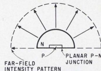
**Geometries** used to construct gallium arsenide light sources. At left is the etched flat geometry used for the TIXLO2. The planar geometry shown in the center is used in building the TIXLO1 and PEX1004. The hemispherical geometry of the TIXLO3 is at right. The dotted lines show the light-intensity patterns before packaging of the wafers.
