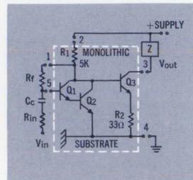
4JPA113 silicon monolithic circuit (TO-5 configuration, 5 leads)
