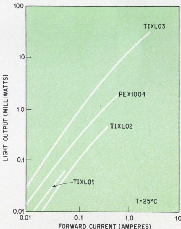
**Output power curves** for typical gallium-arsenide light sources. Power capability is determined by the device's internal geometry and by the package used.
