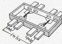
Sprague leads again with two dual-emitter chopper transistors in one flat-pack case, with tight  $V_{OFF}$  matching of both devices.
