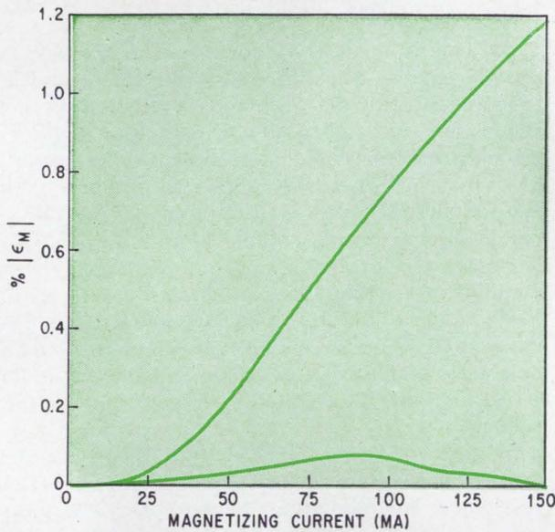
**Magnetic component of tracking error as a function of magnetizing current before and after (lower line) its partial compensation by means of a 0.112 megohm resistor shunted across  $r_2$ .**
