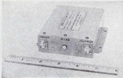
A light-weight, X-band tunnel-diode amplifier now on the market requires no temperature-controlling heaters. Model D65X3 typically has  $20 \pm 2$  db gain from 8.3 to 9.7 Gc over a temperature range of  $-10^\circ$  to  $+60^\circ\text{C}$ . The noise figure under these conditions is 6.0 db maximum. Bias power requirements are 10 mw maximum at 1.25 volts from external source. An internal battery can be provided if desired. Other frequency ranges are available.
