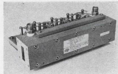
Precise, incremental phase-shift values can be switched into or out of a signal path at high speed by the model D14H1 digital phase shifter. Four phase shift increments of 180°, 90°, 45°, and 22.5° can be switched either singly or in any combination at average switching rates up to 5 kc.
