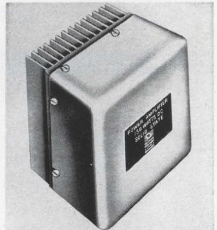
A line of modular d-c servo amplifiers is available in 50-, 150-, and 350-watt sizes. All are completely transistorized. Essentially, these operational power amplifiers, along with d-c direct-drive torque motors, provide a complete servo system. Gain is adjustable from a value of less than unity to  $5 \times 10^5$  v/v, which eliminates the need for a preamplifier.
