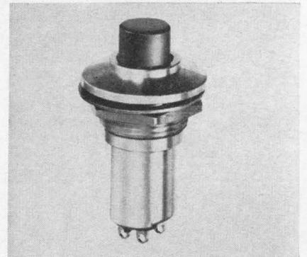
A dpdt push-push design switch features the use of internal bonding and grounding to eliminate mechanical discontinuities that could serve as points of rfi emission. All switches meet radiation requirements for use in airborne electronic equipment designed to MIL-I-26600 specifications.
