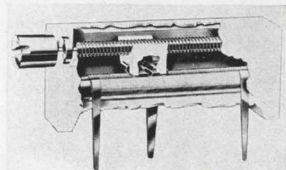
A series of microminiature trimming potentiometers now available use a new production process called Weld-Fast to fasten the tiny trimmer lids permanently to the cases.
