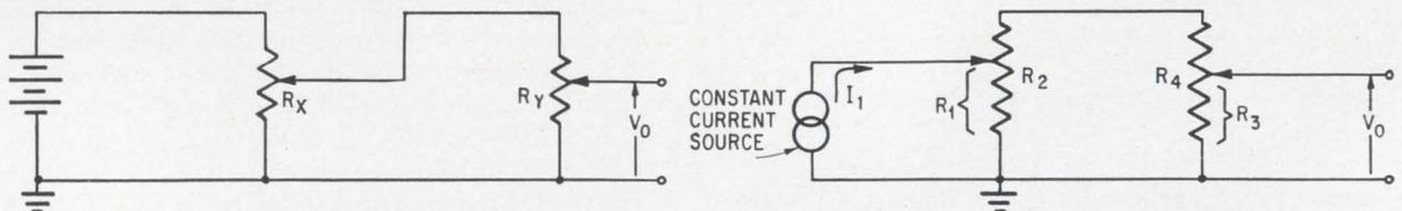
**Conventional cascaded** potentiometer on the left has an output which is approximately proportional to the product of the shaft rotations. The improved circuit on the right has an output which is exactly proportional to the product.
