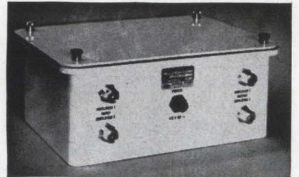
Transistor amplifiers now available feature extremely low noise figures in the uhf and vhf ranges. Typical of the new line is the model TQN-2251-2 dual-transistor amplifier assembly. It operates over a range of 225 to 235 Mc with a gain of 25 db and a maximum noise figure of 2 db.
