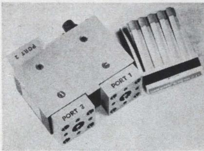
A line of circulators designed to operate at liquid-nitrogen or liquid-helium temperatures is offered for use with ultra-low-noise parametric amplifiers. By cooling the circulator, the noise contribution of its input losses is significantly reduced, and degrading long-line effects caused by diode-circulator separation are eliminated.
