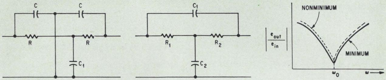
Two typical notch-filter RC circuits are the parallel-T at left and the bridged-T, center. The attenuation vs frequency relationships for minimum and nonminimum phase-shift networks are similar, as shown at right.
