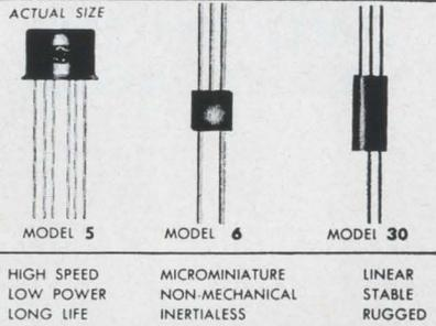
The transistor chopper (or modulator) is a solidly encapsulated unit designed to alternately connect and disconnect a load from a signal source. It may also be used as a demodulator to convert an a.c. signal to d.c. It is capable of linearly switching or chopping voltages over a wide dynamic range which extends down to a fraction of a millivolt and up to 150 volts.
