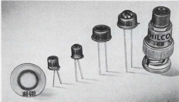
**speed up your system**—offering response times typically less than  $1\mu\text{sec}$  (custom devices with RC cutoff frequencies beyond 5 Gc)—compared with the millisecond range of typical PbS detectors.
