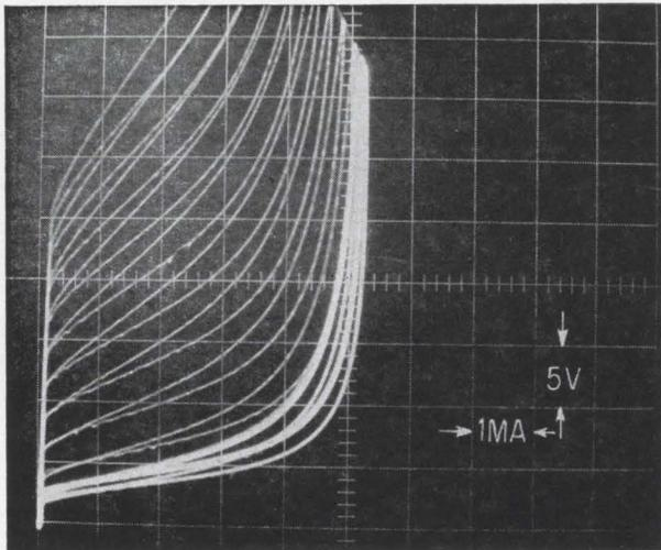
The characteristics of an expensive, high-quality silicon transistor can be simulated by a three-terminal circuit containing a high-gain germanium transistor using local feedback. These characteristics are collector curves that are nearly flat out to the breakdown voltage; low leakage; and adjustable current gain over a wide range of temperatures, current levels and collector voltages.
