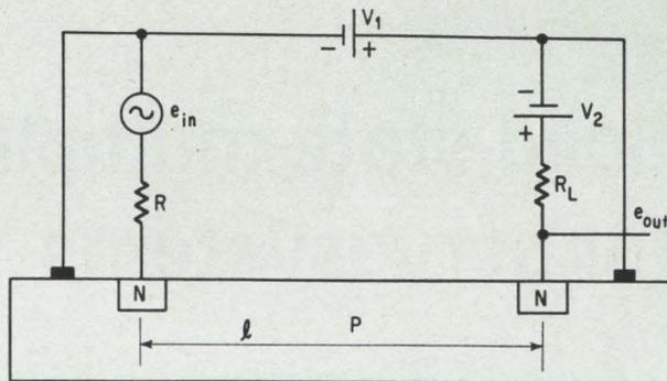
**Semiconductor delay line.** The time delay is a function of the distance between n-type silicon regions. The stability criterion of a circuit using a semiconductor delay line is similar to that of a network using an RC feedback circuit such as a notch filter.
