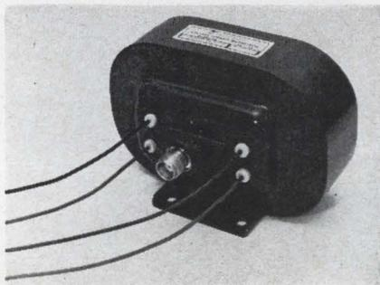
A high-efficiency, high-power, voltage-tunable magnetron can be electronically tuned over the 3- to 3.5-Gc frequency range at 100 watts minimum power with an electronic efficiency of 70%.
