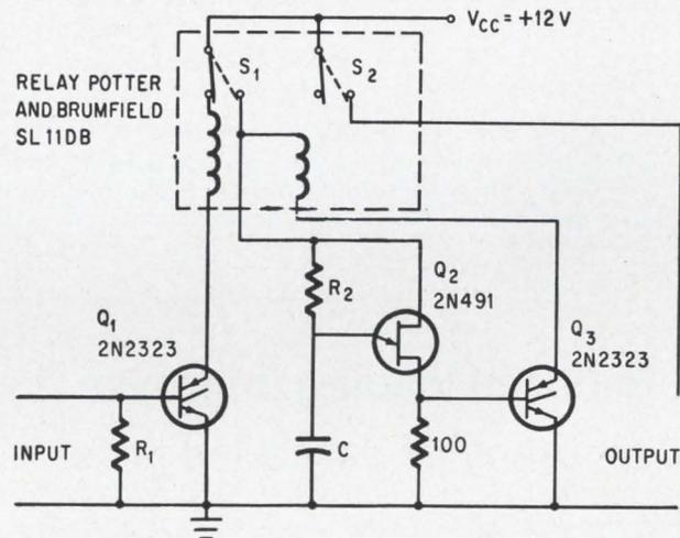
**Unijunction transistor circuit determines output pulse length.** Latching relay is turned on by input pulse, remains on until ujt reaches its peak point voltage.
