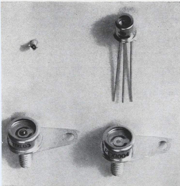
**Typical gallium-arsenide light sources.** The miniature TIXLO1 (top left) permits high mounting densities. The medium-power TIXLO2 (top right) comes in a package similar to the Jedec TO-18 case. Two bottom units, are the TIXLO3 (left) and the PEX1004.
