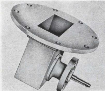
A high-power S-band transition section for a WR-284 waveguide flange to 7/8 in. coaxial handles 600 watts average with a peak of 25 kw. Frequency range is from 3.1 to 3.5 Gc; vswr is less than 1.2 to 1. Specialty Automatic Waveguide Corp., 12 Wilmington Road, Burlington, Mass. [425]
