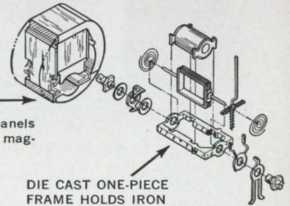
DIE CAST ONE-PIECE FRAME HOLDS IRON CORE IN EXACT ALIGNMENT
