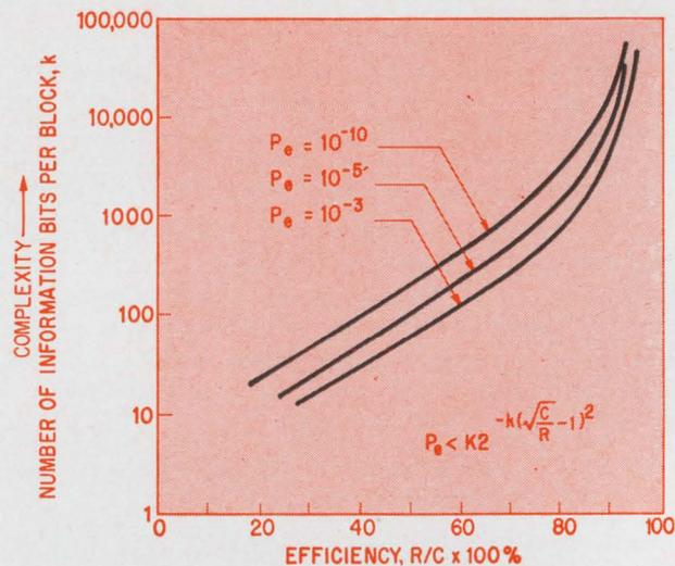
**Decoder complexity** can be expressed as a function of channel efficiency. To approach 100% efficiency for a fixed error rate,  $P_e$  would require an extremely large number of information bits in each block of the code, and a complex decoder.
