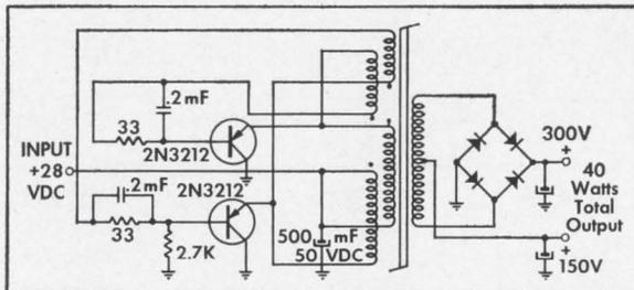
40-watt DC to DC converter gets an efficiency of 90 percent from the low saturation resistance of the miniature Delco 2N3212.
