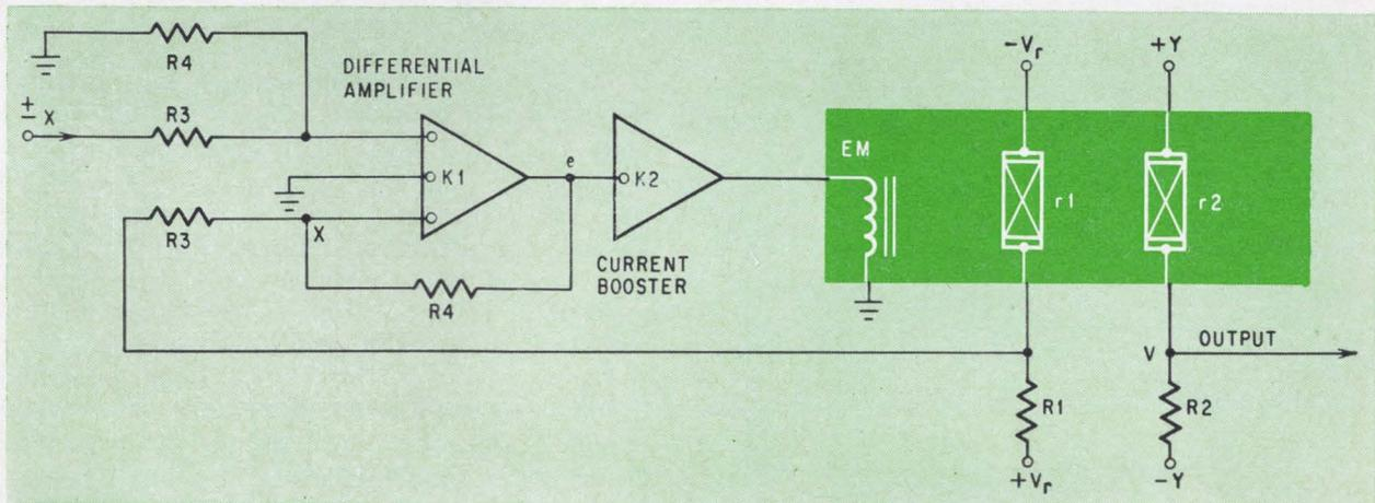
Magnetoresistive analog multiplier: Magnetoresistors  $r_1$  and  $r_2$  are in the gap of electromagnet EM. Resistors  $R_1$  and  $R_2$  are adjusted to match respectively  $r_1$  and  $r_2$ ;  $R_1 = 1000$  ohms and  $R_2 = 1$  megohm.  $V_r$  is a fixed reference potential.  $X$  and  $Y$  are variable input voltages whose product appears as the output voltage  $v$ .
