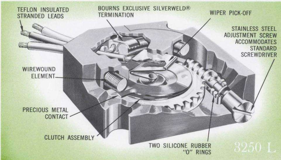
BOURNS WORM GEAR ACTUATED POTENTIOMETERS, in the popular square configuration, were developed to add packaging versatility yet assure the same high performance and reliability as the TRIMPOT Leadscrew Actuated Potentiometer line. These units, in 1/2" and 3/8" sizes, available with stranded insulated leads or printed circuit pins, feature all-sealed construction, excellent resolution, and an exclusive clutch-action wiper which prevents damage from forced adjustment.
