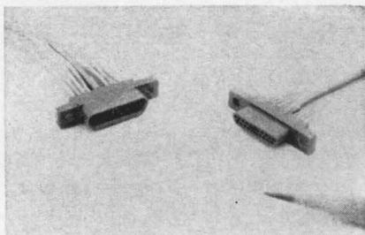
The Micro-D, a microminiature connector with coaxial contacts, is available with a seven-contact layout—five standard Micropin and two coaxial contacts. It is designed to accommodate cables RG196/U and RG178, and 50-ohm coaxtube with an outside diameter of 0.070 in. RG 188/U cable will be added in the near future.
