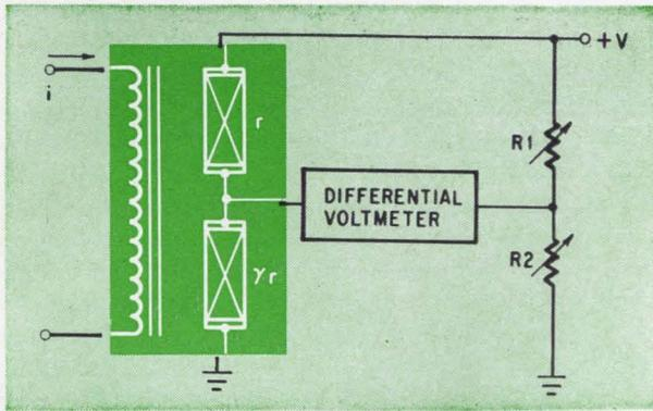
**Circuit to determine tracking error of inter-laced magneto-resistors.** The differential voltmeter is accurate to within  $\pm 0.02\%$  for inputs above 0.1 v, and  $\pm 0.02\%$  for inputs  $+2\mu$  v to 0.1 v;  $R_1$  and  $R_2$  are precision decade resistor boxes.
