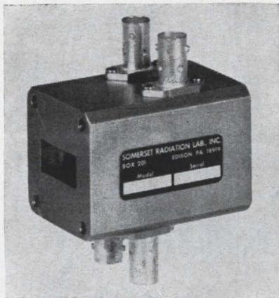
Model X710 crystal-diode, X-band digital phase shifter features a vswr of 1.04:1, a switching time of 100 nsec maximum, low insertion loss of 0.6 db, and a peak power capability of 1,000 w. In addition to being ideal for phased-antenna arrays, the unit is suitable for general laboratory, microwave-system, and classroom service as a phase shifter and phase modulator.
