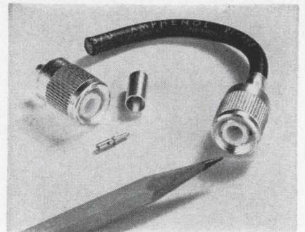
A complete line of Quick Crimp TNC coaxial connectors has been developed to meet revised military specification MIL-C-23329A. Known as MIL-Crimp TNC's, the connectors can be assembled in about 30 seconds as compared with 5 to 15 minutes for a standard solder and clamp type connector, and are far superior electrically to their older counterparts.
