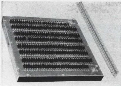
Model 30A61 delay line has a maximum delay time of  $4.0 \pm 0.01 \mu\text{sec}$ , and provides 250 equally spaced taps along its length. Impedance of the line is 150 ohms, attenuation is 3 db, and rise time is  $0.05 \mu\text{sec}$ . Connection to this  $10 \times 10 \times 1\text{-in.}$  delay network is made by two BNC connectors. Specially designed variations can be supplied to individual needs. ESC Electronics Corp., 534 Bergen Blvd., Palisades Park, N.J. [404]
