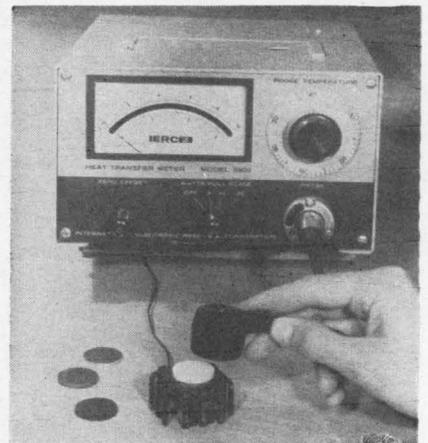
Model 5900 heat-transfer meter—designed to reduce the test time required to measure the amount of heat or energy dissipated by a
