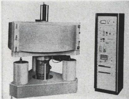
A precision dual-range centrifuge, model 444, has many design features that suit it for testing highly precise components under simulated g-forces. Range 1 is infinitely variable from 5 to 100 g's, with over-all accuracy of 0.005%. Range 2 is 10 to 600 g's, infinitely variable, and an over-all accuracy of 0.25%. Either mode will accommodate a 12-in.-cube test package, up to 50 lb dead weight, at each end of the boom. Maximum g-rating of either mode is 10,000 g-pounds.
