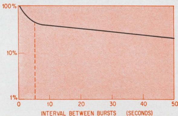
**Measured statistical distribution of intervals between bursts of errors, plotted as a function of time.** The data shows that the probability is rather high that the time between error bursts is less than five seconds.
