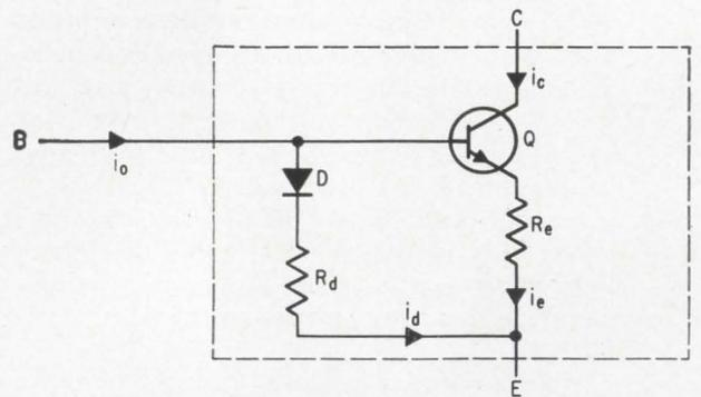
Feedback path between base and emitter improves the collector characteristics of an inexpensive germanium transistor.
