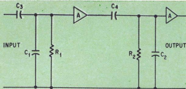
**Two-stage circuit using RC networks in the forward transmission path. Adding stages increases gain and reduces bandwidth.**
