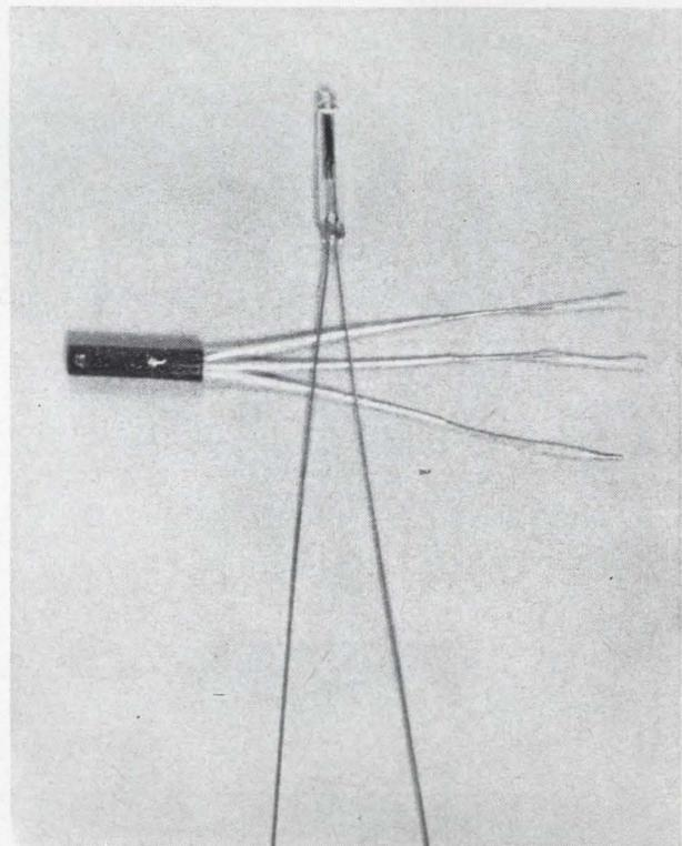
Two types of silicon photovoltaic sensors. The detector at left is a dual type. Its voltage output represents an imbalance of light on the two junctions. The other detector is a miniature solar cell.
