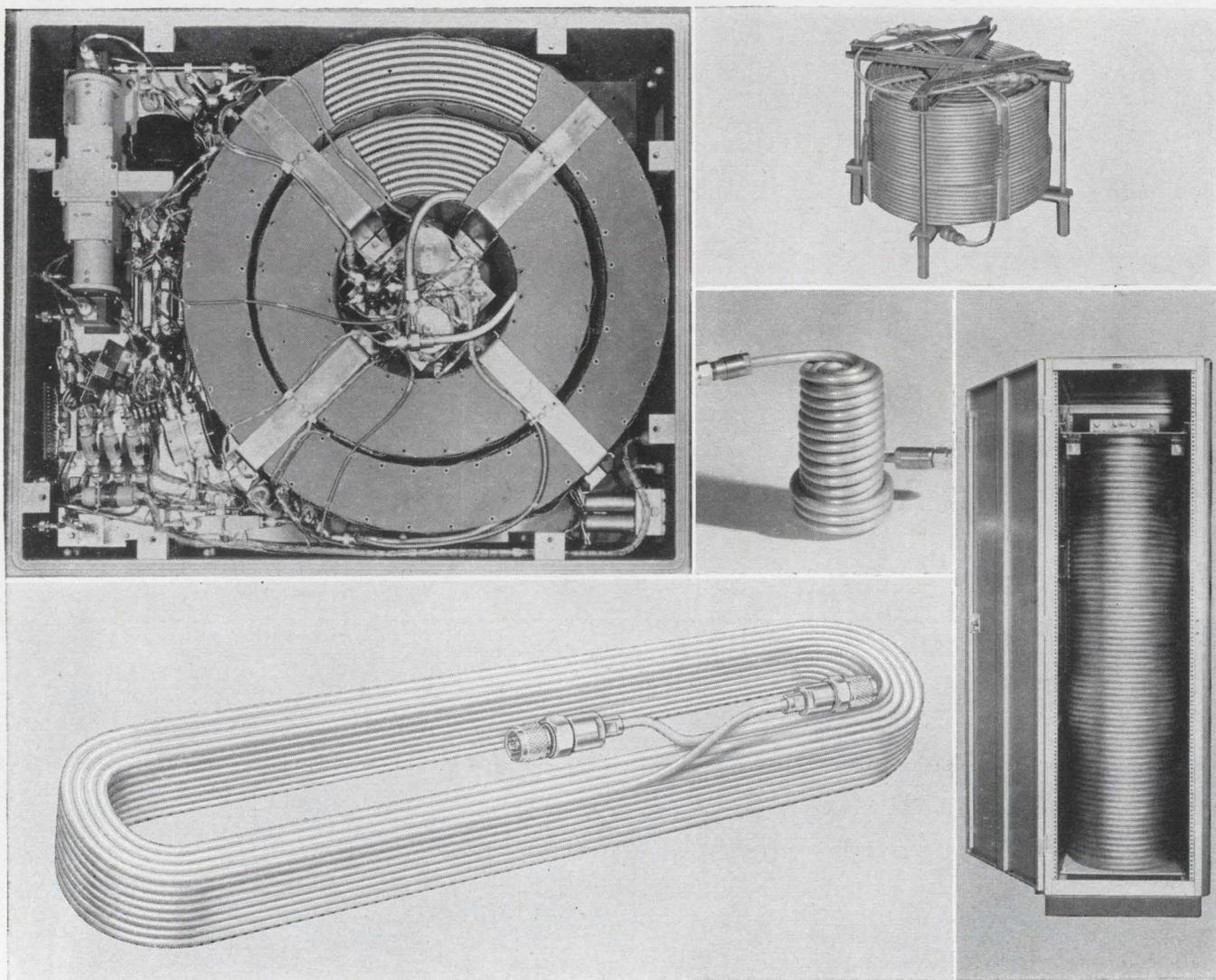
**Coaxial cable delay lines. Big. Miniature. Plain, packaged or potted. Capable of accuracies up to  $\pm .02$  nanoseconds.**
