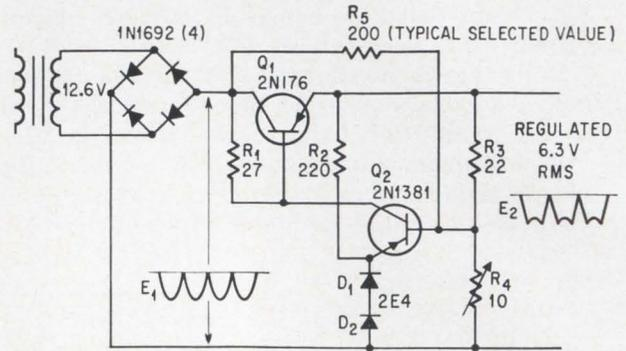
As input voltage rises, compensating resistor  $R_5$  depresses the top of the output waveform so that the effective rms output remains unchanged.
