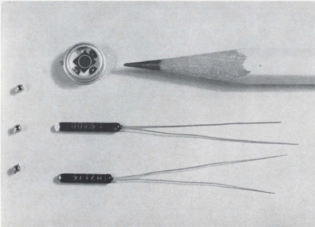
**Photoconductive pn sensors.** The detectors (all in the same package) in a column at the left are the LS600, the LS515 and the LS900. At the right (from bottom to top) are the 1N2175, the LS515, a thyristor unit and the LS900, a laser light detector.
