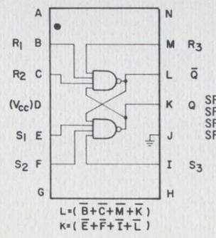
Two-Phase SR Clocked Flip-Flop
