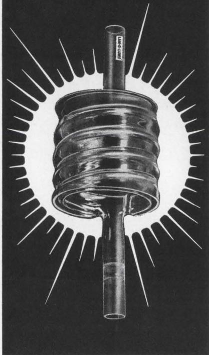
This unitized, dimensionally accurate, pure fused quartz envelope (coil), of rugged design, provides an excellent source for Xenon high intensity lighting or ultra-violet irradiation. The LAM-O-LUME can be supplied as a plain envelope or as a completed tube with electrodes and rare gas.
