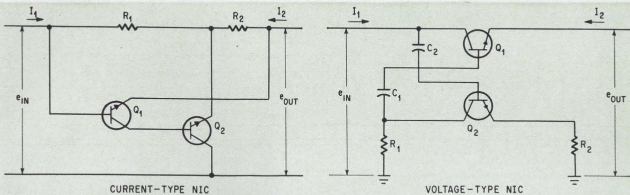
Two types of negative-impedance converter circuits. In the current-type circuit at left, input and output currents are made equal by varying the ratio  $R_1/R_2$ . The output-to-input voltage ratio of the voltage-type circuit at right is set approximately to unity by selection of  $R_1$  and  $R_2$ .
