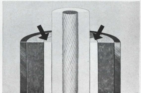
**For sealing out moisture**—Used over TFE insulation to bond with potting compounds.
