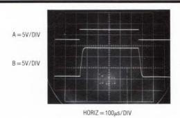
Figure 5. Expanded Scale Display of Figure 3's V<sub>pp</sub> Pulse. Controlled Risetime Eliminates Overshoots.
