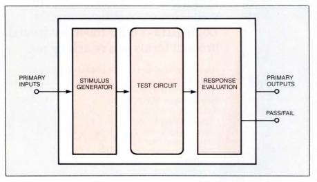
Fig 4—In a self-testing ASIC, the primary inputs seed the stimulus generator to exercise the circuit. A signature analyzer or set of comparators then evaluates the response against the expected result.
