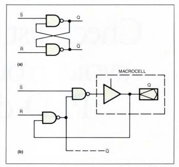
Fig 2—You can implement asynchronous set-reset latches (a) in a single macrocell by using combinatorial feedback. The cross-coupled NAND latch in **b** requires one macrocell.
