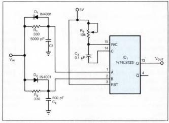
Fig 1—The RC-diode networks at the inputs of the monostable multivibrator delay one edge with respect to the other. This action produces an output pulse for every input transition—positive or negative—effectively doubling the input frequency.
