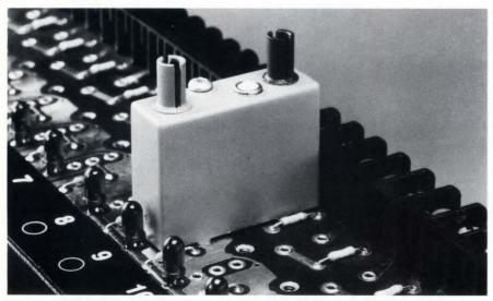
**Designed to bring the power of the PC to the manufacturing floor,** FiberPak fiber-optic sensors are available in high-speed and high-sensitivity versions that sense over 75-ft distances.
