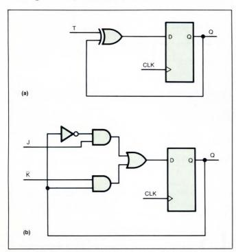
Fig 4—You can use D flip-flops to emulate both T flip-flops (a) and J-K flip-flops (b).
