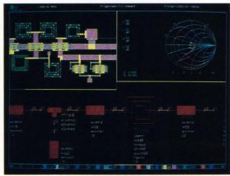
Optimized for microwave designers, the MMIC Design Workstation from EEsof comes with the Touchstone simulation package and provides schematic capture, simulation, and layout tools.
