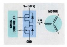
The Si9950 MOSPOWER driver is the perfect way to get more power into less space in motor control applications for disk drives, printers, copiers, plotters & battery-powered systems. It also makes an ideal MOSFET driver in high frequency power supplies.
