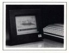
in less than 300 msec. The displays are initially being manufactured as 4-, 8-, and 14-in. diagonal versions. The 14-in. version can display a full-size A4 page. The initial displays are black and white, but color versions are under development. Samples of the 640×480-pixel display, complete with interface circuitry and a power supply, are available for £600. In high volume, the displays will compete in price with supertwist LCD technologies.
