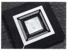
Fig 1—You can surround this standard-cell 16-bit microcontroller core of a macrocell with multiplexers to permit access to its I/O. National Semiconductor's HPCCOREA offers 64k bytes of external memory addressing, a 135-nsec cycle time (when using a 30-MHz clock), and high code efficiency because instructions are mostly single bytes.
