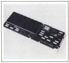
MHz, the board delivers from 8 to 10 VAX 11/780 MIPS. "Bus master" functions within the board permit the operation of as many as four coprocessors in parallel in the same enclosure. The board typically draws 4A from the 5V supply and operates from 0 to 35°C with 0 to 95% humidity. An optional NS32381 floating-point processor is also available. Board with optional floating-point unit, \$9980.
