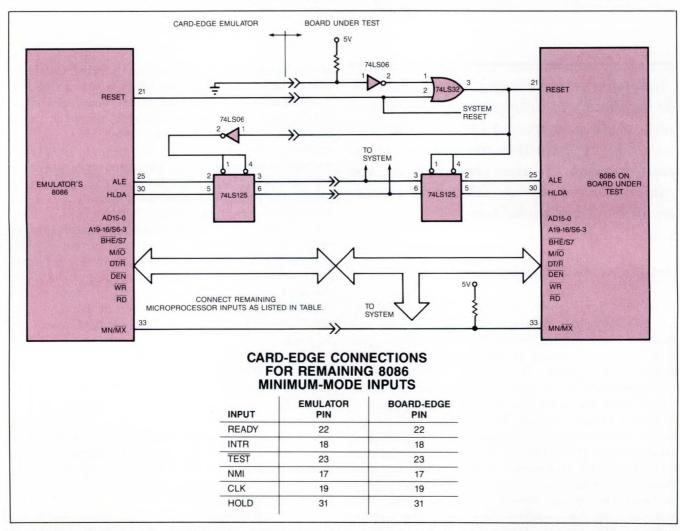
Fig 1—For an 8086 in minimum mode, you can implement card-edge emulation by placing only three ICs on the assembly that replaces the in-circuit emulator's probe.
