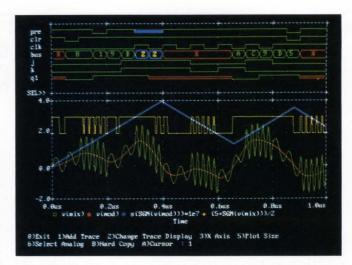
Mixed-analog/digital simulation is available on Microsim's latest release of PSpice. Nearly 50 logic primitives accurately represent TTL, CMOS, and ECL families.
