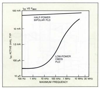
Fig 8—The power-vs-frequency characteristics of CMOS and bipolar PLDs are inherently different.
