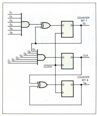
Fig 1—With this carry-look-ahead circuit, binary counters of 8 bits or more can easily fit within the 8-product-term macrocells offered by most PLDs.
