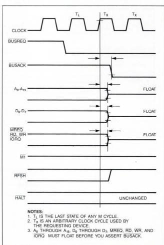
Fig 4—After a bus request, the Z80 floats the address and data buses before the second falling clock edge appears.
