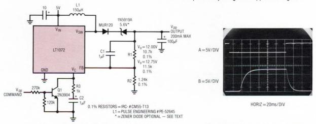
Figure 1. Basic Flash EPROM V<sub>DD</sub> Pulse Generator
