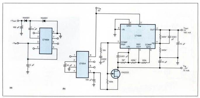
Fig 3—By adding some steering diodes to Fig 2's circuit, you can convert a negative input into a positive output (a). By modifying the circuit somewhat (b), you can develop a converter that transforms a 6V input into  $\pm 5V$  outputs.
