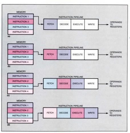
Fig 2—The SPARC pipeline holds as many as four instructions in various stages of execution. After an instruction is fetched (a), it passes through the subsequent decode (b), execute (c), and write (d) stages at the rate of one stage per clock cycle. If the processor can keep each stage filled, the average instruction time (AIT) will be one clock cycle.
