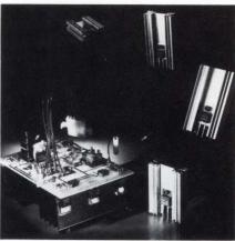
Featuring a ±5°C trip accuracy over an operating range of 40 to 120°C, the Series 6700 thermostat is housed in a TO-220 package that can be mounted directly on a heat sink.
