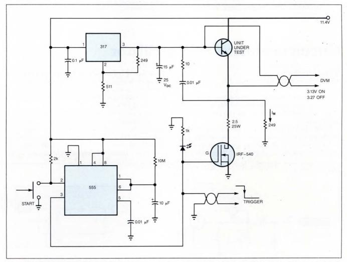
Fig 1—This 10W thermal tester applies a known high current to the transistor under test for a period of 2 minutes. You can calculate the thermal resistance of your transistor/heat-sink assembly from the change in  $V_{BE}$  you observe at high and low power levels.
