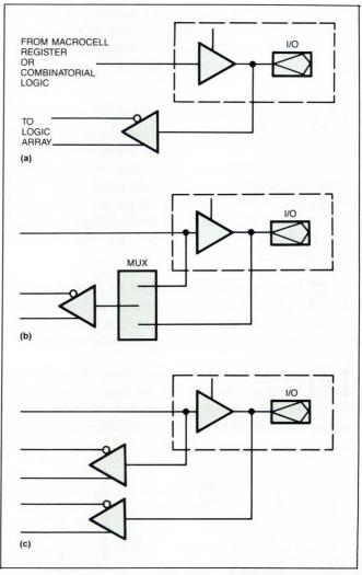
Fig 3—When using a macrocell for buried logic, beware of PLDs that have only one feedback path into the macrocell's AND-OR array (a). In these devices, buried logic functions, such as flip-flops in counters or shift registers, also consume the I/O pin. Other PLDs offer a multiplexed feedback path (b) or dual feedback (c), which allows you to bury the macrocell logic while still using the I/O pin for an unrelated input.
