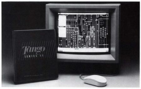
Support for 32×32-in. boards with as many as six signal layers makes the personal-computer-based Series II Tango-PCB and Tango-Route packages competitive with many workstation-based products.
