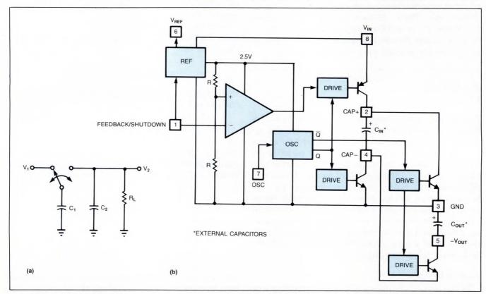
Fig 1—When the switch is in the left position, the total charge on  $C_1$  in a basic switched-capacitor building block (a) equals  $C_1V_1$ . When the switch moves to the right position,  $C_1$  discharges to voltage  $V_2$  and total charge on  $C_1$  now equals  $C_1V_2$ . Switched-capacitor converters like the LT1054 (b) have the same switching action as the basic switched-capacitor building block.
