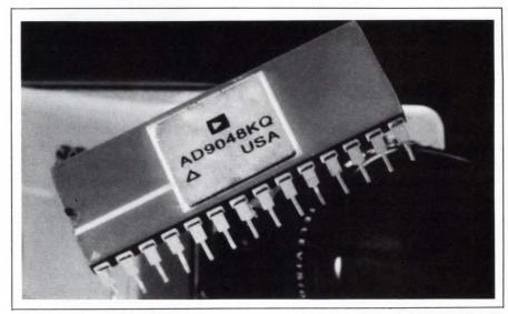
recovery time after a -3V overvoltage input is 8 nsec. The AD9048 dissipates 550 mW and operates from 5V and -5.2V supplies. Several package options, temperature grades, and accuracy grades are
