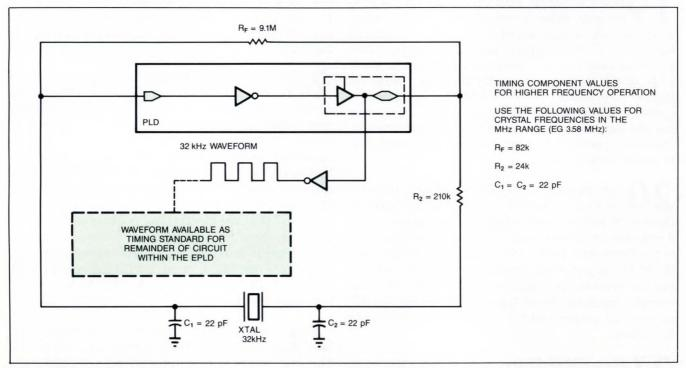
Fig 7—For timing more precise than that you can achieve using monostable multivibrators and RC oscillators built with PLDs, use a quartz crystal in conjuction with the PLD.
