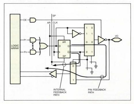
Fig 9—PLDs frequently have an external feedback path from the macrocell I/O pin as well as from the internal register's output.
