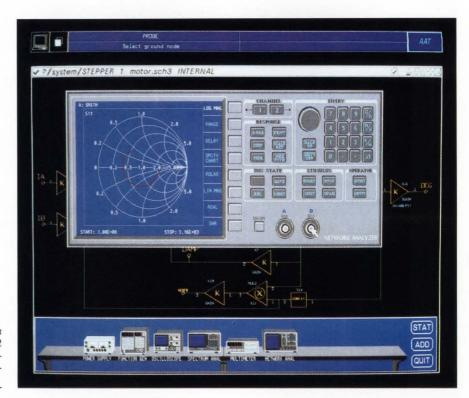
With analog-simulation packages such as this one from Intergraph, you can look at your simulation results using virtual instruments that simulate the ones you're accustomed to using on your lab bench.
