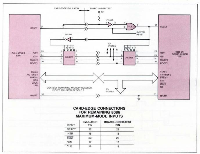
Fig 2—For an 8086 in maximum mode, implementing card-edge emulation is only slightly more complicated than it is for an 8086 in minimum mode (Fig 1).
