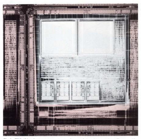
Fig 3—With this microprocessor core, you have a choice of two versions. You can either provide for scan testing of the LSI Logic 1750A core or you can multiplex out the I/O.
