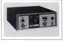
square wave whose amplitude and period you can select. The unit also provides an uncalibrated 1-kHz sine wave. You can set the square-wave amplitude from 1 mV to 100V in a 1-2-5 sequence. Voltage accuracy when driving a 1-M $\Omega$  impedance probe is  $\pm 0.5\%$ . You can set the square-wave duration from 10 nsec to 0.5 sec, also in a 1-2-5 sequence. The timing accuracy is  $\pm 0.015\%$ , and the rise time is <1 nsec. \$499.
