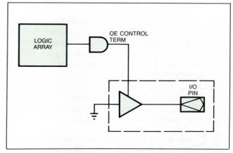
Fig 6—By driving the data input of the three-state buffer with a fixed logic 0 and using the PLD's output-enable product term for logic control, you can emulate open-drain outputs.
