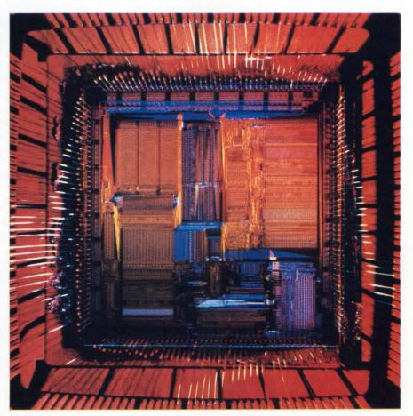
Comprising 160,000 transistors, the Motorola MC88100 RISC  $\mu P$  incorporates integer and floating-point execution units and features separate instruction and data buses to overcome memory-bandwidth limitations.
