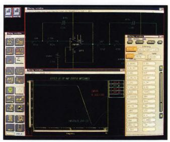
The component-modeler capability of Daisy's Analog Design System lets you modify model parameters and quickly see the effect of those changes. This example shows the effect of changing the output impedance of an amplifier. Modifying models are useful for diagnosing problems.
