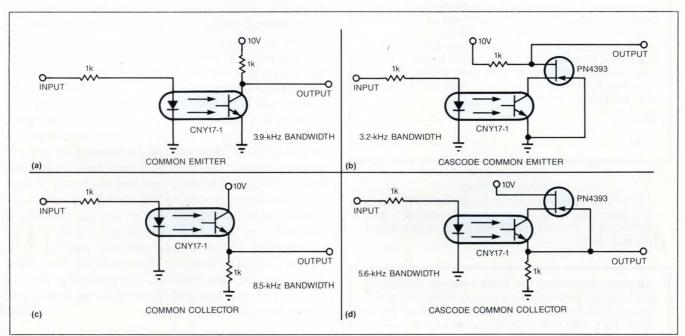
Fig 1—Adding a cascode stage to your optoisolator's feedback elements can double the optoisolator's bandwidth.
