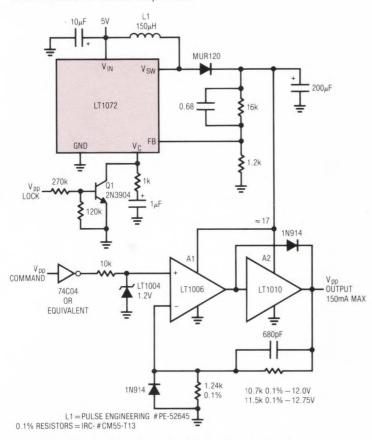
Figure 3. High Repetition Rate V<sub>pp</sub> Pulse Generator
