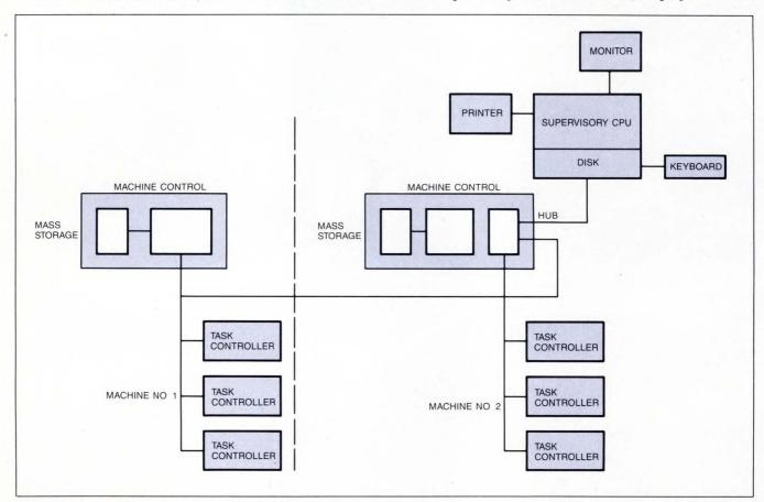
Fig 3—Local industrial topologies come in many shapes and sizes. This example shows two complex machines with various task controllers operating from a machine controller via a multidrop configuration. Each machine communicates with a supervisory unit through an active hub in a star configuration.
