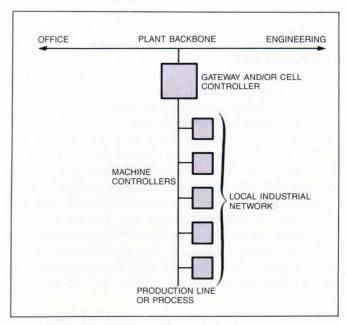
Fig 1—Typical local industrial networks connect to a large plant backbone through gateways or cell controllers.
