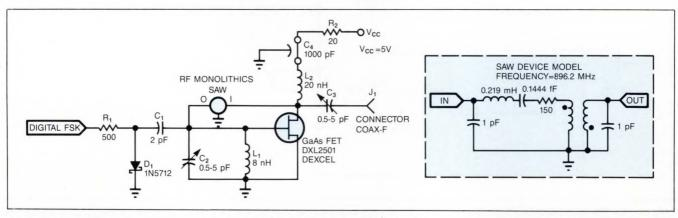
Fig 1—A simple RC-diode network transforms a SAW oscillator into a FSK oscillator.
