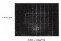
Figure 6A. An "Ideal" Flash EPROM Vpp Pulse . . .
