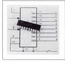
two modes of operation, Read and Write-Read, and an overflow output for cascading the devices. A Stand-Alone mode permits operation without the use of a  $\mu$ P. The device, which operates from a 5V supply, has analog and reference inputs of -0.3V to  $V_{CC}+0.3V$  and a digital input range from -0.3 to 12V. The device comes in a plastic or a ceramic DIP. From \$8.25 (100).
