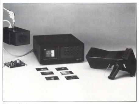
This portable thermal imaging system lets you map pc-board temperatures to identify hot spots that reduce system reliability. You can photograph images with a scope camera or transmit them via an RS-232C port to a computer.
