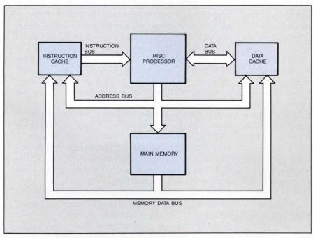
Fig 3—Because RISC processors have high memory-bandwidth requirements, many RISC-based systems employ separate data and instruction buses (a Harvard architecture) to improve the total bandwidth into the processor. Dual buses also allow you to incorporate dual cache memories in your design.
