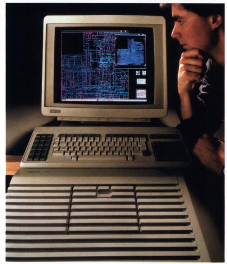
Capable of accommodating four RISC processors, the DN10000 Personal Supercomputer from Apollo Computer employs a 64-bit instruction word that's split into 32-bit integer and floating-point segments.
