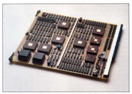
Together, the integer and the floating-point unit on the Apollo DN10000 RISC processor board can execute as many as three instructions simultaneously.
