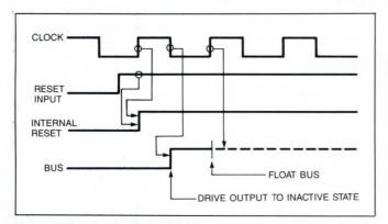
Fig 3—When the 8086's Reset input goes high, the chip waits until the next rising clock edge to set the internal reset high, and it waits until the second rising clock edge to float the bus.
