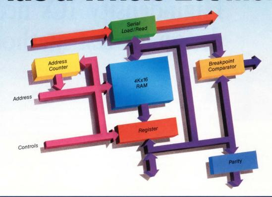
The core of the IDT 71502 is a 4K x 16 CMOS static RAM. But surrounding that core are features that will make your mouth water. Features that make the IDT 71502 work like 3 chips in 1.
