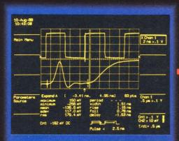
FASTGLITCH trigger mode is used to trigger on a glitch 1.51 nsec wide which occurs before the leading edge of a 500 kHz clock signal (top trace, see trigger arrow at the bottom of the graticule). Fast sampling rates, automatic pulse parameters and horizontal expansion by 250 times (lower trace) all combine to reveal the signal details.
