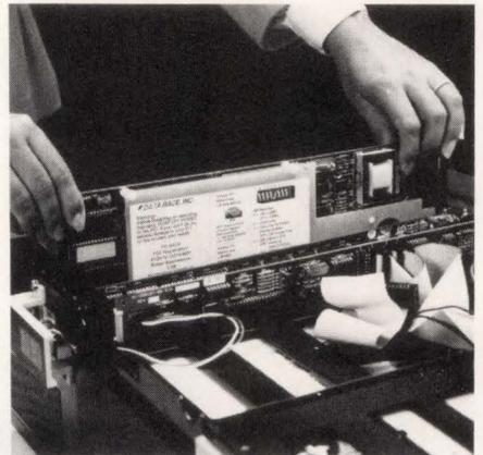
*The modular construction of the PC-Race modem card from Data Race lets you upgrade your PC's file-transfer speed from 2400 bps to 19,200 bps by plugging a daughter board into the vendor's basic, PC-compatible expansion card.*
