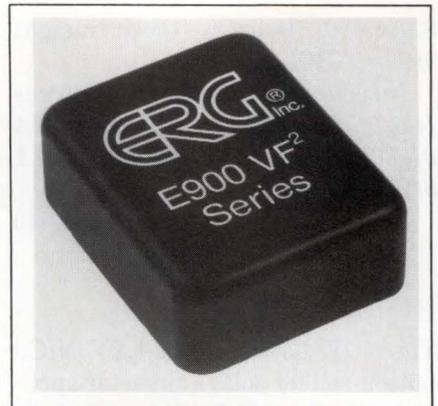
dissimilar displays requiring as much as 12W of total output power. The converters power standard displays from Noritake, Futaba, and NEC. You can order custom units for displays that require voltages not specified in the series. The units accept 5, 9, 12, 15, and 24V dc and have  $\pm 10\%$  tolerance. They operate over 0 to 70°C and provide 600V rms I/O isolation at 60 Hz for one minute. The converters weigh 122g and come in aluminum pc-board mounts
