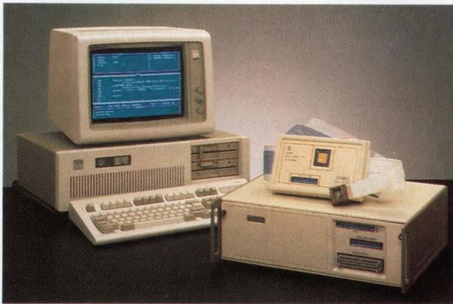
*In-circuit emulator and high-level-language debugger (Applied Microsystems and Microtec Research)*
