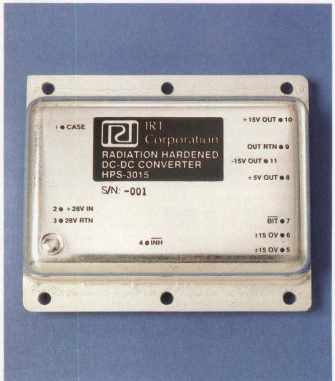
Radiation-hardened dc/dc converter (IRT Corp)
