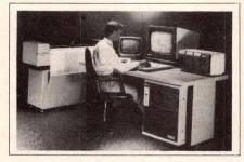
PC-BOARD CAD. Based on a Data General Model 10 computer, the MicroQuad pc-board-design workstation does more than generate board-layout artwork; it also produces parts lists, schematics, and assembly/drilling drawings. In addition, it compiles a database suitable for input into computer-aided-manufacture and test equipment such as NC-controlled drills, component-in-
