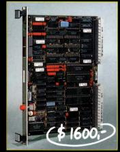
MVME050 Combo Module Controller; I/O; Memory
