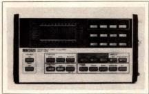
LCD LOGIC ANALYZERS. Models 1310 (10 MHz) and 1320 (20 MHz) perform logic timing, logic state, and signature analyses. These handheld, battery-powered units have 16-channel×256-word main and reference memories. Their 16-channel inputs also have one clock and one clock-qualifier line.
