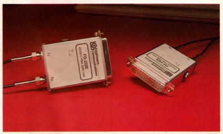
Plug-to-plug compatible with RS-232C connectors, the FO-232E from Lightwave Communications offers an inexpensive way to get complete EMI/RFI immunity when interconnecting terminals, printers, and other peripherals with computers.
