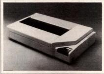
PRINTER. The OT-700 dot-matrix printer provides a 700-cps draft-quality print speed. You can also select correspondence quality printing at 350 cps. The unit offers dot-addressable graphics printing in two operating modes—50×69 dots/in. for high-speed output or 100×69 dots/in. for higher resolution copies.
