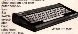
baud. Full color graphics and reverse video. 40 character  $\times$  20 lines or 20  $\times$  12 display formats. Video output for 525-line color or standard monochrome monitor. Size: 13.1"  $\times$  7"  $\times$  2". Weight: approx. 5 lbs.
