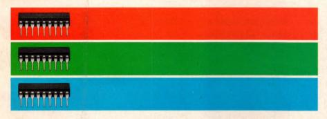
Give yourself a head start with a monolithic DAC designed specifically for raster scan systems—the TRW TDC1034 4-bit, 125 MSPS D/A converter. It directly drives CRTs to video compatible levels. Save on circuitry-no extra registering, buffering or deglitching. Save space—the 4-bit TDC1034 is an ultra-thin 18 lead DIP.
