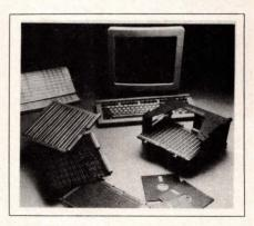
MODELING SYSTEM. See Why is a Cromemco μC-based visual interactive simulation package for computer-aided modeling. Intended for the design and control of manufacturing processes, the system lets users create plant diagrams and watch units passing through their factories on an Intecolor 8051 terminal. By varying layouts and control rules, engineers can optimize the design of factory equipment and processes. \$50,000. BLSL Inc, 83 Cambridge St, Burlington, MA 01803. Phone (617) 272-7333.
