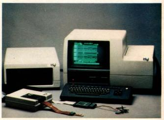
Combining in-circuit emulation with 100-MHz logic analysis, Intel's I<sup>2</sup>ICE handles as many as four of the firm's 16-bit processors at once.
