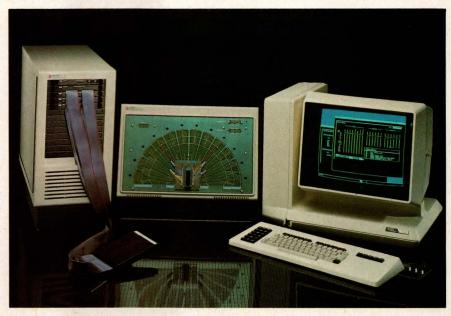
By performing tests under CAE control, the Logic Master from Integrated Measurement Systems brings prototype IC testing to the designer's workstation. Tests created on the workstation download to the Logic Master over a GPIB or RS-232C connection, while test results return to the workstation for analysis.
