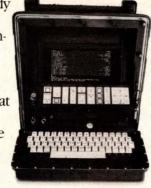
Librascope's Communications Terminal uses a fully militarized Intel bubble memory subsystem.
