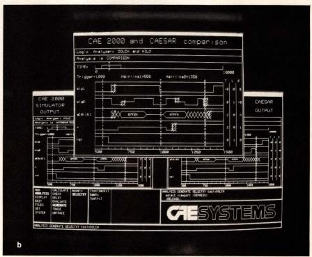
Four instrumentation plug-ins provide flexibility for the Caesar test system (a). When the plug-ins are connected to a CAE Systems workstation, test patterns and results appear in a test window (b). In addition, simulation results can be combined with the test results (middle window) for easy comparison.
