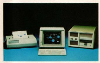
Whether running on a DEC mainframe or on the firm's 8560 development station, the integrated software for Tektronix's 8500 series supports a project from definition through debugging.
