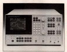
You can store as many as 32,000 recordings on disk during a single analysis session when using Model 3562A. It can extract design parameters like the open-loop or impulse response from measured data. It also serves as a design tool by accepting design parameters like pole and zero locations and generating displays like Bode plots from them.
