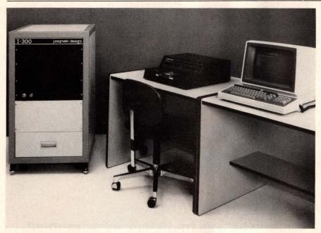
**By adding simulation software,** the Inspector 200 and 300 testers from Pragmatic Test Systems integrate CAE and testing. The Eplog software accepts net-list input, simulates the design, and generates test vectors for prototype IC test.
