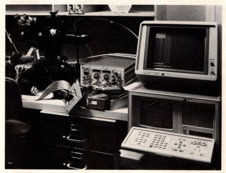
By hooking an instrumentation system to a VAX, the Tektronix DAS 9100 with the 91DVV software package links VAX Unix-based CAE tools to a variety of test configurations. The DAS (lower right) operates using local input from its own keypad or remote data from a VAX terminal.
