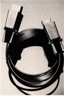
Handling analog or digital signals, Molex's fiber-optic-link components are sealed against dust and moisture. The systems transmit 40-kHz analog or 10k-baud squarewave signals over 60m.
