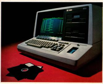
Offering a choice of high-level-language software debuggers, Hewlett-Packard's 64000 system has both software emulation and real-time hardware emulation.
