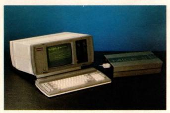
A stand-alone emulator can rival integrated development systems using an IBM PC or PC clone. Microtek's MPDS currently supports the 8048/49/50, 8085, 8086, 8088, 80186, 80188, 6809, 68000, 68010, 6502, 65SC02, 65C02, 65SC802, Z80, and NSC800. The firm plans to include the 68020 and 80286.
