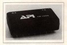
OPTICAL TRANSCEIVERS. TR1001S Series fiber-optic transceivers transmit data at rates to 100M bps NRZ. The TR1001SA version has an 8-dB system margin; the TR1001SB version has a 17-dB margin. TR1001SA. \$275: TR1001SB. \$550. American Photonics Inc. Box 289, Brookfield Center, CT 06805, Phone (203) 775-8950.
