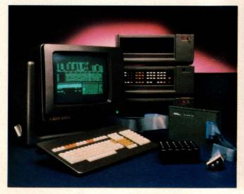
With either a Unix box or a hardwired, high-speed link to a DEC mainframe, the Kontron KDS gains access to high-level tools previously unavailable on its 8-bit controlling computer.
