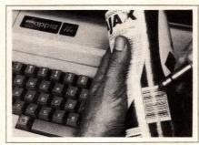
BAR-CODE READER. With the Symbtrak scanning system, your Apple IIe can read and print bar codes. The system includes a handheld scanning wand, ROM-based software, a tutorial diskette, and
