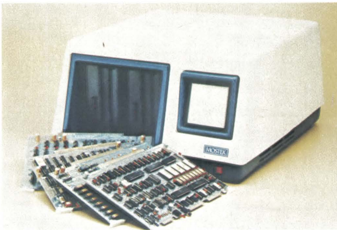
All the tools for software and hardware development and debug for Z80 and 3870 \mu P s come in Mostek's AID-80F. The enclosure, a CPU with 32k of RAM, two single-sided drives, a card case and cabling cost $5995 total.
