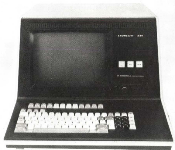
Incorporating complete hardware and software for any 6800-based development task, Motorola's Exorterm 220 costs either $8600 or $9200, depending on whether you choose dynamic or static memory.
