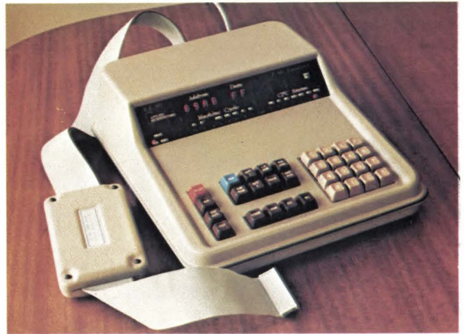
Development tools don't always come in system packages. Applied Microsystems' EZ-80 permits full emulation of Z80 \mu Ps while providing built-in diagnostics.
