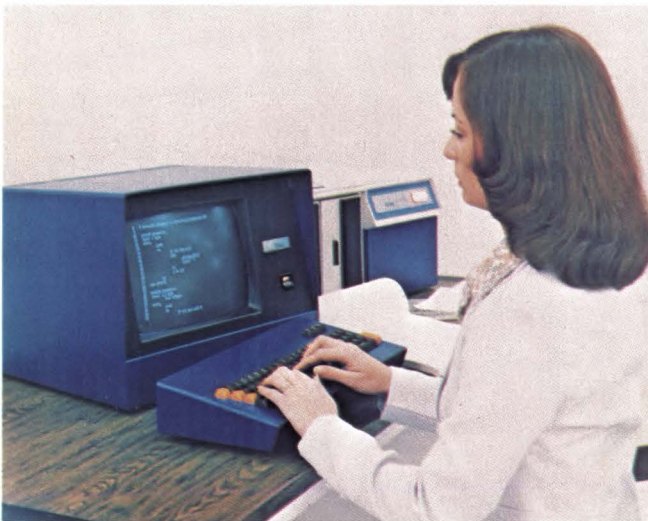
An all-in-one configuration , Zilog's ZDS-1 provides emulator, logic analyzer and ROM/RAM-simulator functions.
