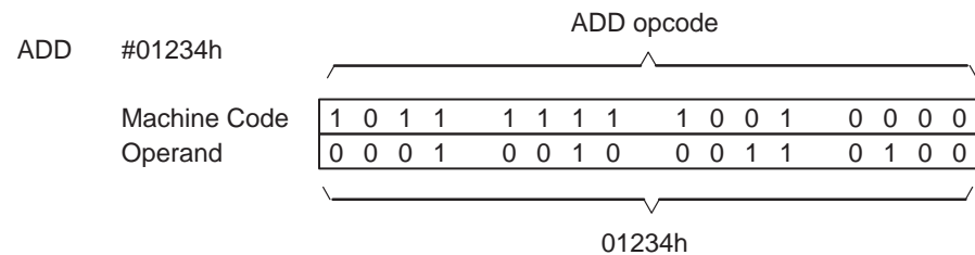
Figure 5–6. Long Immediate Addressing Mode — No Data Memory Access
