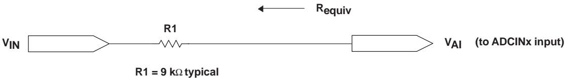
Figure 47. Typical ADC Input Pin Circuit
