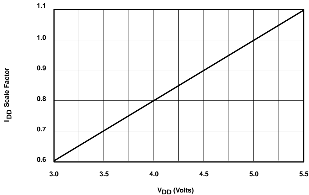
Figure 6. I_{DD} Variation With Respect to V_{DD} Supply Voltage
